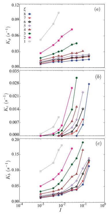
Figure 5.5 – Elongation rate  $K_g$  (a), erosion rate  $K_e$  (b), and breakage rate  $K_b$  (c) of the wet agglomerate as a function of the inertial number I for different values of the cohesion index  $\xi$ .
