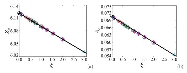
Figure 2.8 – Number density of capillary bonds (a) and bond anisotropy (b) in the quasistatic state as a function of the cohesion index  $\xi$ . The symbols and their colors correspond to different values of the control parameters as in Fig. 2 of the paper.
