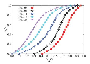
Figure 2.6 – Velocity profiles in the steady state for different values of the inertial number, with cohesion index  $\xi = 0.5$  and liquid viscosity  $\eta_f = 1$  mPa.s. The velocities are average values on in the steady flow state and they are normalized by the shear velocity applied on the top wall.
