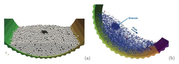
Figure 3.2 – (a) Snapshot of the granular bed showing the distribution of dry particles (in white) and wet particles (in black) both those inside the initially defined granule in the center of the bed and those randomly distributed throughout the bed; (b) Force chains during agglomeration: line thickness is proportional to normal force between neighboring particles with compressive forces in blue and tensile forces in red.
