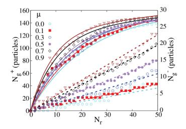
Figure 3.9 – Cumulative accretion (solid lines) and erosion (dashed lines) of wet particles for five different values of the friction coefficient  $\mu$ , size ratio  $\alpha = 5$  and  $d_{min} = 10 \ \mu m$ , as a function of the number of drum rotations. The lines are fitting forms given by equations (3.7) and (3.8).
