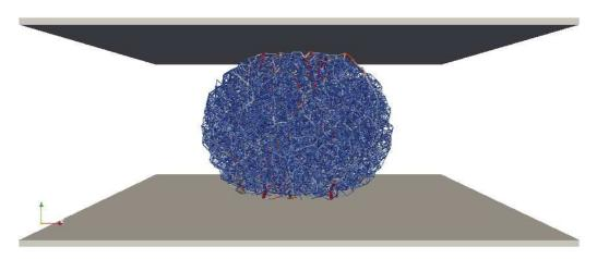
Figure 4.2 – Snapshot of a granule under diametrical compression for  $\alpha = 1$ . The lines are force chains joining the particle centers.
