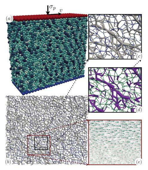
Figure 2.1 – (a) Simulated system of wet spherical particles under a constant confining stress  $\sigma_p$  and sheared by a constant horizontal velocity v of the top rough wall. The particle colors are proportional to particle diameters. (b, c) Snapshot of compressive (grey) and tensile (blue) force chains. Line thickness is proportional to normal force. (d) Snapshot of contact forces (violet) and non-contact capillary forces (green). (e) Snapshot of the particle velocity field in steady flow.
