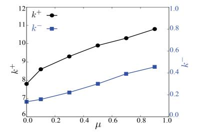
Figure 3.10 – Fitted values of erosion rate  $k^-$  and accretion rate  $k^+$  as a function of friction coefficient  $\mu$  for size ratio  $\alpha = 5$ .
