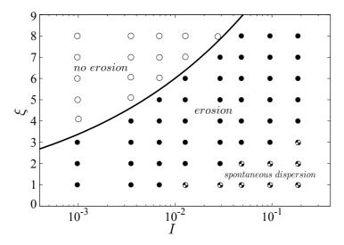
Figure 5.10 – Diagram of erosion states in the phase space  $(I, \xi)$ . The filled and empty symbols represent the states of erosion and vanishing erosion, respectively, for all the simulated values of I and  $\xi$  with a power-law frontier  $\xi = I^{1/4}/I_0$  between them. The half-filled symbols correspond to the simulations where the agglomerate breaks up spontaneously, i.e. over one time step.
