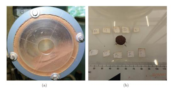
Figure 1.7 – Experimental drum demonstrating the agglomeration of single wet agglomerate in dense granular flows of dry particles (a), the geometrical granule after 50 rotations of drum (b). Experiments by R. Contreras in CRM Group, Liège.
