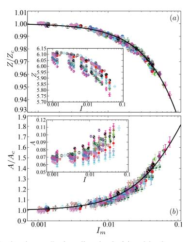
Figure 2.5 – Number density Z of capillary bonds (a) and bond anisotropy A (b) as a function of the modified inertial number  $I_m$  for different parameter values. The error-bar symbols and their colors are the as in Fig. 2.2.
