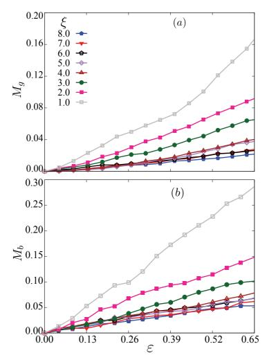
Figure 5.3 – Evolution of cumulative elongation  $M_g$  (a) and breakage  $M_b$  (b) of a wet agglomerate inside a homogeneous shear flow of dry particles as a function of cumulative shear strain  $\varepsilon$  for different values of the cohesion index  $\xi$  and for  $I \simeq 10^{-3}$ .
