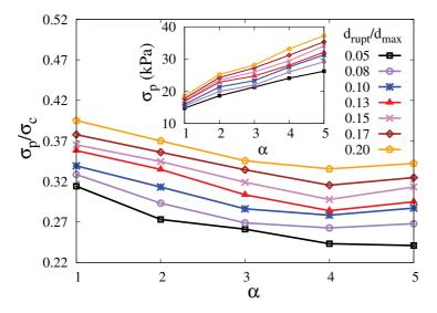
Figure 4.4 – Normalized plastic strength of the granule for several values of the debonding distance as a function of the size ratio  $\alpha$ . The inset shows the non-normalized value of the strength as a function of  $\alpha$ .
