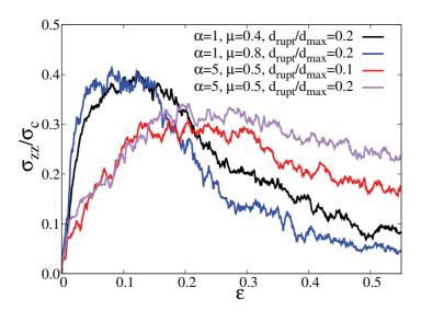
Figure 4.3 – Vertical strength  $\sigma_{zz}$  normalized by the reference stress  $\sigma_c$  for different values of friction coefficient  $\mu$ , size ratio  $\alpha$  and the debonding distance  $d_{rupt}$ , as a function of cumulative vertical strain  $\varepsilon$ .
