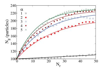
Figure 3.4 – Evolution of the granule size  $N_g$  (in number of particles) for different values of size ratio  $\alpha$  and  $d_{min} = 10 \ \mu m$ . The solid lines are exponential fits given by equation (3.6).
