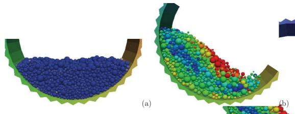
Figure 3.1 – Snapshots of the initial state (a) and stable flow (b) in the arum for a The colors show the magnitudes of particle velocities varying from red (fast particles a free surface) to blue (slowest particles in the middlezof the drum).
