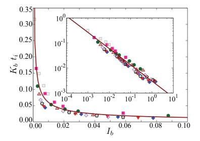
Figure 5.8 – Normalized breakage rate  $K_b t_i$  as a function of the scaling parameter  $I_b = \xi I^{\alpha_b}$  with  $\alpha_b = 1$  for all our simulations. The symbols and their colors represent the same values of cohesion index  $\xi$  as in Fig. 5.3. The solid line is a power-law fitting form (Eq. 5.11).
