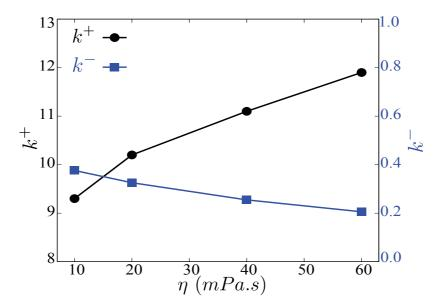
Figure 3.12 – Erosion rate  $k^-$  and accretion rate  $k^+$  as a function of liquid viscosity  $\eta$  for size ratio  $\alpha = 5$  and  $d_{min} = 10 \ \mu m$ .
