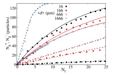
Figure 3.8 – Evolution of the cumulative number of wet particles for accretion (solid lines) and erosion (dashed lines) for four different values of the mean particle diameter  $\langle d \rangle$  and size ratio  $\alpha = 5$ , as a function of the number of drum rotations.
