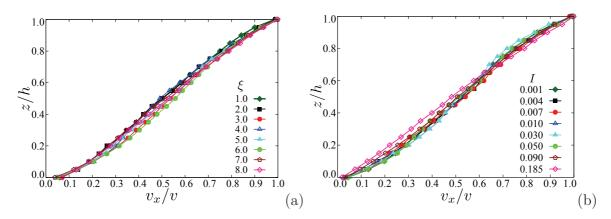
Figure 5.1 – Velocity profiles in steady shear state for different values of the cohesion index  $\xi$  (a) with  $I \simeq 10^{-3}$ , and for different values of the inertial number I with  $\xi = 5.0$  (b).
