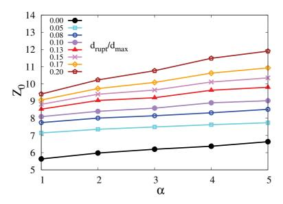
Figure 4.6 – The initial wet coordination number  $Z_0$  of the granules for different values of debonding distance as a function of the size ratio  $\alpha$ .
