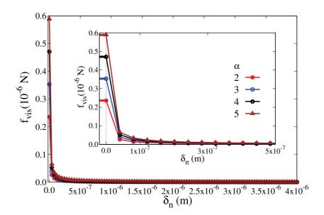
Figure 1.12 – Viscous force  $f_{vis}$  declines as a function of the gap  $\delta_n$  between two particles in the capillary contact for different values of the size ratio  $\alpha$  which is the ratio between the largest and smallest particle diameter. The viscous force exists up to the rupture distance  $d_{rupt}$ . This force is plotted for systematic parameters in Chapter 3 and keeping a fixed relative normal velocity  $\dot{\delta}_n = 5.10^{-3}$ .
