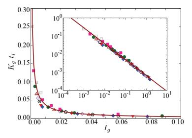
Figure 5.7 – Normalized elongation rate  $K_g t_i$  as a function of the scaling parameter  $I_g = \xi I^{\alpha_g}$  with  $\alpha_g = 1$  for all our simulations. The symbols and their colors represent the same values of cohesion index  $\xi$  as in Fig. 5.3. The solid line is a power-law fitting form (Eq. 5.10).
