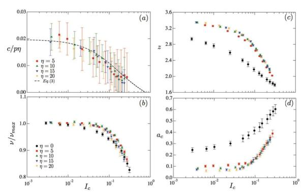
Figure 1.4 – Evolution of normalized cohesion (a), normalized packing fraction (b), coordination number (c), and the contact anisotropy (d) for different values of the cohesion index.[3]
