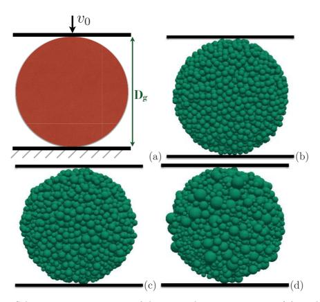
Figure 4.1 – Schematic representation of diametrical compression test (a), and snapshots of granules composed from 5000 primary spherical particles before diametrical compression for (b)  $\alpha = 1$ ; (c)  $\alpha = 2$ , and (d)  $\alpha = 5$ .
