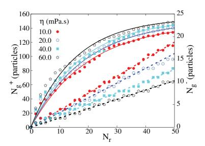
Figure 3.11 – Cumulative accretion (solid lines) and erosion (dashed lines) for four different values of the liquid viscosity  $\eta$  for size ratio  $\alpha = 5$  and  $d_{min} = 10$   $\mu$ m as a function of the number of drum rotations. The solid and dashed lines are exponential and linear fits to the data points, respectively.
