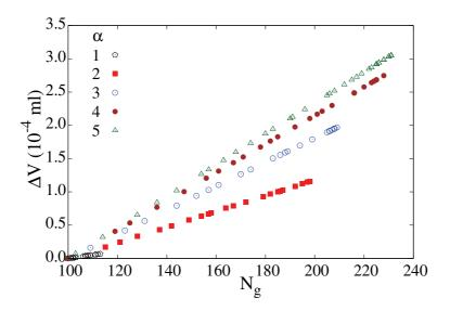
Figure 3.5 – Variation  $\Delta V$  of the volume of particles inside the granule as a function of their number  $N_q$  for different values of size ratio  $\alpha$  and  $d_{min} = 10 \ \mu m$ .
