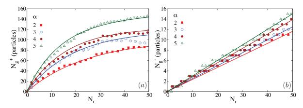
Figure 3.6 – Cumulative accretion (a) and cumulative erosion (b) of particles for different values of the size ratio  $\alpha$ . The lines are fitting forms given by equations (3.7) and (3.8), respectively.
