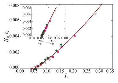
Figure 5.9 – Normalized erosion rate  $K_e t_i$  as a function of the scaling parameter  $I_e \simeq I^{\alpha_e} \xi^{\beta_e}$  with  $\alpha_e = 0.25$  and  $\beta_e = -1$  for all our simulations. The symbols and their colors represent the same values of cohesion index  $\xi$  as in Fig. 5.3. The solid line is a truncated power-law fitting form Eq. (5.13).
