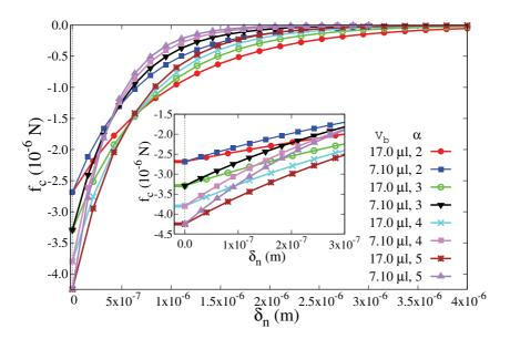
Figure 1.11 – Capillary cohesion force  $f_c$  decreases in absolute value as a function of the gap  $\delta_n$  between two particles in the capillary bridge contact for different values of the liquid volume  $V_b$  of capillary bond. The capillary force exists up to the rupture distance  $d_{rupt}$ .
