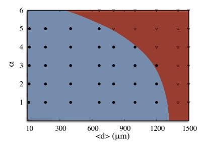
Figure 3.13 – Phase diagram of granule growth in the parametric space of  $\langle d \rangle$  vs.  $\alpha$  for  $\eta = 1$  mPa.s and  $\mu = 0.5$ . The granule grows only in the light blue region and disappears otherwise.
