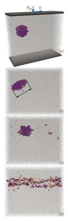
Figure 5.2 – (a) Simulated model of a wet agglomerate in a granular bed of dry particles subjected to a homogeneous shear flow; (b) elongation and erosion of the agglomerate; (c) elongation, erosion, and breakage modes; (d) spontaneous dispersion of wet particles.
