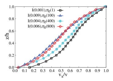
Figure 2.7 – Velocity profiles in the steady state for different values of the inertial number I and liquid viscosity  $\eta_f$  (in mPa.s) in cohesionless samples. The velocities are average values on in the steady flow state and they are normalized by the shear velocity applied on the top wall.
