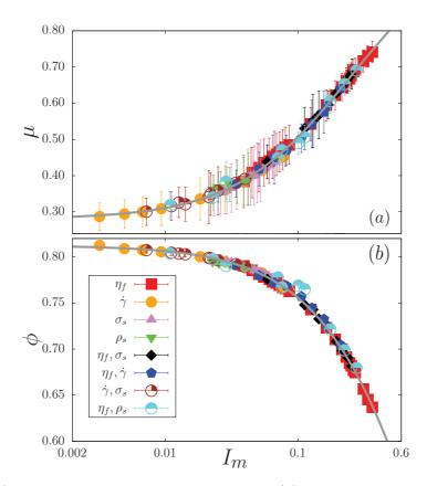
Figure 1.6 – (a) Effective friction coefficient  $\mu$  and (b) packing fraction  $\Phi$  as a function of the visco-inertial number  $I_m$  (similar to  $I_{\vartheta}$  in this thesis) for different values of liquid viscosity  $\eta_f$ , shear rate  $\dot{\gamma}$ , normal stress  $\sigma_s$ , and particle density  $\rho_s$ .[4]
