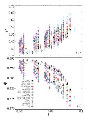
Figure 2.2 – Apparent friction coefficient  $\mu$  (a) and packing fraction  $\Phi$  (b) as a function of the inertial number I. The data are averaged over the steady state. The error bars represent the standard deviation of the data in each simulation. For each set of simulations, the symbols and their colors correspond to the parameters that are varied with their ranges, all other parameters being kept constant.
