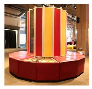
Figure 1: Supercomputer Cray-1 (photo credits from https://www.cray.com)
