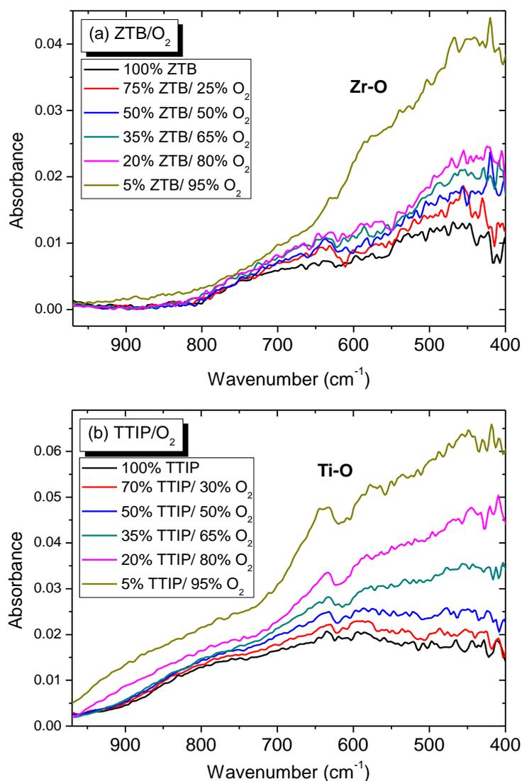
Figure III-28: FTIR spectra (950-400 cm<sup>-1</sup>) of thin films deposited at different proportion of O<sub>2</sub> gas in a) ZTB/O<sub>2</sub> and b) TTIP/O<sub>2</sub> gas mixture ( $p_{total} = 1$  mTorr,  $P_{MW} = 800$  W,  $V_{substrate} = floating$ ). Absorbance: normalised by thin film thickness.
