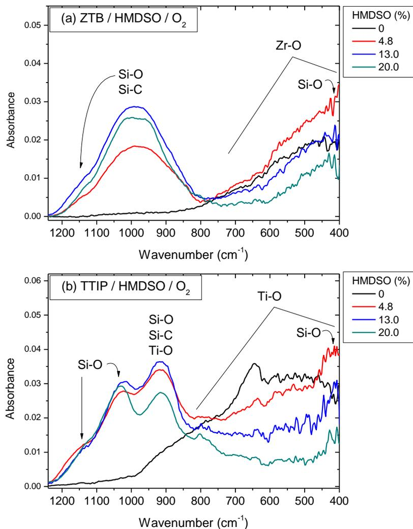
Figure V-10: Evolution of thin film FTIR spectra (1230-400 cm<sup>-1</sup>) with HMDSO addition to (a) ZTB/HMDSO/O<sub>2</sub> and (b) TTIP/HMDSO/O<sub>2</sub> plasma ( $p_{total} = 2.00\text{-}2.50$  mTorr,  $P_{MW} = 800$  W,  $V_{substrate} = \text{floating}$ ). Absorbance: normalised by thin film thickness.
