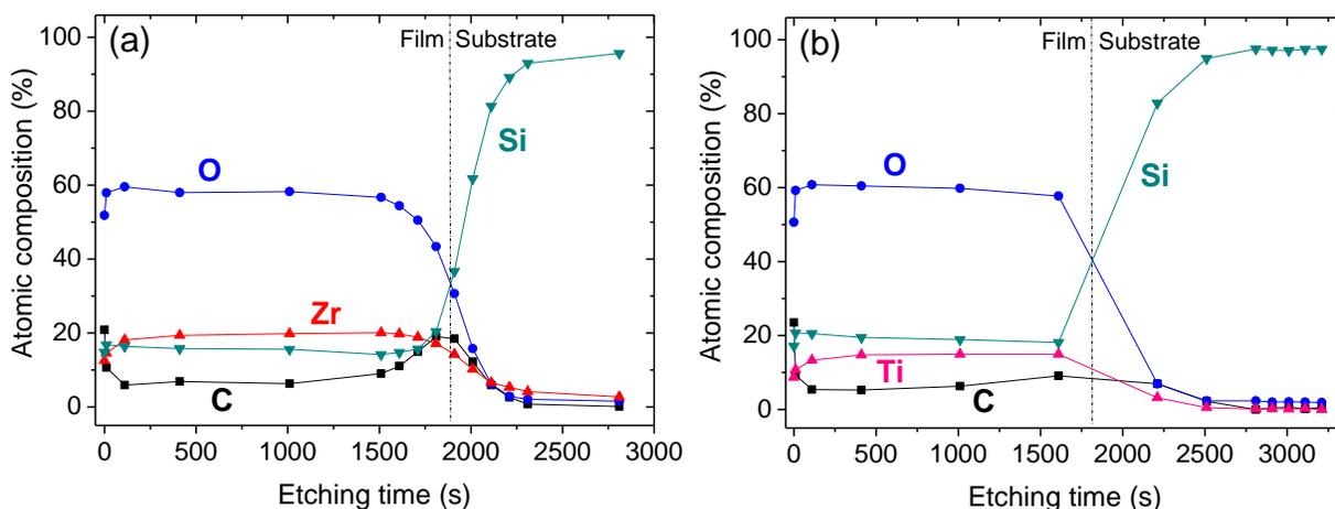
Figure V-2: XPS in-depth chemical composition profile of thin films deposited in (a) 4% ZTB/13% HMDSO/83%  $O_2$  and (b) 4% TTIP/13% HMDSO/83%  $O_2$  plasma ( $p_{total} = 2.3$  mTorr,  $P_{MW} = 800$  W,  $V_{substrate} = floating$ ).
