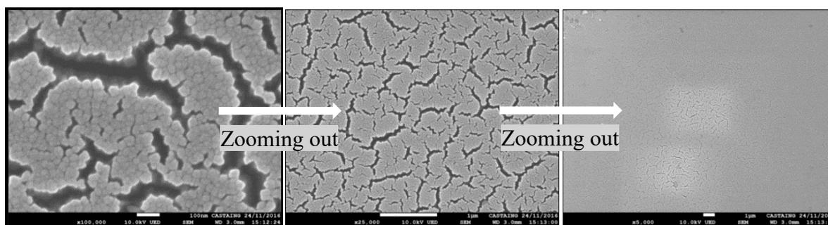
Figure IV-12: SEM images of the same location on thin film surface obtained at different levels of magnification: influence of surface charging. Thin film obtained at 6 mTorr in 5% ZTB/95% O<sub>2</sub> plasma ( $P_{MW} = 800\text{ W}$ ,  $V_{substrate} = \text{floating}$ ).
