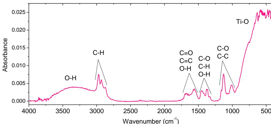
Figure III-18: FTIR spectrum of thin film deposited in 50% TTIP/50%  $O_2$  plasma ( $p_{total} = 1$  mTorr;  $P_{MW} = 800$  W,  $V_{substrate} = floating$ ).
