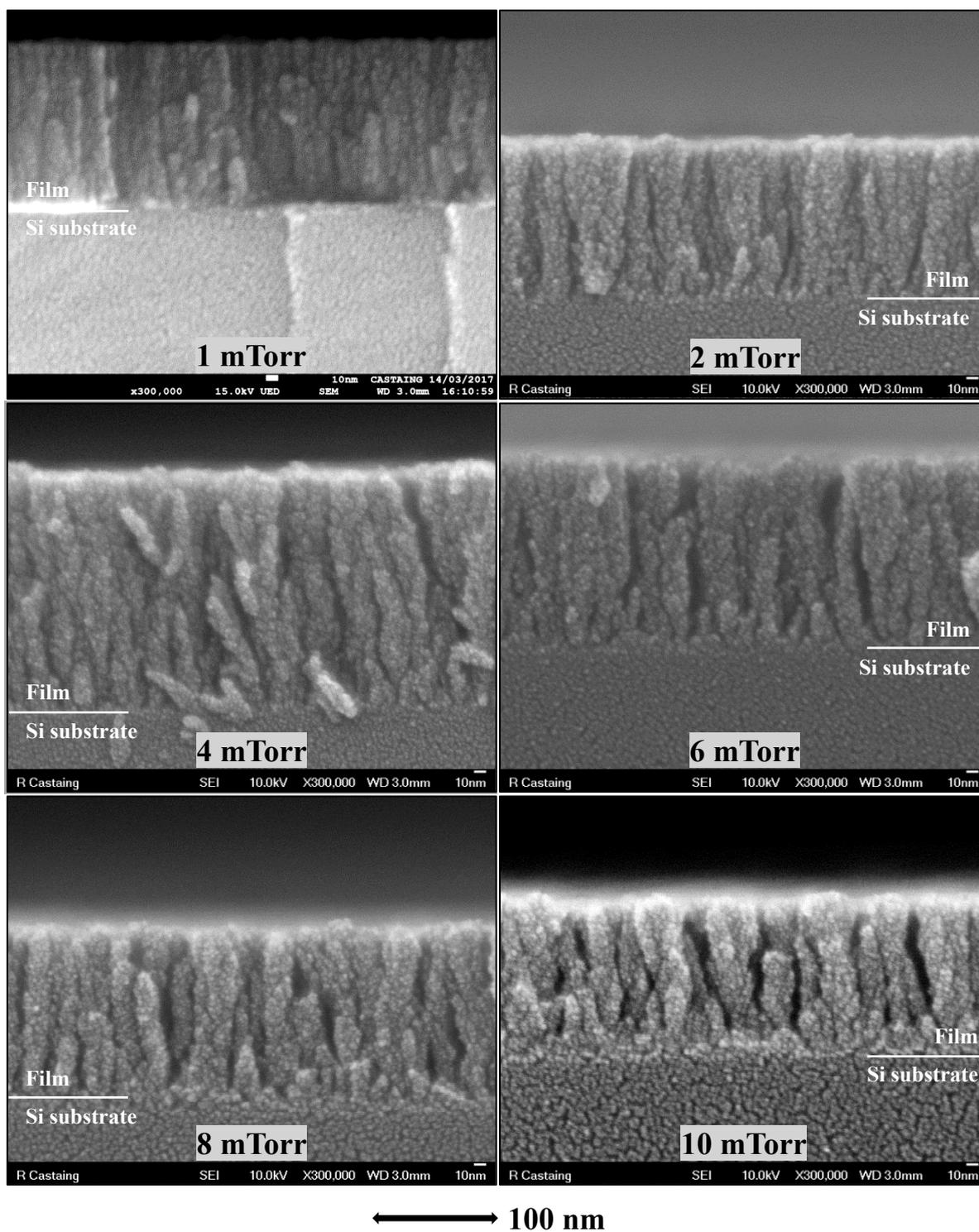
Figure IV-13: SEM cross-sectional images of thin films deposited at different total gas pressures in 5% TTIP/95% O<sub>2</sub> plasma ( $P_{MW} = 800$  W,  $V_{substrate} = floating$ ).
