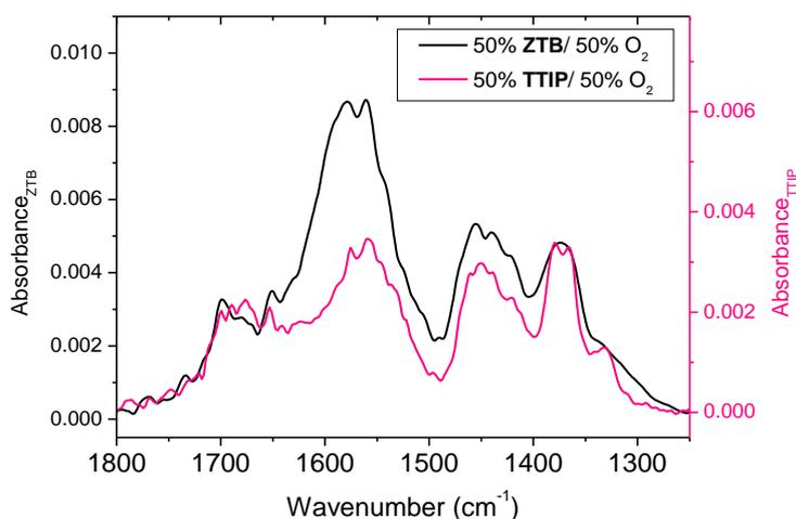
Figure III-20: Comparison of FTIR 1800-1250  $\text{cm}^{-1}$  spectral region corresponding to thin films deposited in ZTB/ $\text{O}_2$  and TTIP/ $\text{O}_2$  plasmas ( $p_{\text{total}} = 1 \text{ mTorr}$ ,  $P_{\text{MW}} = 800 \text{ W}$ ,  $V_{\text{substrate}} = \text{floating}$ ). Absorbance: normalised by thin film thickness.
