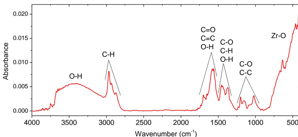
Figure III-13: FTIR spectrum of thin film deposited in 50% ZTB/50%  $\text{O}_2$  plasma ( $p_{\text{total}} = 1\text{ mTorr}$ ;  $P_{\text{MW}} = 800\text{ W}$ ,  $V_{\text{substrate}} = \text{floating}$ ).
