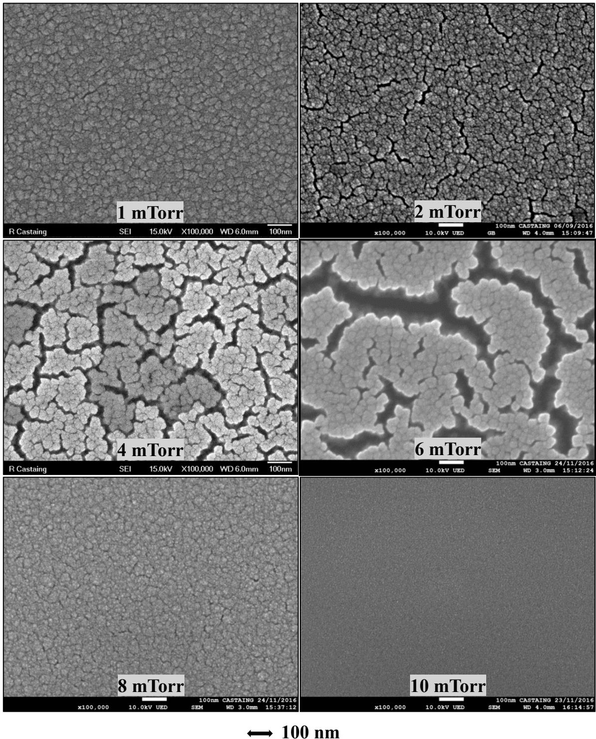
Figure IV-11: SEM surface images of thin films deposited at different total gas pressures in 5% ZTB/95% O<sub>2</sub> plasma ( $P_{MW} = 800$  W,  $V_{substrate} = floating$ ).
