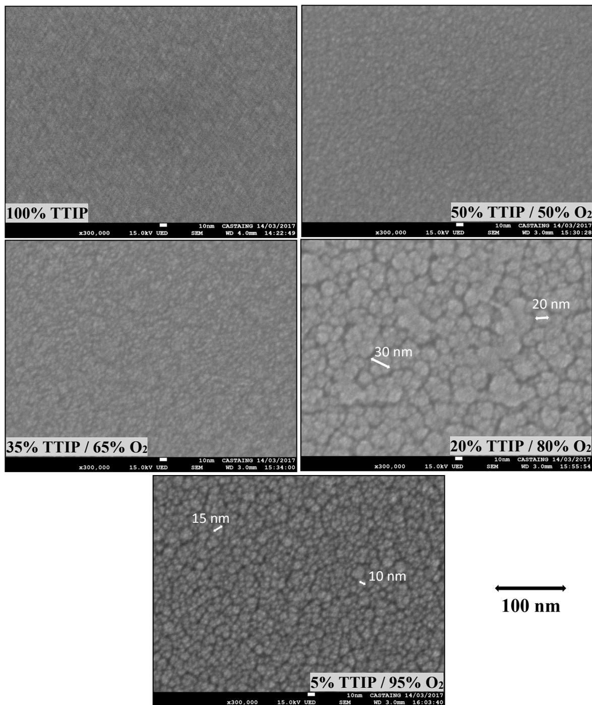
Figure III-34: SEM surface images of thin films deposited at different gas compositions in TTIP/O<sub>2</sub> plasma ( $p_{total} = 1$  mTorr,  $P_{MW} = 800$  W,  $V_{substrate} = floating$ ). Thin film thickness: 120-170 nm.
