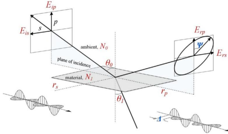
Figure II-29: Schematic representation of spectroscopic ellipsometry principle [159].
