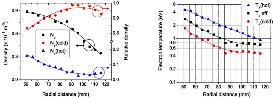
Figure II-5: Radial variations, in the mid plane, of relative density (left) and electron temperature (right) of “hot” (triangles) and “cold” (circles) electrons. Experimental conditions:  $H_2$  plasma,  $p = 0.72 \text{ Pa}$ ,  $P_{MW} = 200 \text{ W}$  applied to a single source [147].
