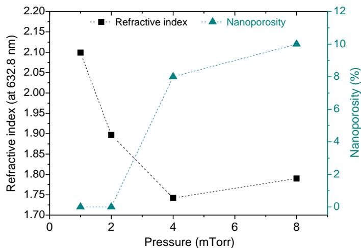
Figure IV-17: Refractive index and nanoporosity fraction of thin films deposited in TTIP/O<sub>2</sub> plasma as a function of total gas pressure (5% TTIP/95% O<sub>2</sub>,  $P_{MW} = 800$  W,  $V_{substrate} = floating$ ).
