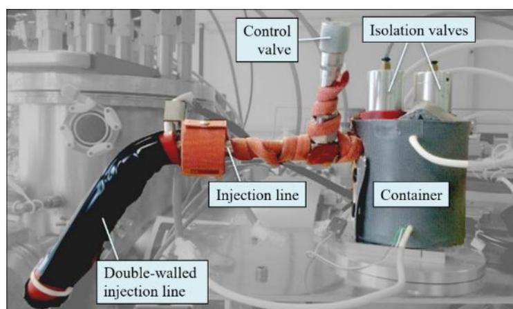
Figure II-13: Photograph of the manual precursor injection system.
