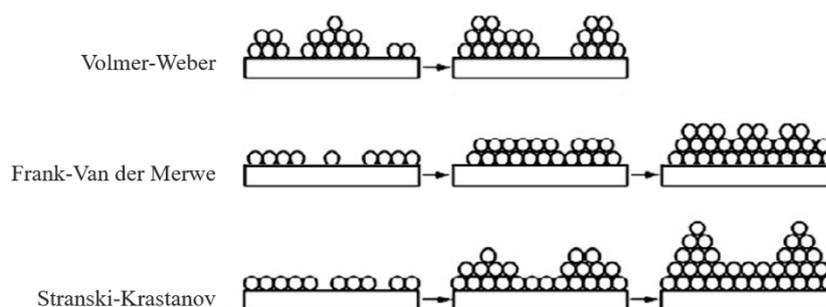
Figure I-3: Basic thin film growth modes (adapted from [14]).
