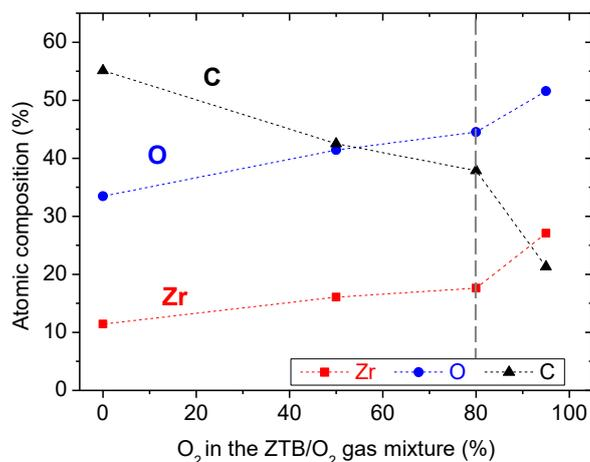
Figure III-8: Atomic composition of thin films deposited in ZTB/ $\text{O}_2$  plasma ( $p_{\text{total}} = 1$  mTorr;  $P_{\text{MW}} = 800$  W,  $V_{\text{substrate}} = \text{floating}$ ) as a function of  $\text{O}_2$  proportion in the gas mixture.
