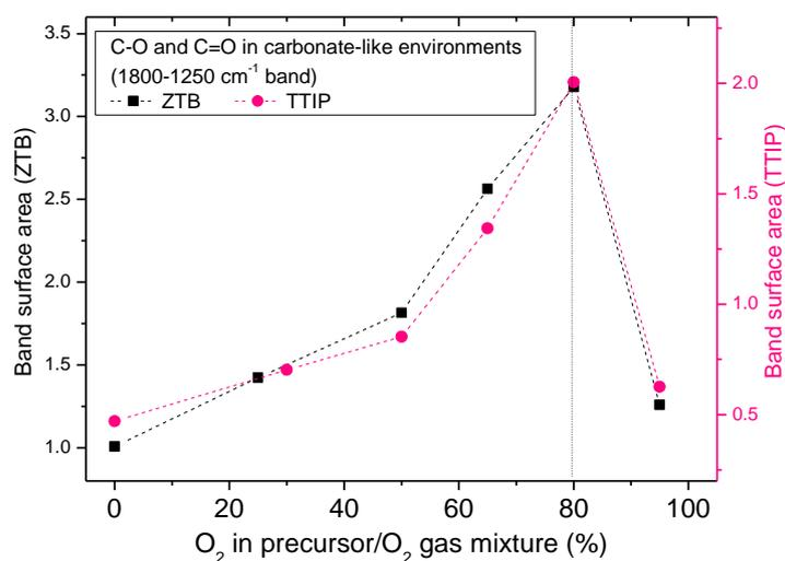
Figure III-25: Change in surface area of peaks observed in FTIR spectra of thin films deposited in ZTB/ $\text{O}_2$  and TTIP/ $\text{O}_2$  plasmas:  $1800\text{-}1250\text{ cm}^{-1}$  band (primarily C-O and C=C in carbonate-like environment).
