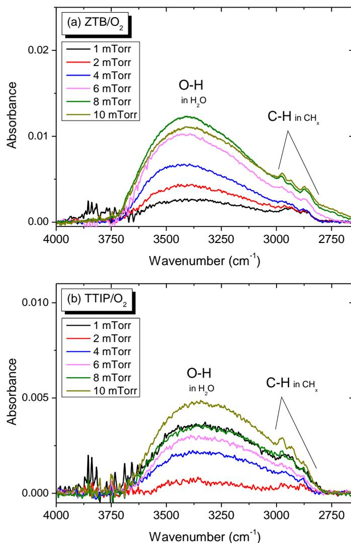
Figure IV-5: FTIR spectra (4000-2650 cm<sup>-1</sup>) of thin films deposited at different total gas pressures in a) ZTB/O<sub>2</sub> and b) TTIP/O<sub>2</sub> gas mixture (5% precursor/95% O<sub>2</sub>, P<sub>MW</sub> = 800 W, V<sub>substrate</sub> = floating). Absorbance: normalised by film thickness.
