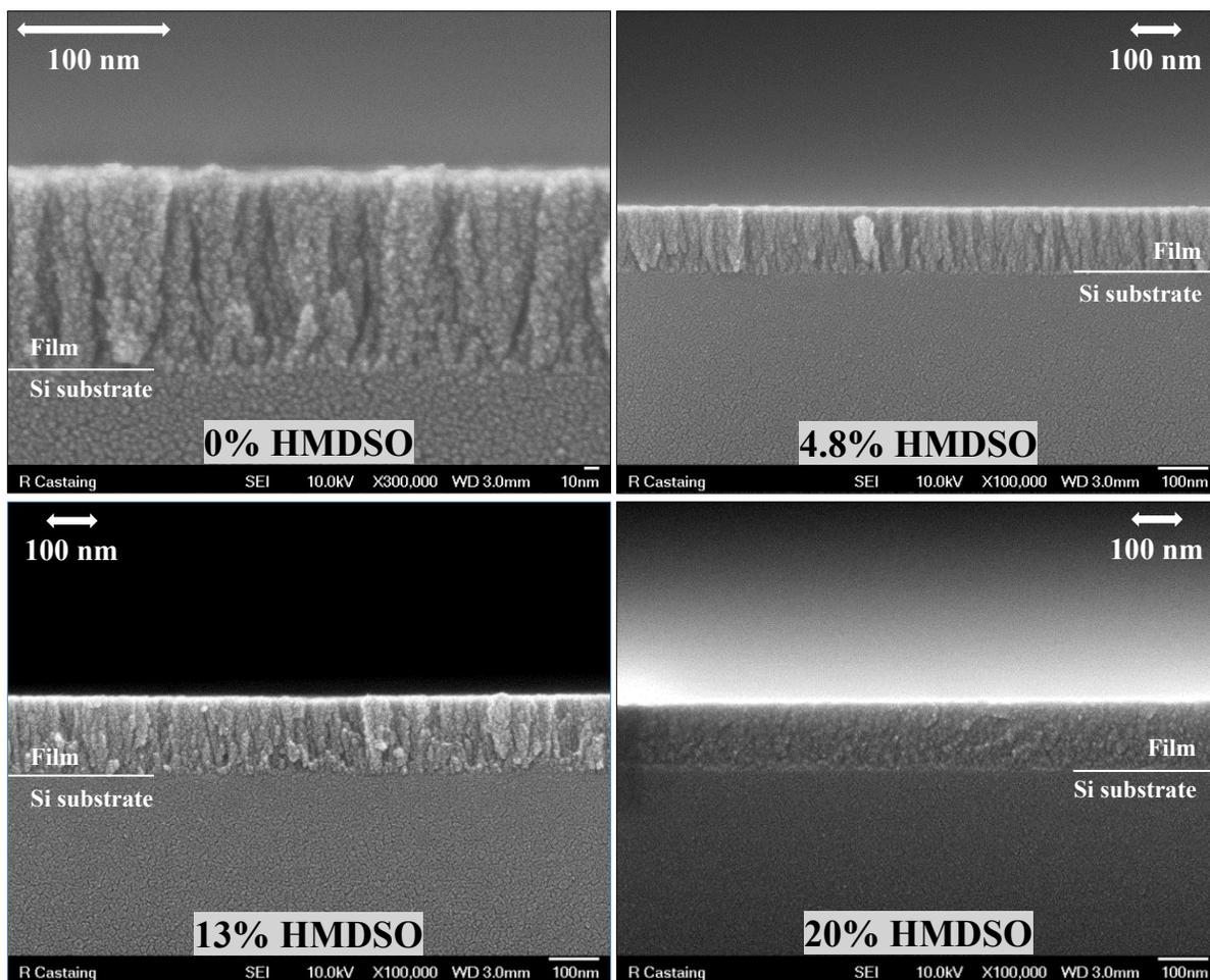
Figure V-15: SEM cross-sectional images of thin films deposited at different quantities of HMDSO in TTIP/HMDSO/O<sub>2</sub> plasma gas mixture ( $p_{total} = 2.0\text{-}2.5$  mTorr,  $P_{MW} = 800$  W,  $V_{substrate} = floating$ ).
