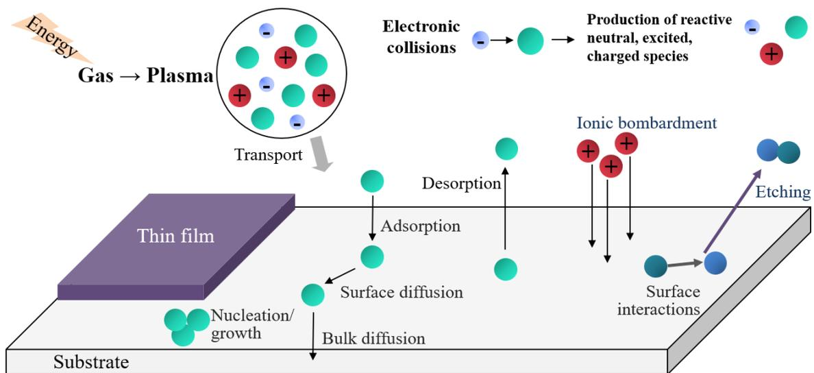
Figure I-6: Schematic presentation of plasma and surface processes in PECVD (adapted from [38]).
