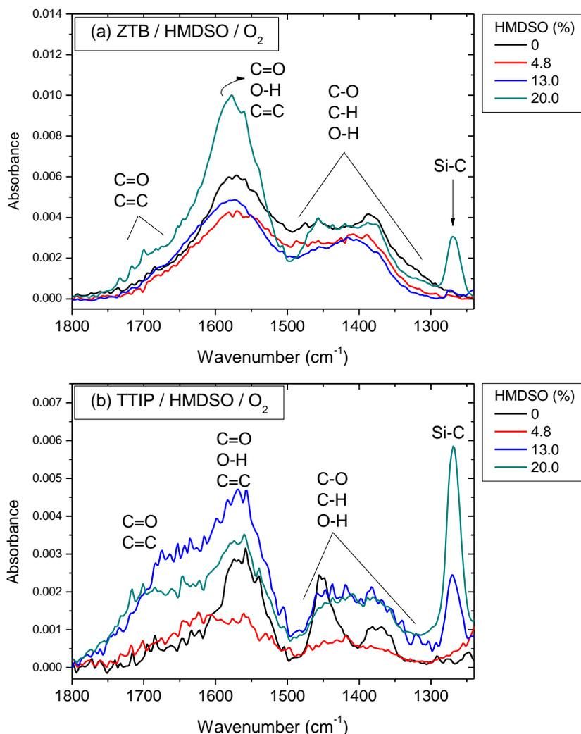
Figure V-9: Evolution of thin film FTIR spectra ( $1800\text{-}1230\text{ cm}^{-1}$ ) with HMDSO addition to (a) ZTB/HMDSO/ $\text{O}_2$  and (b) TTIP/HMDSO/ $\text{O}_2$  plasma ( $p_{\text{total}} = 2.00\text{-}2.50\text{ mTorr}$ ;  $P_{\text{MW}} = 800\text{ W}$ ,  $V_{\text{substrate}} = \text{floating}$ ). Absorbance: normalised by thin film thickness.
