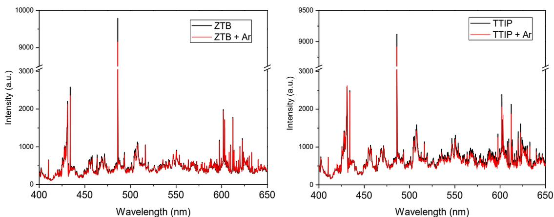
Figure III-1: Comparison of 400-650 nm region of OES spectra corresponding to precursor and precursor/Ar plasma (precursor: ZTB or TTIP,  $p_{\text{precursor}} = 1 \text{ mTorr}$ ;  $p_{\text{Ar}} = 0.05 \text{ mTorr}$ ;  $P_{\text{MW}} = 800 \text{ W}$ ).
