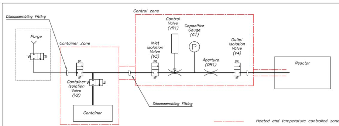
Figure II-12: Schematic representation of the LVD 200 injection system.
