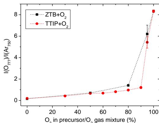
Figure III-5: Evolution of spectral line intensity ratio  $I(O)/I(Ar)$  as a function of O<sub>2</sub> fraction in precursor/O<sub>2</sub> gas mixture (precursors: ZTB or TTIP,  $p_{total} = 1$  mtorr,  $P_{MW} = 800$ W).
