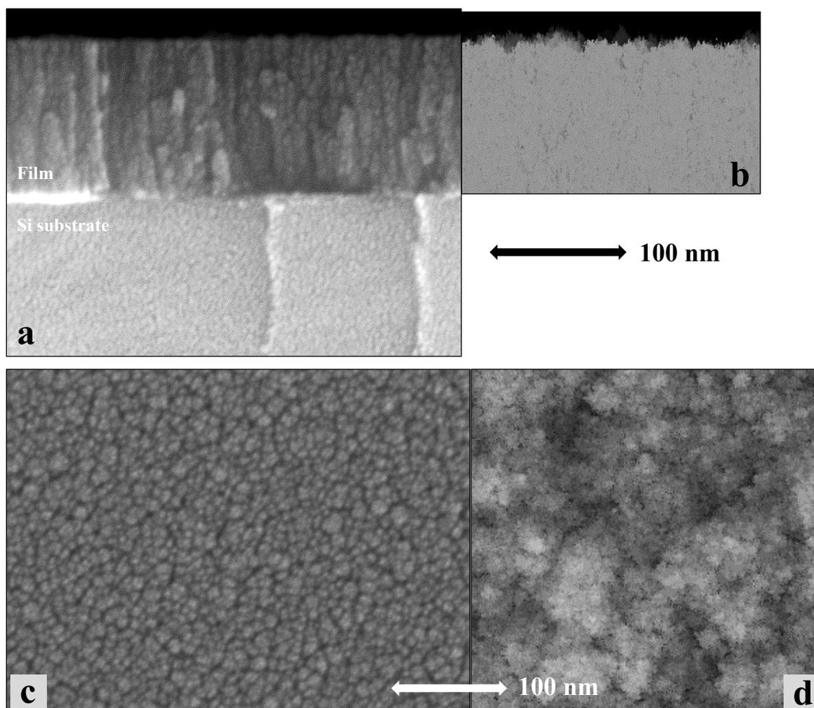
Figure III-40: Cross-sectional and surface images of thin films obtained by (a, c) PECVD from  $\text{TTIP}/\text{O}_2$ , (b, d) MC simulation of  $\text{TiO}_2$ . PECVD process parameters: 5%  $\text{TTIP}/95\% \text{O}_2$ ,  $p_{\text{total}} = 1 \text{ mTorr}$ ,  $P_{\text{MW}} = 800 \text{ W}$ ,  $V_{\text{substrate}} = \text{floating}$ . MC model parameters: perpendicular flux direction favoured, no relaxation at the surface.
