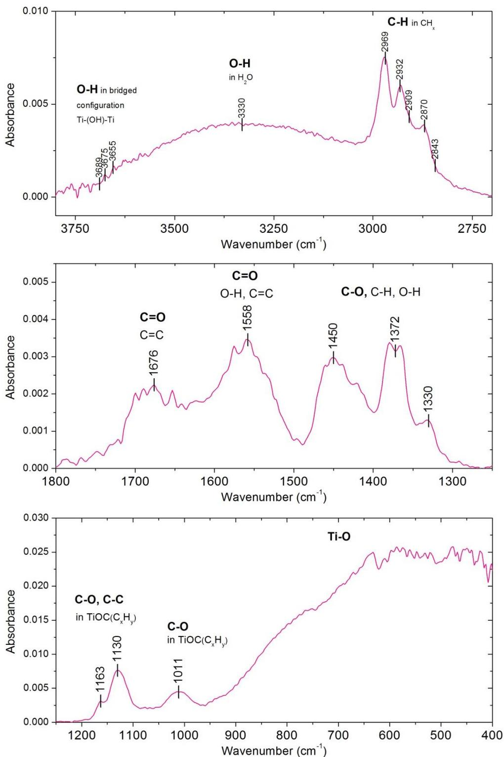
Figure A-2: FTIR spectrum of thin film deposited in 50% TTIP / 50% O<sub>2</sub> plasma ( $p_{total} = 1$  mTorr,  $P_{MW} = 800$  W,  $V_{substrate} = floating$ ).
