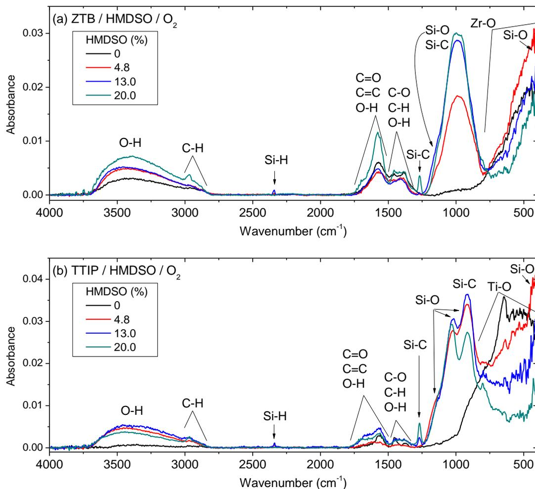
Figure V-7: Evolution of thin film FTIR spectra ( $4000\text{-}400\text{ cm}^{-1}$ ) with HMDSO addition to (a) ZTB/HMDSO/ $\text{O}_2$  and (b) TTIP/HMDSO/ $\text{O}_2$  plasma ( $p_{\text{total}} = 2.00\text{-}2.50\text{ mTorr}$ ,  $P_{\text{MW}} = 800\text{ W}$ ,  $V_{\text{substrate}} = \text{floating}$ ). Absorbance: normalised by thin film thickness.
