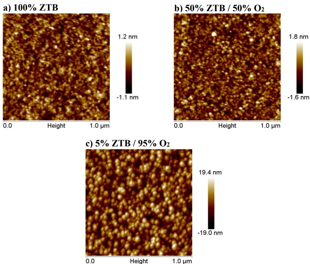
Figure III-29: AFM surface images of thin films grown in ZTB/O<sub>2</sub> plasma ( $p_{total} = 1$  mTorr,  $P_{MW} = 800$  W,  $V_{substrate} = floating$ ): (a) 100% ZTB, (b) 50% ZTB/50% O<sub>2</sub>, (c) 5% ZTB/95% O<sub>2</sub>.
