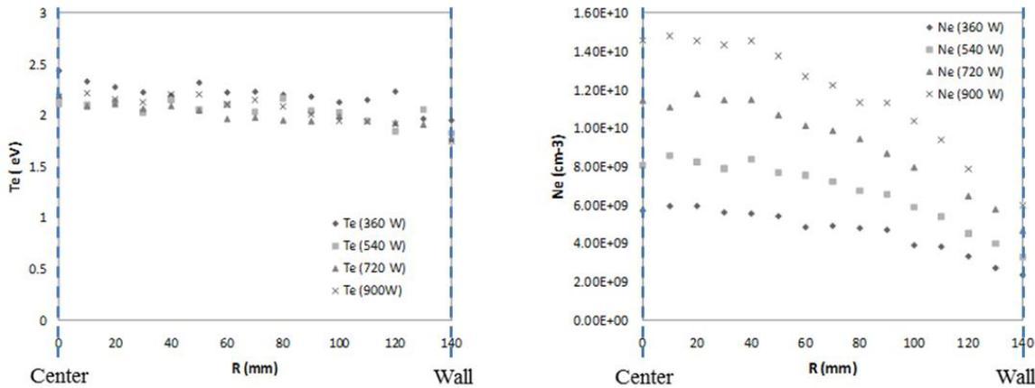
Figure II-6: Evolution of plasma parameters  $T_e$  and  $N_e$  as a function of distance from the centre of the deposition reactor Pixcell for different power values (12 elementary sources; Ar gas;  $p_{Ar}=3 \text{ mTorr}$ ).
