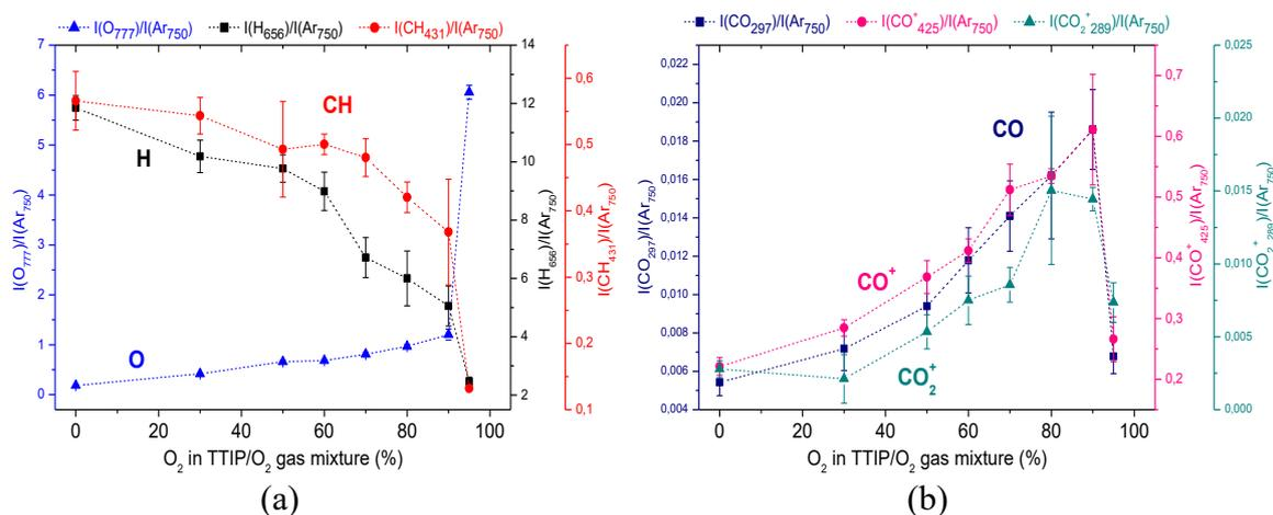
Figure III-4: Evolution of spectral line intensity ratios as a function of O<sub>2</sub> gas percentage of TTIP/O<sub>2</sub> gas mixture ( $p_{TTIP+O_2} = 1$  mTorr;  $p_{Ar\ gas} = 0.05$  mTorr;  $P_{MW} = 800$  W): (a)  $I(O)/I(Ar)$ ,  $I(H)/I(Ar)$ ,  $I(CH)/I(Ar)$ , (b)  $I(CO)/I(Ar)$ ,  $I(CO^+)/I(Ar)$ ,  $I(CO_2^+)/I(Ar)$ .
