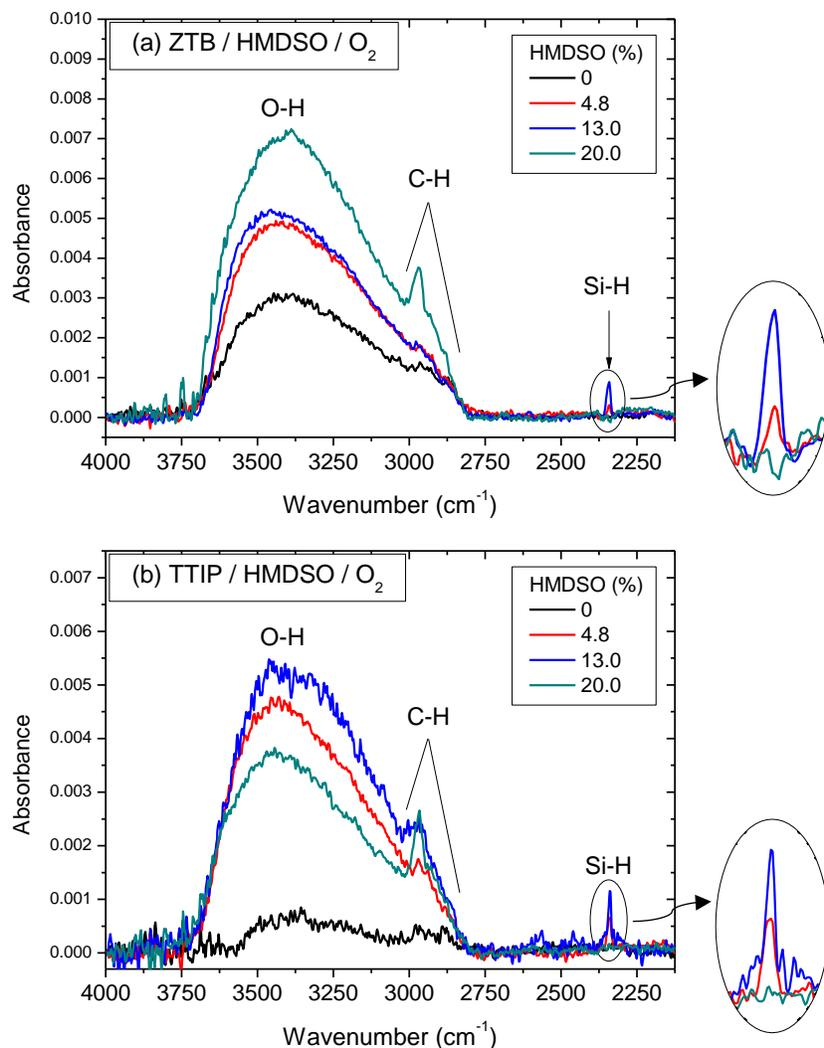
Figure V-8: Evolution of thin film FTIR spectra (4000-1800  $\text{cm}^{-1}$ ) with HMDSO addition to (a) ZTB/HMDSO/O<sub>2</sub> and (b) TTIP/HMDSO/O<sub>2</sub> plasma ( $p_{\text{total}} = 2.00\text{-}2.50$  mTorr;  $P_{\text{MW}} = 800$  W,  $V_{\text{substrate}} = \text{floating}$ ). Absorbance: normalised by thin film thickness.
