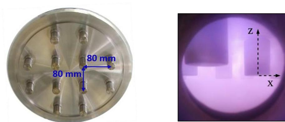
Figure II-3: Photographs of: 12 multi-dipolar magnets positioned at the top of the plasma chamber (left); magnets in argon plasma ( $p_{Ar}=1$  mTorr;  $P_{MW}=800$  W) (right).
