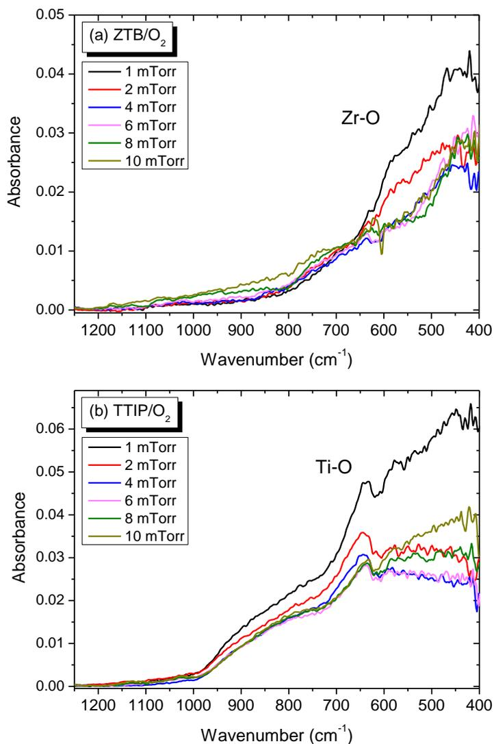
Figure IV-8: FTIR spectra (1250-400  $\text{cm}^{-1}$ ) of films deposited at different total gas pressures in a) ZTB/ $\text{O}_2$  and b) TTIP/ $\text{O}_2$  plasma (5% precursor/95%  $\text{O}_2$ ,  $P_{MW} = 800 \text{ W}$ ,  $V_{\text{substrate}} = \text{floating}$ ).
