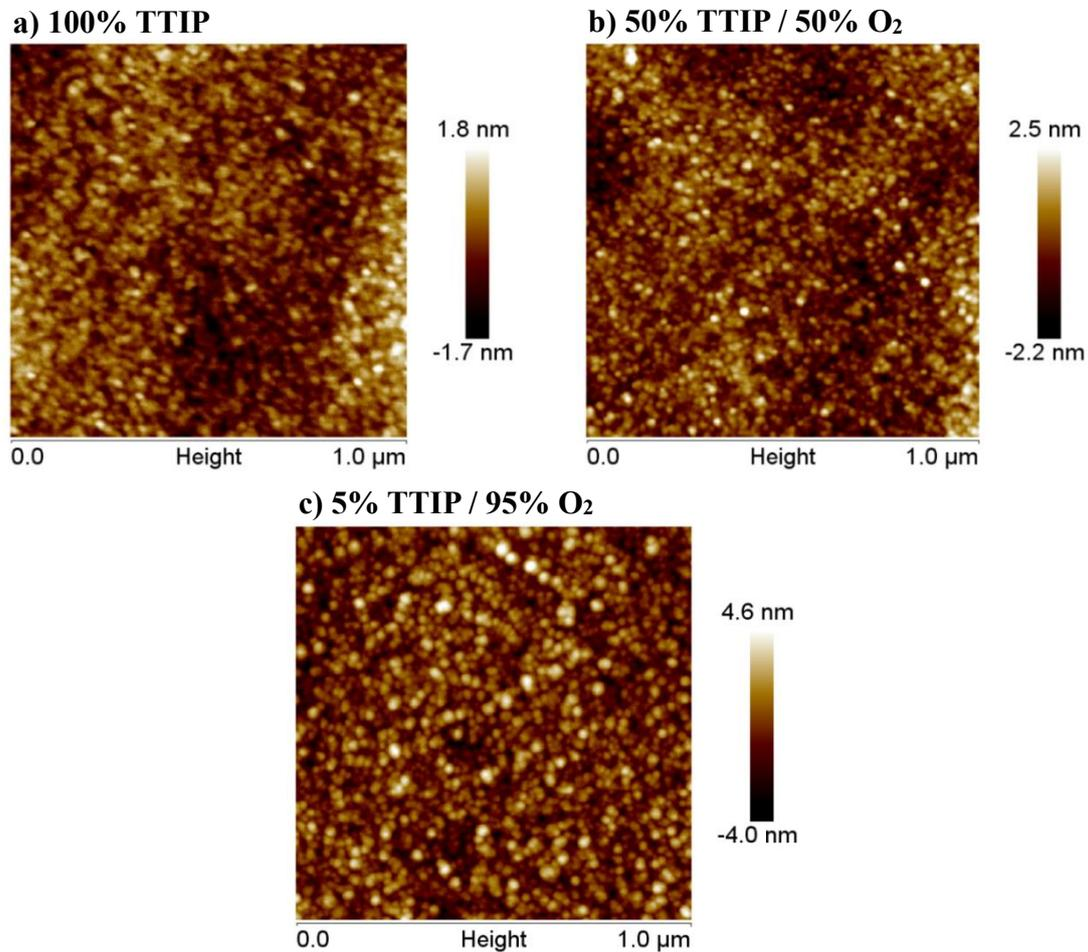
Figure III-32: AFM surface images of thin films grown in TTIP/O<sub>2</sub> plasma ( $p_{total} = 1$  mTorr,  $P_{MW} = 800$  W,  $V_{substrate} = floating$ ): (a) 100% TTIP, (b) 50% TTIP/50% O<sub>2</sub>, (c) 5% TTIP/95% O<sub>2</sub>.
