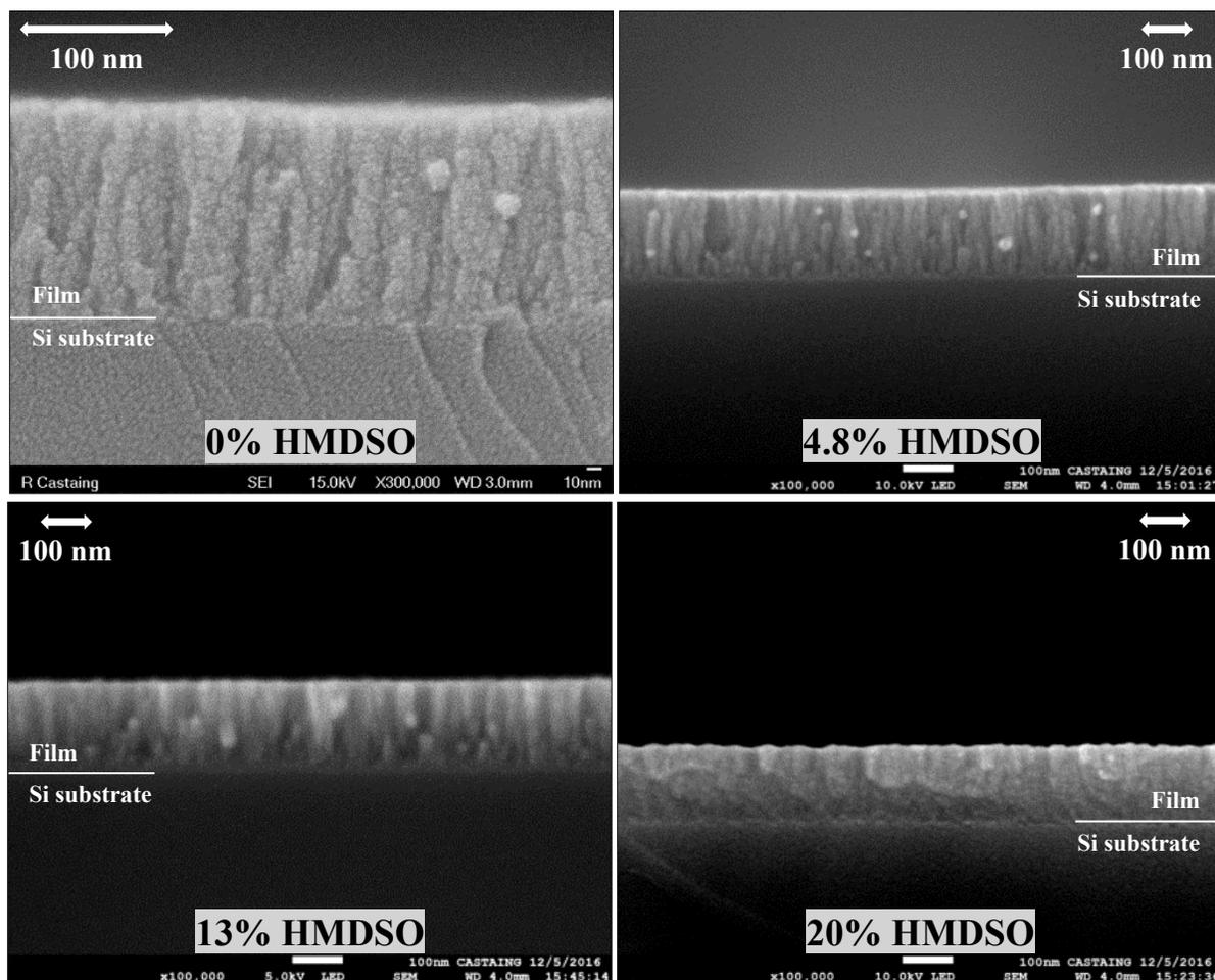
Figure V-13: SEM cross-sectional images of thin films deposited at different quantities of HMDSO in ZTB/HMDSO/O<sub>2</sub> plasma gas mixture ( $p_{total} = 2.0\text{-}2.5\text{ mTorr}$ ;  $P_{MW} = 800\text{ W}$ ;  $V_{substrate} = \text{floating}$ ).
