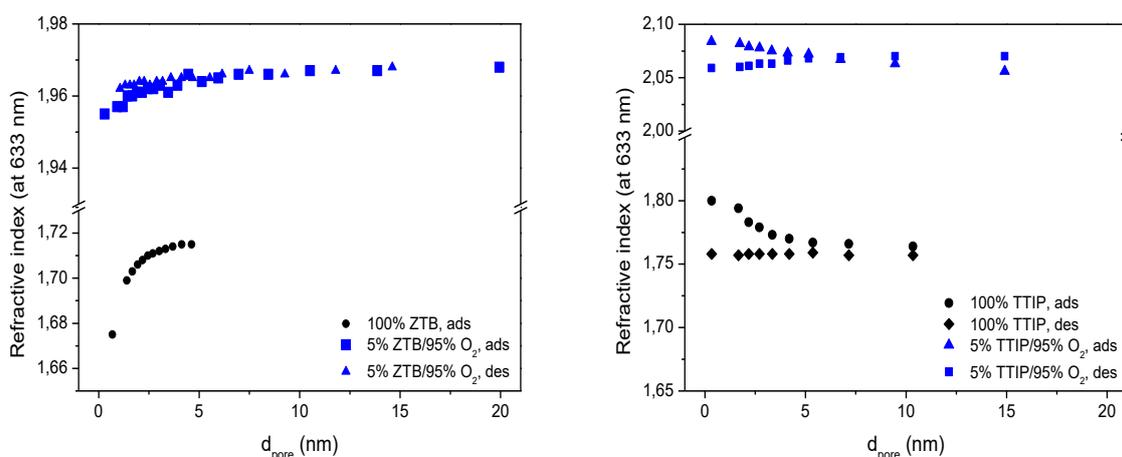
Figure III-42: Refractive index as a function of pore diameter measured by EP during ethanol adsorption and desorption on thin films deposited in ZTB/O<sub>2</sub> and TTIP/O<sub>2</sub> plasmas ( $p_{total} = 1$  mTorr;  $P_{MW} = 800$  W,  $V_{substrate} = floating$ ).
