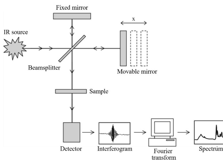
Figure II-24: Schematic representation of FTIR spectrometer (adapted from [156]).
