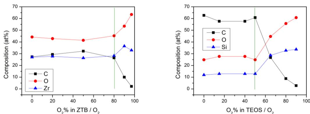
Figure III-11: Atomic composition of thin films deposited in ZTB/ $O_2$  and TEOS/ $O_2$  MMP-ECR plasma ( $p_{total} \approx 1$  mTorr,  $V_{substrate} = floating$ ) (adapted from [11] and [3], respectively).
