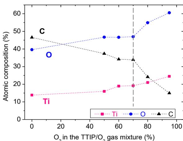
Figure III-9: Atomic composition of thin films deposited in TTIP/ $\text{O}_2$  plasma ( $p_{\text{total}} = 1$  mTorr;  $P_{\text{MW}} = 800$  W,  $V_{\text{substrate}} = \text{floating}$ ) as a function of  $\text{O}_2$  proportion in the gas mixture.
