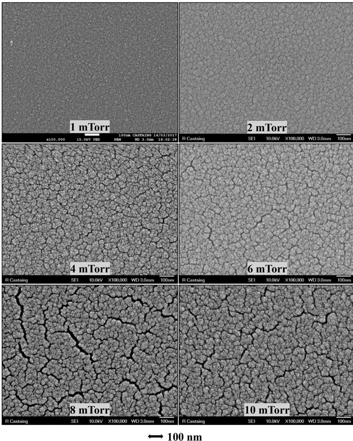
Figure IV-14: SEM surface images of thin films deposited at different total gas pressures in 5% TTIP/95%  $O_2$  plasma ( $P_{MW} = 800$  W,  $V_{substrate} = floating$ ).
