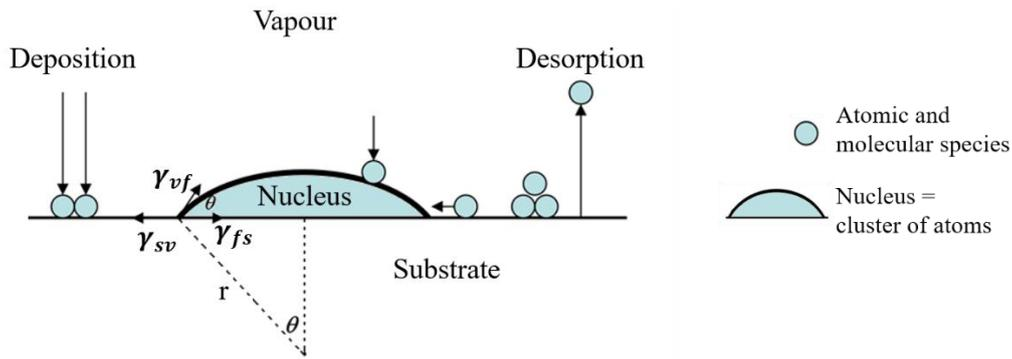
Figure I-1: Schematic representation of a nucleation process during vapour phase deposition (adapted from [14]).  $\theta$  is the substrate-nucleus contact angle;  $\gamma_{sv}$ ,  $\gamma_{fs}$  and  $\gamma_{vf}$  are the substrate-vapour, film-substrate and vapour-film interfacial tensions, respectively.
