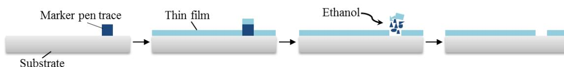
Figure II-23: Schematic presentation of the employed lift-off method.
