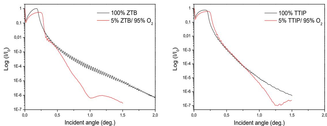
Figure III-43: XRR measurements of reflectivity as a function of an incident angle for thin films deposited in ZTB/O<sub>2</sub> and TTIP/O<sub>2</sub> plasmas ( $p_{total} = 1$  mTorr;  $P_{MW} = 800$  W,  $V_{substrate} = floating$ ).
