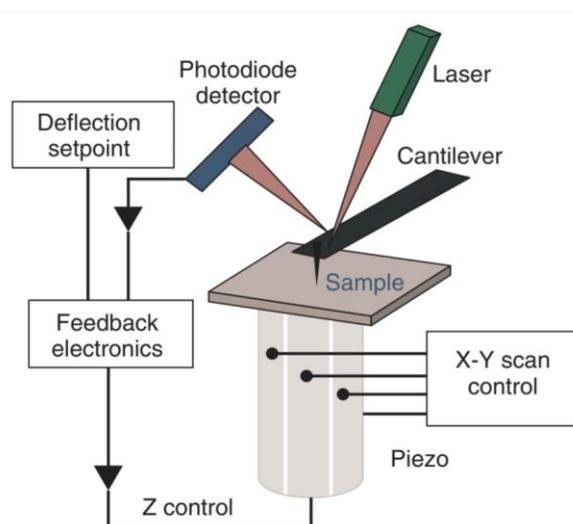
Figure II-27: Schematic representation of an AFM [158].
