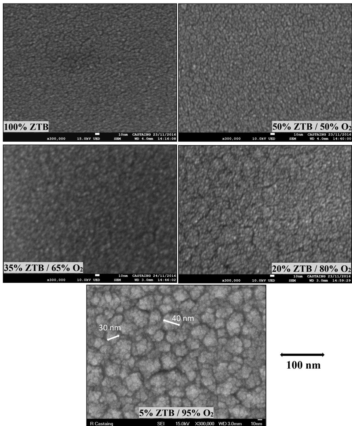
Figure III-31: SEM surface images of thin films deposited at different gas compositions in ZTB/O<sub>2</sub> plasma ( $p_{total} = 1$  mTorr,  $P_{MW} = 800$  W,  $V_{substrate} = floating$ ). Thin film thickness: 140-170 nm.
