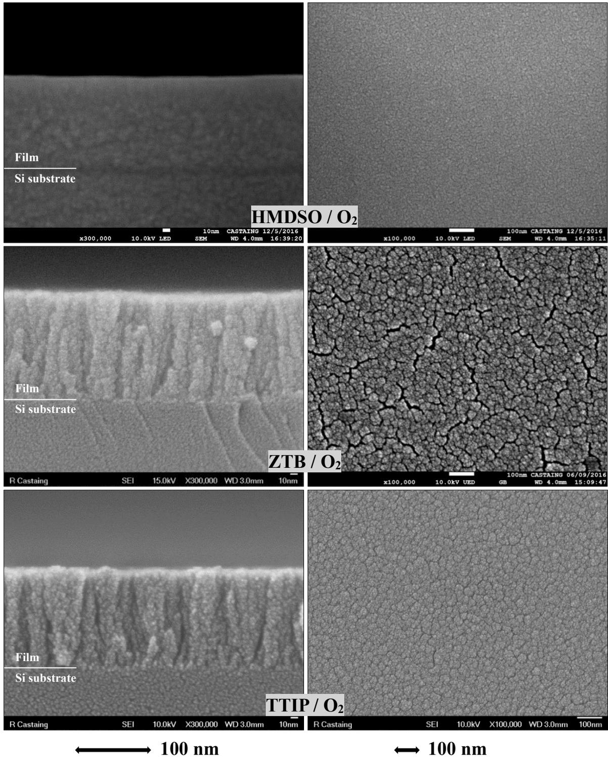
Figure V-12: SEM cross-sectional (left) and surface (right) images of silica-, zirconia- and titania-like thin films (gas mixture: 5% precursor/95% O<sub>2</sub>,  $p_{total}=2$  mTorr,  $P_{MW} = 800$  W,  $V_{substrate} = floating$ ).
