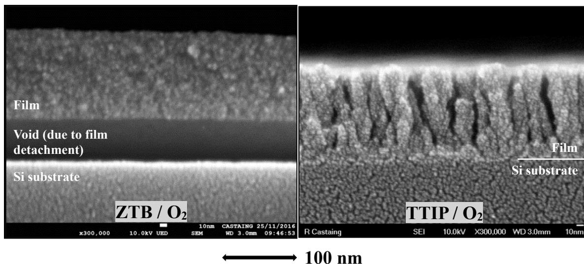
Figure IV-15: SEM cross-sectional images of thin films deposited at 10 mTorr in ZTB/O<sub>2</sub> and TTIP/O<sub>2</sub> plasmas (5% precursor/95% O<sub>2</sub>,  $P_{MW} = 800$  W,  $V_{substrate} = floating$ ).
