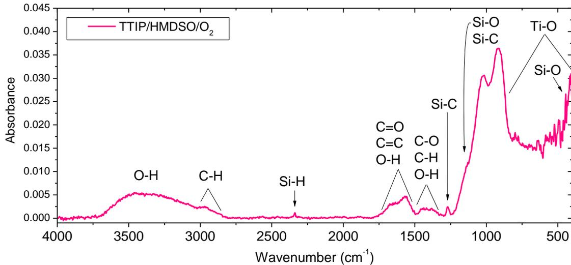
Figure V-6: FTIR spectrum of thin film deposited in 4% TTIP/13% HMDSO/83% O<sub>2</sub> plasma ( $p_{total} = 2.3$  mTorr;  $P_{MW} = 800$  W,  $V_{substrate} = floating$ ).
