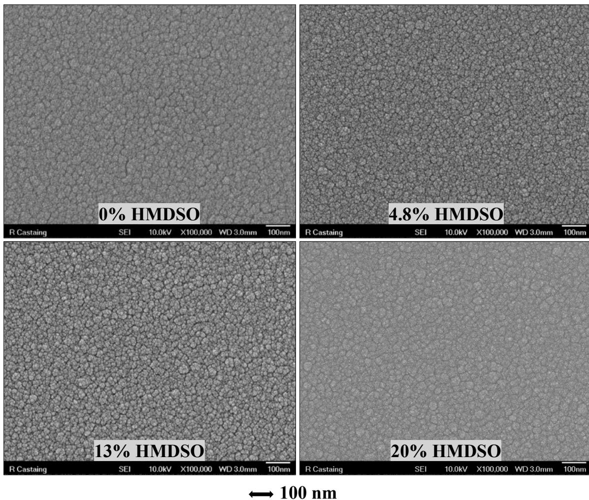
Figure V-16: SEM surface images of thin films deposited at different quantities of HMDSO in TTIP/HMDSO/O<sub>2</sub> plasma gas mixture ( $p_{total} = 2.0-2.5$  mTorr,  $P_{MW} = 800$  W,  $V_{substrate} = floating$ ).
