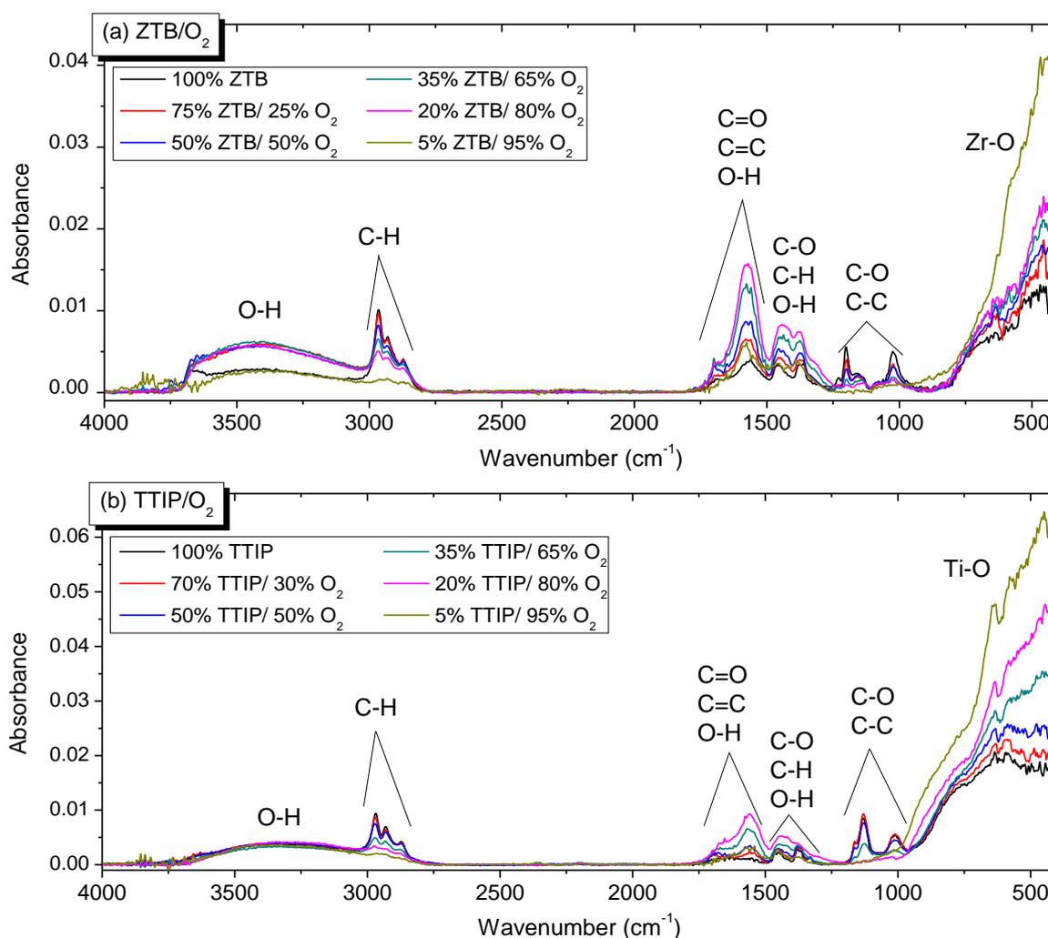
Figure III-22: FTIR spectra of thin films deposited at different O<sub>2</sub> proportion in ZTB/O<sub>2</sub> and TTIP/O<sub>2</sub> plasmas ( $p_{total} = 1$  mTorr,  $P_{MW} = 800$  W,  $V_{substrate} = floating$ ). Absorbance: normalised by thin film thickness.
