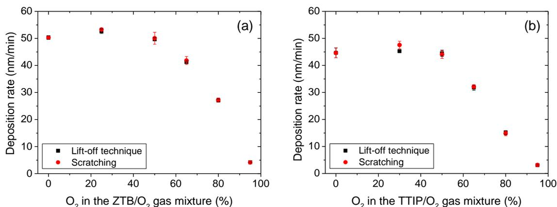
Figure III-6: Deposition rate of thin films deposited at different gas mixture ratios in (a) ZTB/O<sub>2</sub> and (b) TTIP/O<sub>2</sub> plasma ( $p_{total} = 1$  mTorr,  $P_{MW} = 800$  W,  $V_{substrate} = floating$ ). Error bars correspond to standard deviation.
