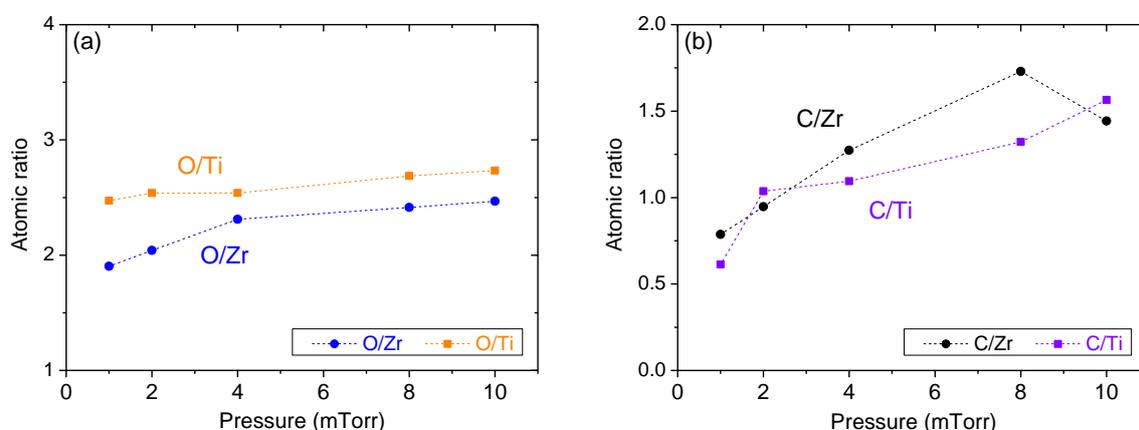
Figure IV-9: Evolution of (a) O/Zr and O/Ti, (b) C/Zr and C/Ti atomic ratios in thin films deposited at different total gas pressures in ZTB/ $\text{O}_2$  and TTIP/ $\text{O}_2$  plasma (5% precursor/95%  $\text{O}_2$ ,  $P_{MW} = 800$  W,  $V_{\text{substrate}} = \text{floating}$ ).
