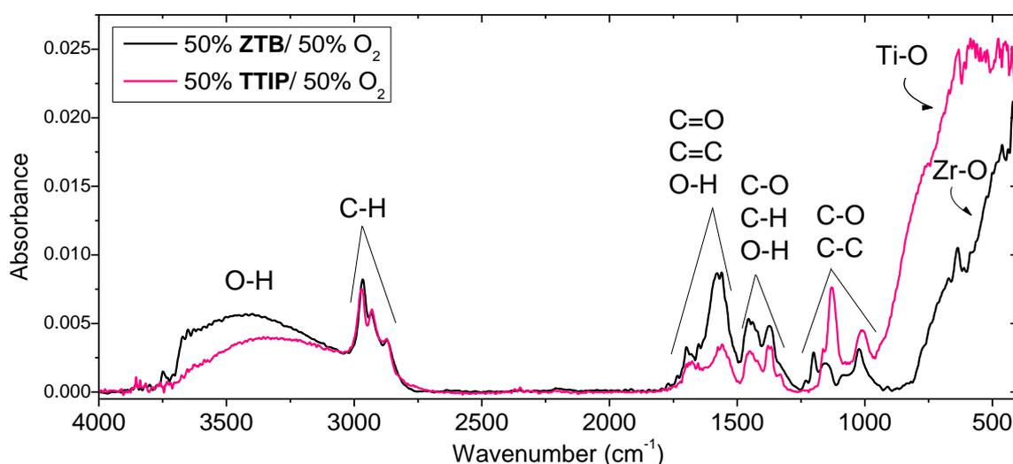
Figure III-19: FTIR spectra of thin films deposited in ZTB/O<sub>2</sub> and TTIP/O<sub>2</sub> plasmas ( $p_{total} = 1$  mTorr,  $P_{MW} = 800$  W,  $V_{substrate} = floating$ ). Absorbance: normalised by thin film thickness.
