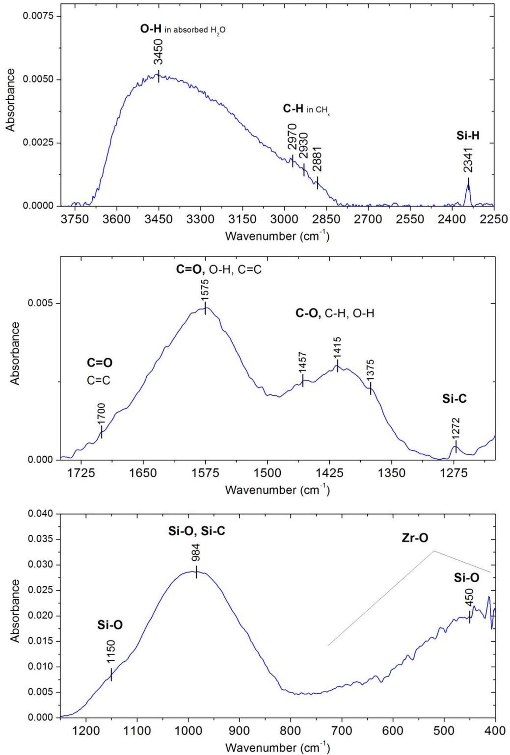
Figure A-3: FTIR spectrum of thin film deposited in 4% ZTB / 13% HMDSO / 83%  $\text{O}_2$  plasma ( $p_{\text{total}} = 2.3 \text{ mTorr}$ ,  $P_{\text{MW}} = 800 \text{ W}$ ,  $V_{\text{substrate}} = \text{floating}$ ).
