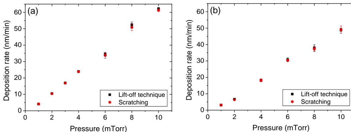
Figure IV-1: Deposition rate of thin films grown at various total gas pressures in (a) ZTB/O<sub>2</sub> and (b) TTIP/O<sub>2</sub> plasma (5% precursor/95% O<sub>2</sub>,  $P_{MW} = 800$  W,  $V_{substrate} = floating$ ). Error bars correspond to standard deviation.
