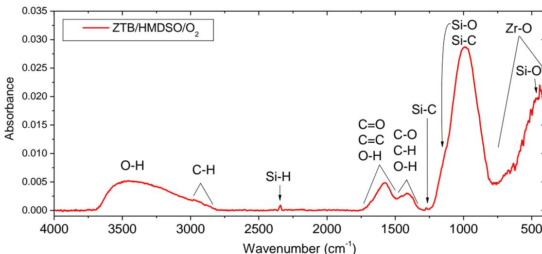
Figure V-5: FTIR spectrum of thin film deposited in 4% ZTB/13% HMDSO/83% O<sub>2</sub> plasma ( $p_{total} = 2.3$  mTorr,  $P_{MW} = 800$  W,  $V_{substrate} = floating$ ).
