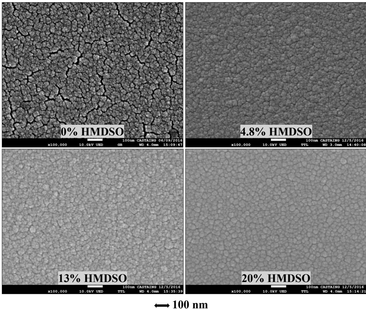
Figure V-14: SEM surface images of thin films deposited at different quantities of HMDSO in ZTB/HMDSO/O<sub>2</sub> plasma gas mixture ( $p_{total} = 2.0\text{-}2.5$  mTorr,  $P_{MW} = 800$  W,  $V_{substrate} = floating$ ).
