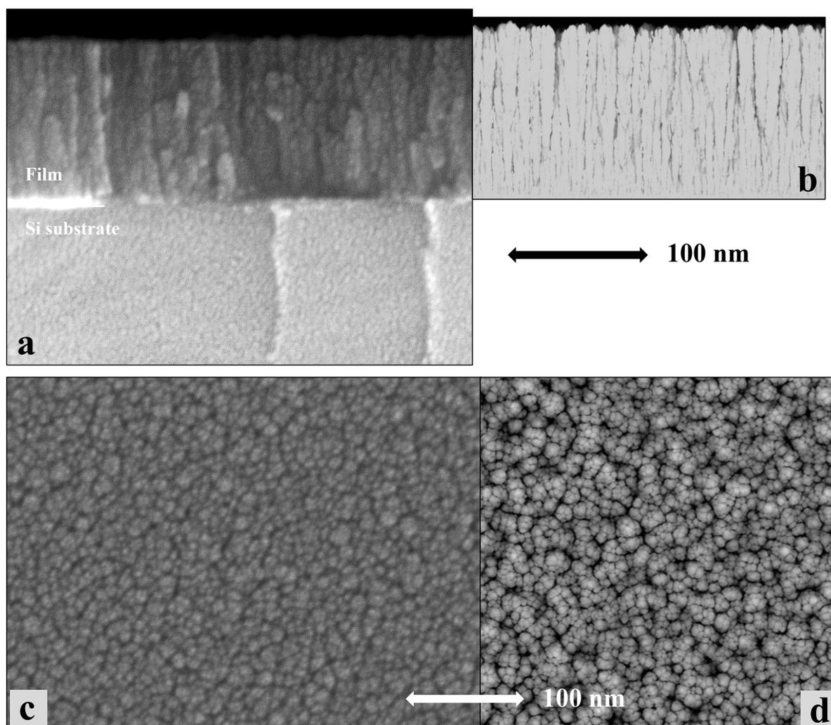
Figure III-41: Cross-sectional and surface images of thin films obtained by (a, c) PECVD from TTIP/O<sub>2</sub>, (b, d) MC simulation of TiO<sub>2</sub>. PECVD process parameters: 5% TTIP/95% O<sub>2</sub>,  $p_{total} = 1$  mTorr,  $P_{MW} = 800$  W,  $V_{substrate} = floating$ . MC model parameters: possible surface relaxation, isotropic flux.
