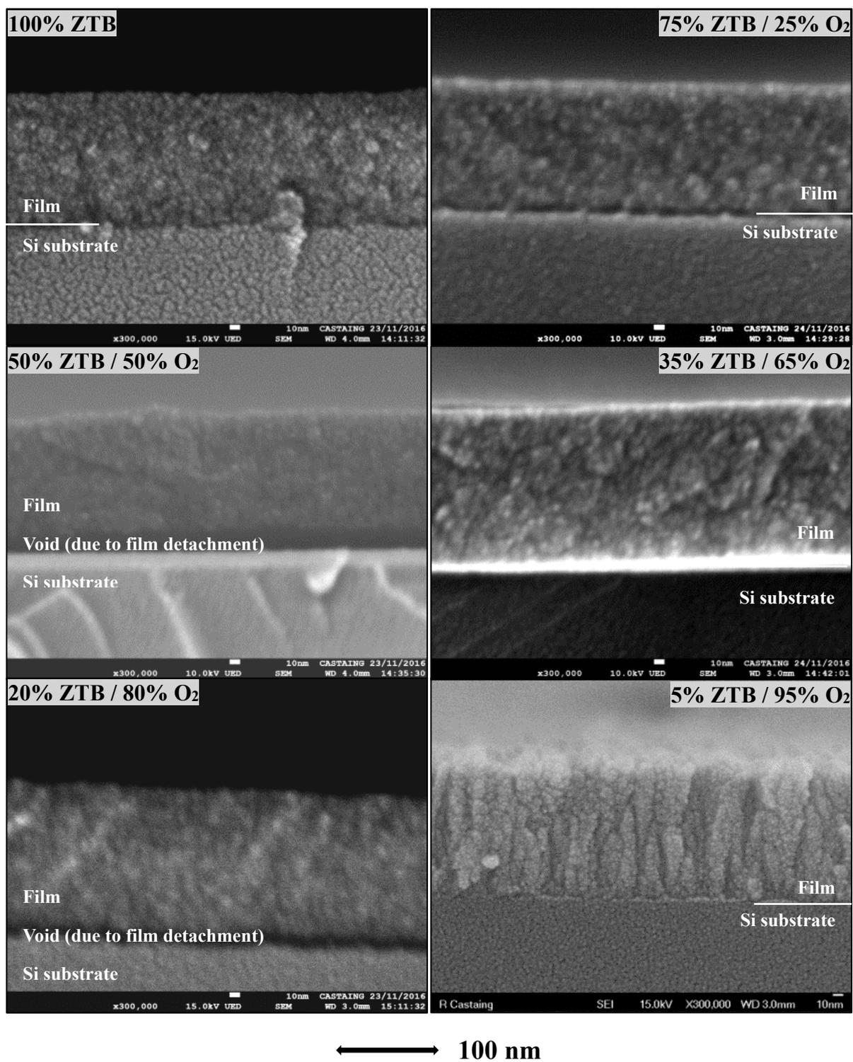
Figure III-30: SEM cross-sectional images of thin films deposited at different gas compositions in ZTB/O<sub>2</sub> plasma ( $p_{total} = 1$  mTorr,  $P_{MW} = 800$  W,  $V_{substrate} = floating$ ). Thin film thickness: 140-170 nm.
