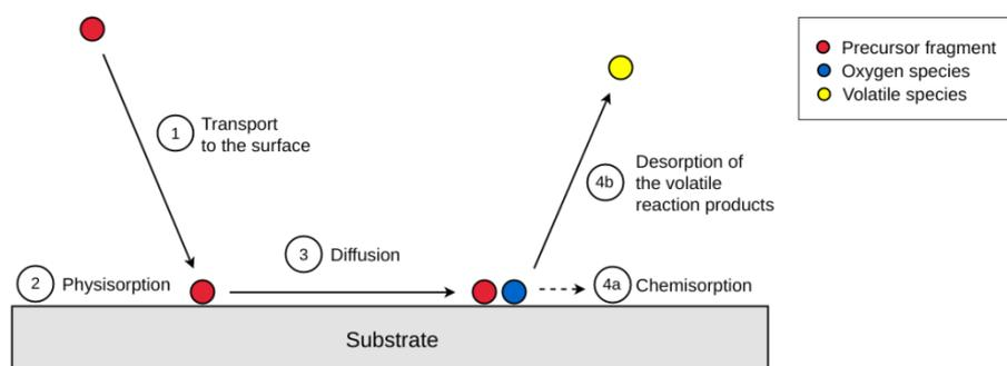
Figure III-35: Simplified schematic representation of the “sticking mechanism”.
