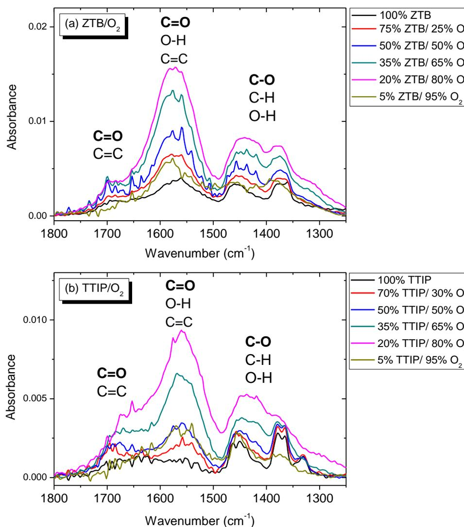
Figure III-24: FTIR spectra (1800-1250 cm<sup>-1</sup>) of thin films deposited at different proportion of O<sub>2</sub> gas in a) ZTB/O<sub>2</sub> and b) TTIP/O<sub>2</sub> gas mixture ( $p_{total} = 1$  mTorr,  $P_{MW} = 800$  W,  $V_{substrate} = floating$ ). Absorbance: normalised by thin film thickness.
