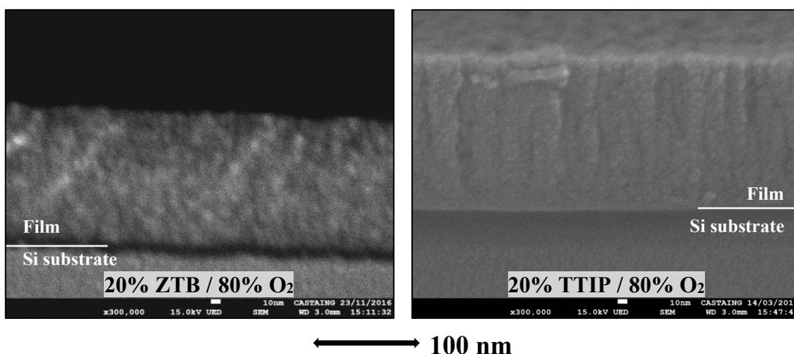
Figure III-36: SEM cross-sectional images of thin films deposited in 20% ZTB/80% O<sub>2</sub> and 20% TTIP/80% O<sub>2</sub> plasmas ( $p_{total} = 1$  mTorr,  $P_{MW} = 800$  W,  $V_{substrate} = floating$ ).
