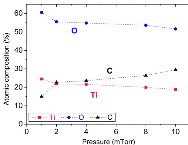
Figure IV-3: Atomic composition of thin films deposited in TTIP/ $\text{O}_2$  plasma as a function of total gas pressure (5% precursor/95%  $\text{O}_2$ ,  $P_{MW} = 800$  W,  $V_{substrate} = \text{floating}$ ).
