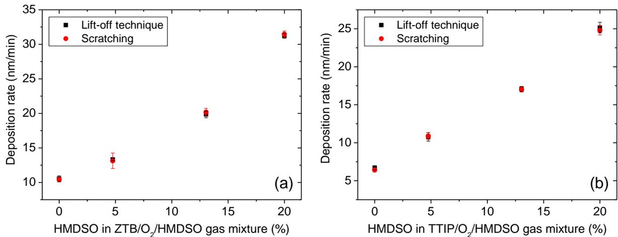
Figure V-1: Deposition rate of thin films grown in (a) ZTB/HMDSO/O<sub>2</sub> and (b) TTIP/HMDSO/O<sub>2</sub> plasma ( $p_{total}=2.0-2.5$  mTorr,  $P_{MW} = 800$  W,  $V_{substrate} = floating$ ). Error bars correspond to standard deviation.
