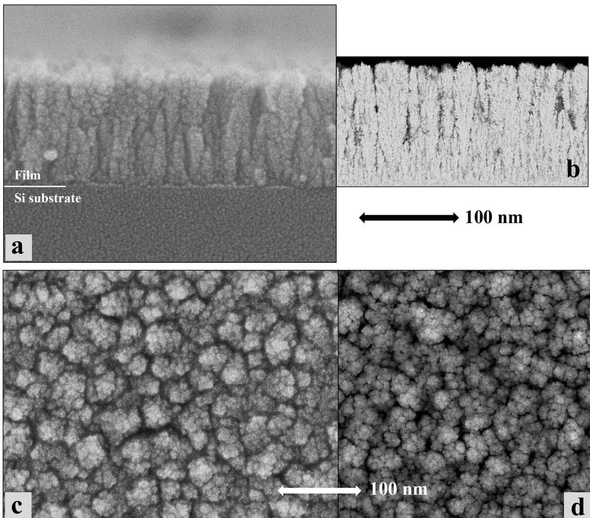
Figure III-39: Cross-sectional and surface images of thin films obtained by (a, c) PECVD from ZTB/ $\text{O}_2$ , (b, d) MC simulation of  $\text{ZrO}_2$ . PECVD process parameters: 5% ZTB/ 95%  $\text{O}_2$ ,  $p_{\text{total}} = 1 \text{ mTorr}$ ,  $P_{\text{MW}} = 800 \text{ W}$ ,  $V_{\text{substrate}} = \text{floating}$ . MC model parameters: isotropic flux, no relaxation at the surface.
