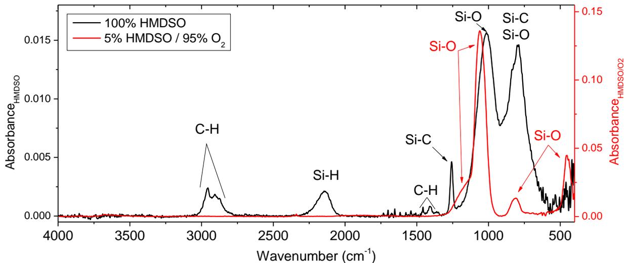
Figure V-4: FTIR spectra corresponding to thin films deposited in 100% HMDSO ( $p_{total} = 1$  mTorr) and in 5% HMDSO/95% O<sub>2</sub> ( $p_{total} = 2$  mTorr) plasma ( $P_{MW} = 800$  W,  $V_{substrate} = floating$ ).
