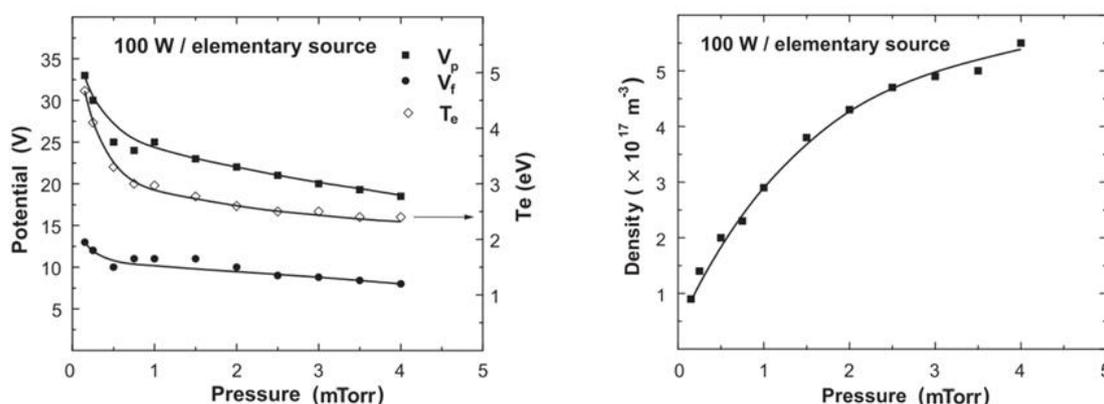
Figure II-7: Plasma potential, floating potential and  $T_e$  (a), and plasma density (b) as a function of Ar pressure (cylindrical reactor, 20 elementary plasma sources, 100 W per source) (adapted from [148]).
