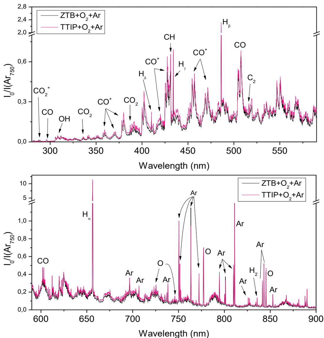
Figure III-2: Optical emission spectra of ZTB/O<sub>2</sub>/Ar and TTIP/O<sub>2</sub>/Ar plasma normalised by Ar spectral line intensity at 750 nm ( $p_{\text{precursor}} = 0.50$  mTorr,  $p_{\text{oxygen gas}} = 0.50$  mTorr,  $p_{\text{Ar gas}} = 0.05$  mTorr,  $P_{\text{MW}} = 800$  W).
