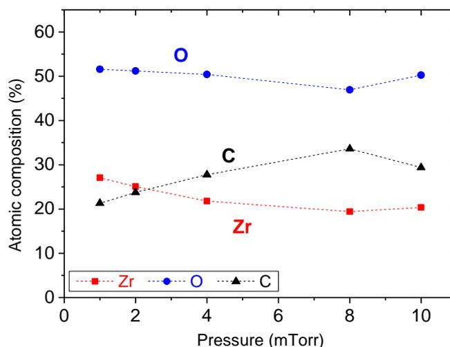
Figure IV-2: Atomic composition of thin films deposited in ZTB/O<sub>2</sub> plasma as a function of total gas pressure (5% precursor/95% O<sub>2</sub>, P<sub>MW</sub> = 800 W, V<sub>substrate</sub> = floating).
