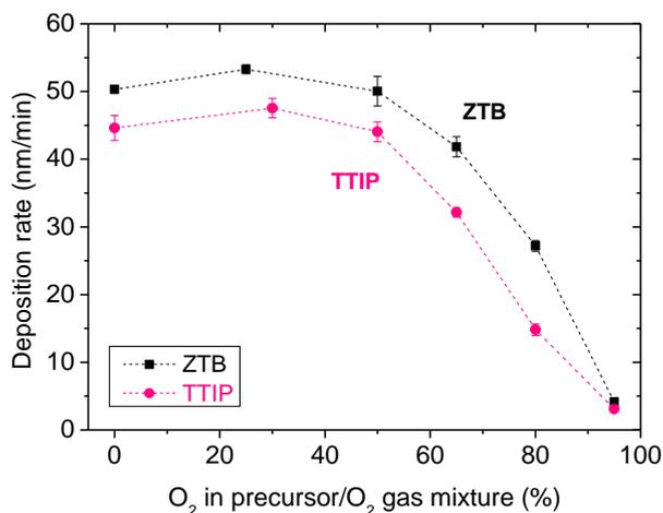
Figure III-7: Deposition rate of thin films deposited at different gas mixture ratios in ZTB/O<sub>2</sub> and TTIP/O<sub>2</sub> plasma ( $p_{\text{total}} = 1$  mTorr,  $P_{\text{MW}} = 800$  W,  $V_{\text{substrate}} = \text{floating}$ ). Error bars correspond to standard deviation.
