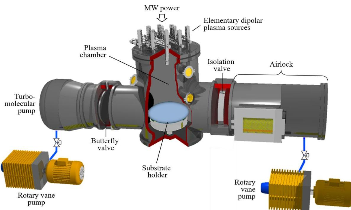
Figure II-8: 3D representation of the reactor Pixcell.
