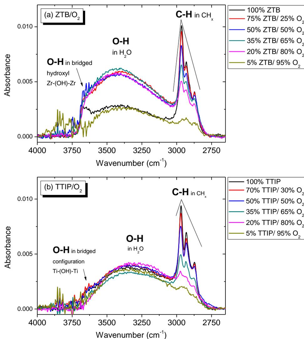
Figure III-23: FTIR spectra (3750-2750  $\text{cm}^{-1}$ ) of thin films deposited at different proportion of  $\text{O}_2$  gas in a) ZTB/ $\text{O}_2$  and b) TTIP/ $\text{O}_2$  gas mixture ( $p_{\text{total}} = 1 \text{ mTorr}$ ,  $P_{\text{MW}} = 800 \text{ W}$ ,  $V_{\text{substrate}} = \text{floating}$ ). Absorbance: normalised by thin film thickness.
