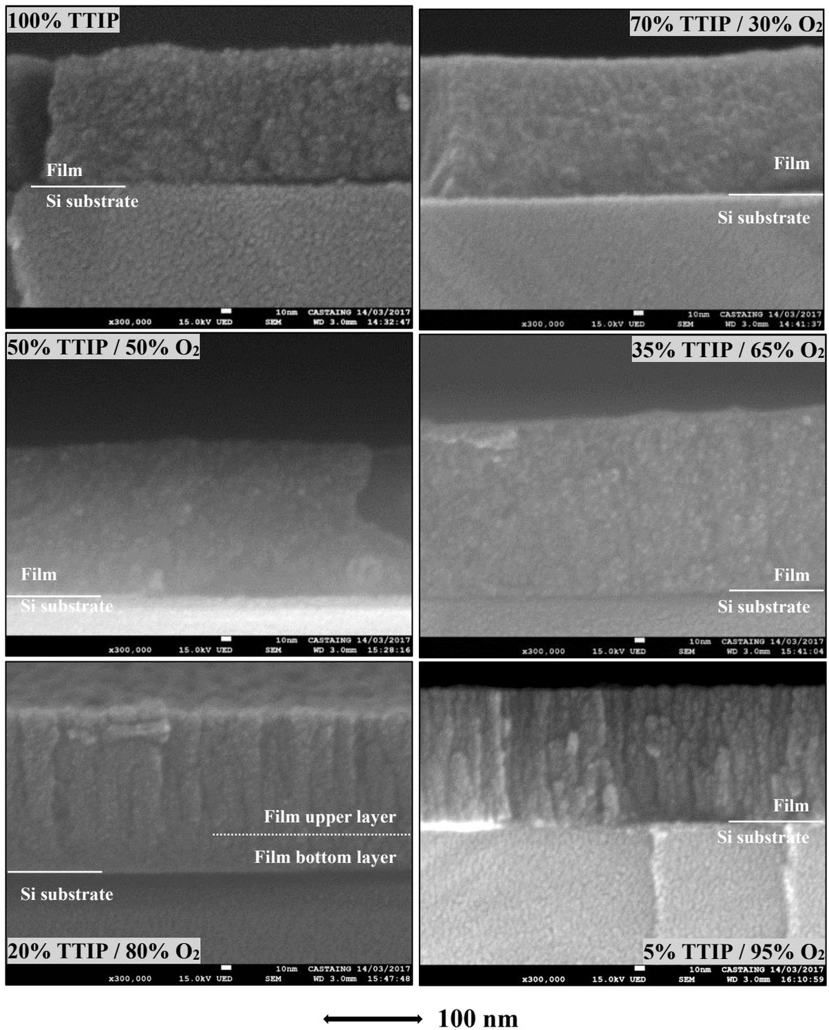
Figure III-33: SEM cross-sectional images of thin films deposited at different gas mixture ratios in TTIP/O<sub>2</sub> plasma ( $p_{total} = 1$  mTorr;  $P_{MW} = 800$  W,  $V_{substrate} = floating$ ). Thin film thickness: 120-170 nm.
