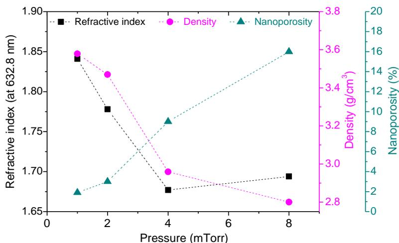
Figure IV-16: Refractive index, density and nanoporosity fraction of thin films deposited in ZTB/O<sub>2</sub> plasma as a function of total gas pressure (5% ZTB/95% O<sub>2</sub>,  $P_{MW} = 800$  W,  $V_{substrate} = floating$ ).
