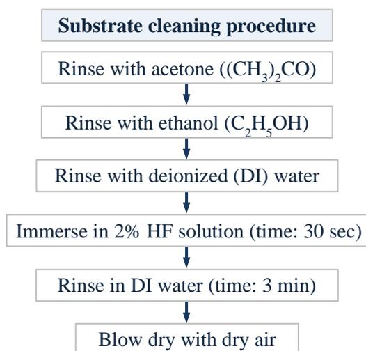
Figure II-15: Steps of the silicon substrate cleaning procedure.
