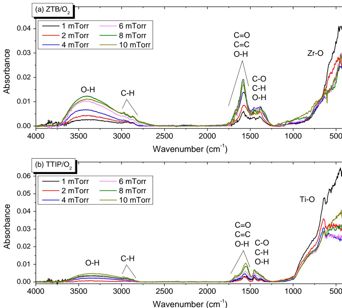
Figure IV-4: FTIR spectra of thin films deposited at different total gas pressures in ZTB/ $\text{O}_2$  and TTIP/ $\text{O}_2$  plasma (5% precursor/95%  $\text{O}_2$ ,  $P_{MW} = 800$  W,  $V_{\text{substrate}} = \text{floating}$ ). Absorbance: normalised by film thickness.
