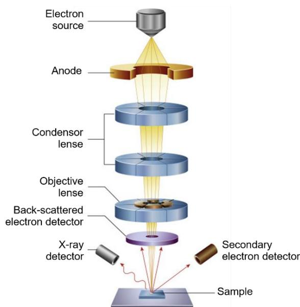
Figure II-26: Schematic representation of an SEM [157].
