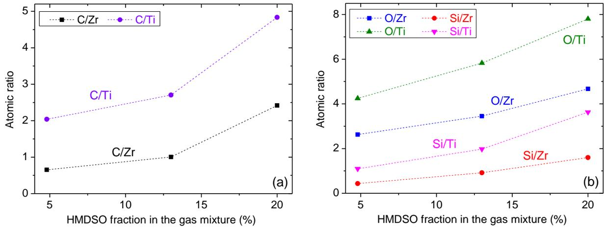
Figure V-11: Evolution of film atomic composition ratios (a) C/M, (b) Si/M and O/M, (M: Zr or Ti) as a function of HMDSO addition to the ZTB/HMDSO/O<sub>2</sub> and TTIP/HMDSO/O<sub>2</sub> gas mixtures ( $p_{total} = 2.0-2.5$  mTorr,  $P_{MW} = 800$  W,  $V_{substrate} = floating$ ).
