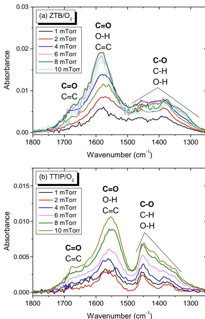
Figure IV-6: FTIR spectra (1800-1250  $\text{cm}^{-1}$ ) of thin films deposited at different total gas pressures in a) ZTB/ $\text{O}_2$  and b) TTIP/ $\text{O}_2$  gas mixture (5% precursor/95%  $\text{O}_2$ ,  $P_{MW} = 800$  W,  $V_{\text{substrate}} = \text{floating}$ ).
