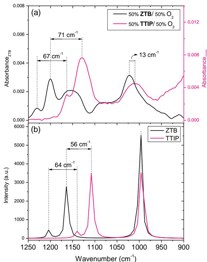
Figure III-21: Comparison of  $1250\text{-}900\text{ cm}^{-1}$  spectral region corresponding to: (a) thin films deposited in ZTB/ $\text{O}_2$  and TTIP/ $\text{O}_2$  plasmas ( $p_{\text{total}} = 1\text{ mTorr}$ ,  $P_{\text{MW}} = 800\text{ W}$ ,  $V_{\text{substrate}} = \text{floating}$ ; absorbance: normalised by film thickness); (b) ZTB and TTIP molecules synthetic IR spectra obtained by DFT calculations.
