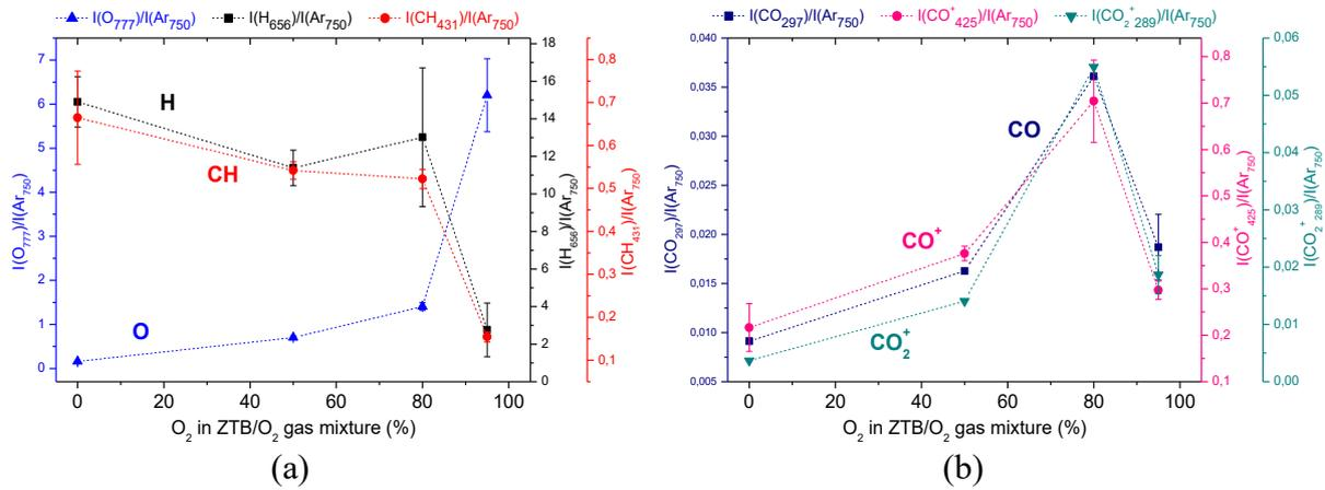
Figure III-3: Evolution of spectral line intensity ratios as a function of O<sub>2</sub> gas percentage of ZTB/O<sub>2</sub> gas mixture ( $p_{ZTB+O_2} = 1 \text{ mTorr}$ ,  $p_{Ar \text{ gas}} = 0.05 \text{ mTorr}$ ,  $P_{MW} = 800 \text{ W}$ ): (a)  $I(O)/I(Ar)$ ,  $I(H)/I(Ar)$ ,  $I(CH)/I(Ar)$ , (b)  $I(CO)/I(Ar)$ ,  $I(CO^+)/I(Ar)$ ,  $I(CO_2^+)/I(Ar)$ .
