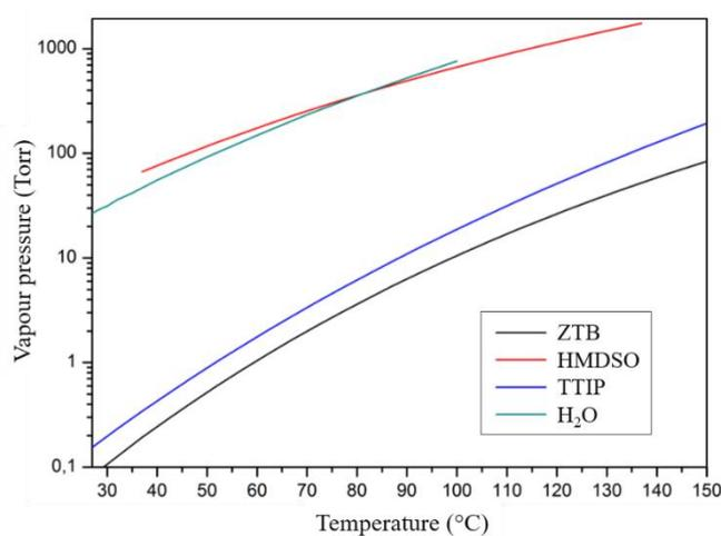
Figure II-10: Vapour pressure as a function of temperature for: H<sub>2</sub>O, HMDSO, ZTB and TTIP [12].
