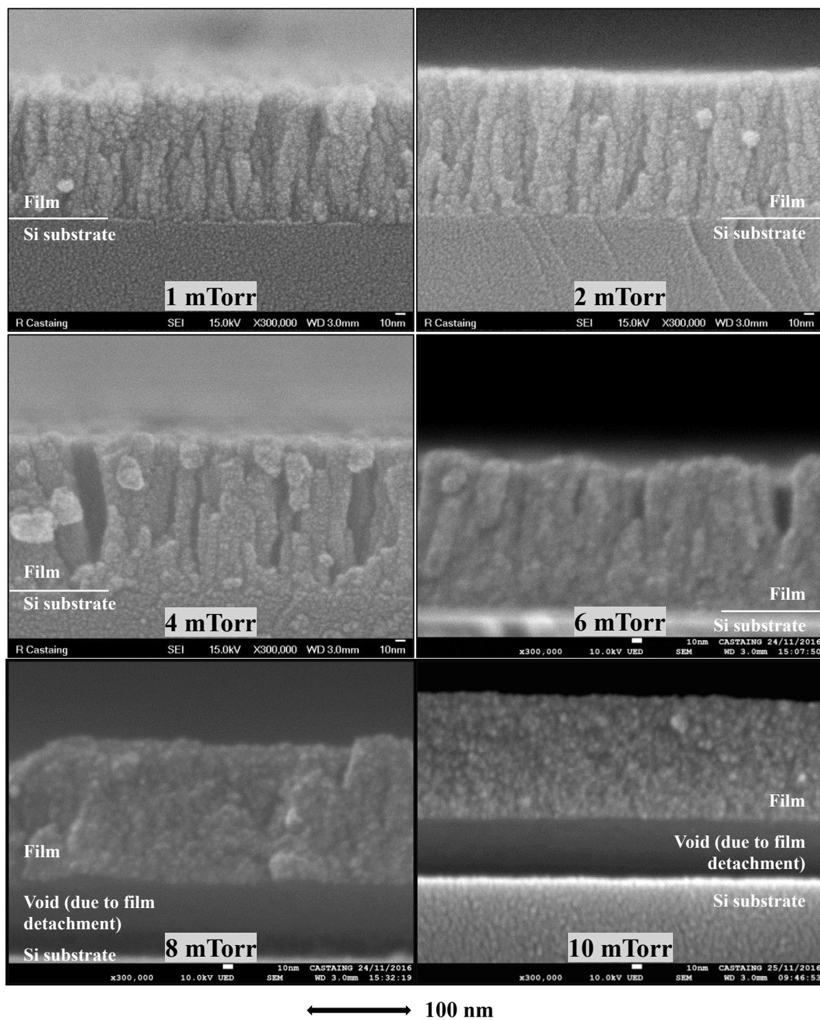
Figure IV-10: SEM cross-sectional images of thin films deposited at different total gas pressures in 5% ZTB/95%  $O_2$  plasma ( $P_{MW} = 800$  W,  $V_{substrate} = floating$ ).
