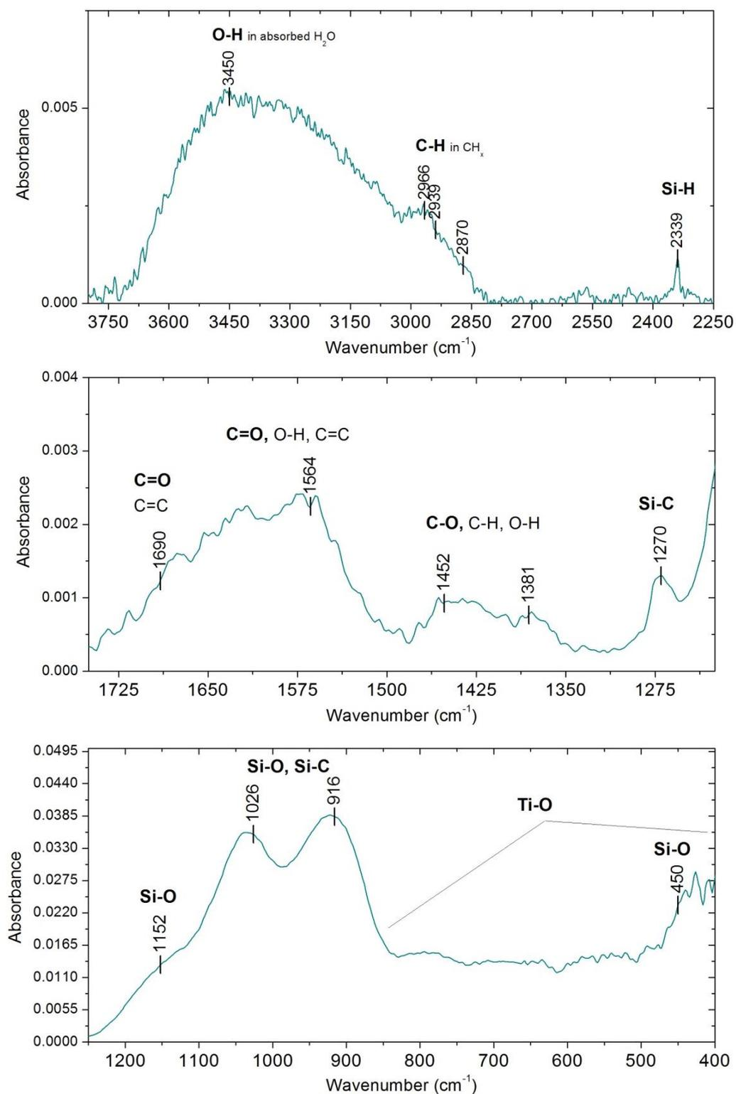
Figure A-4: FTIR spectrum of thin film deposited in 4% TTIP / 13% HMDSO / 83% O<sub>2</sub> plasma ( $p_{total} = 2.3$  mTorr,  $P_{MW} = 800$  W,  $V_{substrate} = floating$ ).
