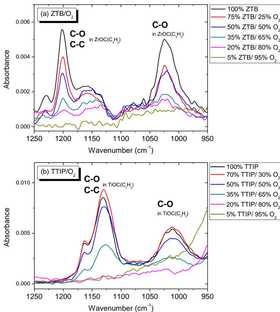
Figure III-26: FTIR spectra ( $1250\text{-}950\text{ cm}^{-1}$ ) of thin films deposited at different proportion of  $\text{O}_2$  gas in ZTB/ $\text{O}_2$  and TTIP/ $\text{O}_2$  gas mixture ( $p_{\text{total}} = 1\text{ mTorr}$ ,  $P_{\text{MW}} = 800\text{ W}$ ,  $V_{\text{substrate}} = \text{floating}$ ). Absorbance: normalised by thin film thickness.
