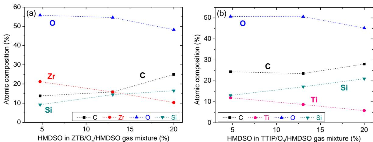
Figure V-3: Atomic composition of thin films deposited in (a) ZTB/HMDSO/O<sub>2</sub> and (b) TTIP/HMDSO/O<sub>2</sub> plasma as a function of gas mixture composition ( $p_{total} = 2.0-2.5$  mTorr,  $P_{MW} = 800$  W,  $V_{substrate} = floating$ ).
