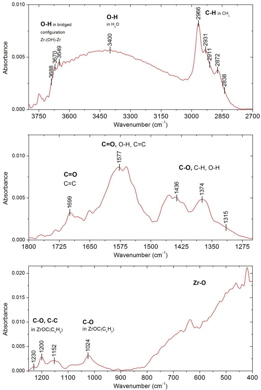
Figure A-1: FTIR spectrum of thin film deposited in 50% ZTB / 50%  $\text{O}_2$  plasma ( $p_{\text{total}} = 1 \text{ mTorr}$ ,  $P_{\text{MW}} = 800 \text{ W}$ ,  $V_{\text{substrate}} = \text{floating}$ ).
