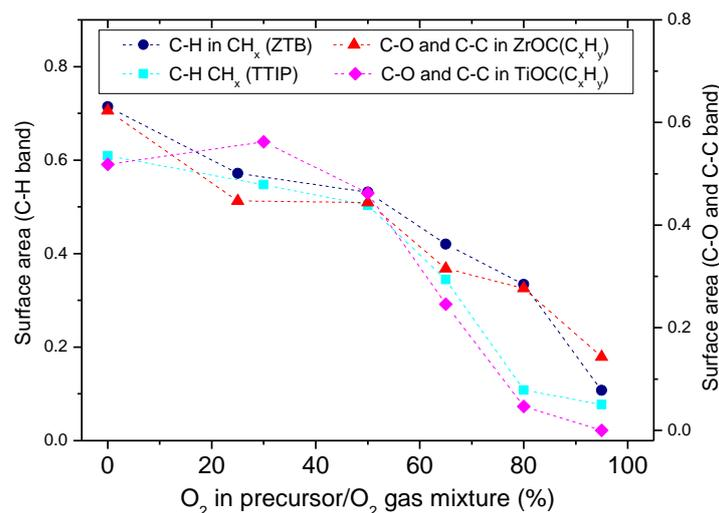
Figure III-27: Change in surface area of FTIR peaks corresponding to films deposited in ZTB/O<sub>2</sub> and TTIP/O<sub>2</sub> plasmas: 3050-2800 cm<sup>-1</sup> band (C-H in CH<sub>x</sub>); 1250-950 cm<sup>-1</sup> band (C-O and C-C in metal alkoxide groups).
