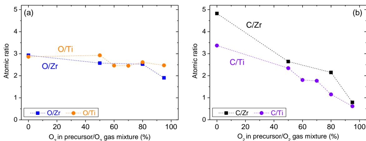
Figure III-10: Evolution of (a) O/Zr and O/Ti, (b) C/Zr and C/Ti atomic ratios in thin films deposited at different gas mixtures in ZTB/O<sub>2</sub> and TTIP/O<sub>2</sub> plasma ( $p_{total} = 1$  mTorr,  $P_{MW} = 800$  W,  $V_{substrate} = floating$ ).
