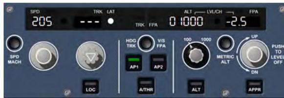
(a) Flight Control Unit (FCU) adjustment.
