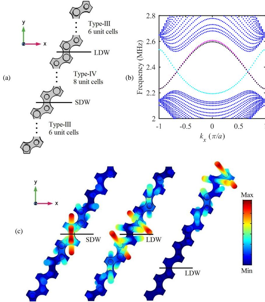
Figure 2.18: (a) Schematic of the proposed three-layers ribbon supercell constructed by sandwiching eight unit cells of type-IV PPnC in between two sets of six unit cells of type-III PPnC. (b) Antisymmetric dispersion curves of the ribbon supercell. (c) Eigenmode of the edge states (magenta and cyan branches) and locally resonant mode (black branch) at the wave vector  $k_x = 0.5\pi/a$ .
