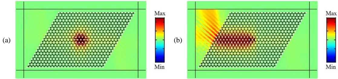
Figure 2.10: Plots of the magnitude of the out-of-plane displacement on the top surface of the plate under the excitation of the  $K2'$ -polarized (a)  $SH_0$  and (b)  $A_0$  Lamb waves at frequency 4.325MHz. The straight wave guide is constructed by inverting the position of type-I and type-II PPnCs as illustrated in figure 2.9(a).
