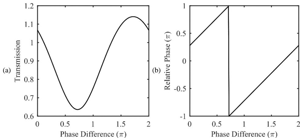
Figure 3.11: (a) Transmission coefficient against the phase difference of the external pressure when the magnitude is assumed to be 0.5MPa. (b) Relative phase between the transmitted amplitude  $A_{transEx}$  and  $A_{transIn}$ .
