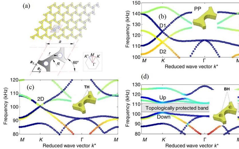
Figure 2.3: (a) A triangular-hole patterned phononic crystal plate. Perspective view of the patterned unit cells and the corresponding band structures: (b) patterned plate (PP), (c) plate with additional circular holes drilled through the thickness (TH) and (d) with blind holes (BH). [143]
