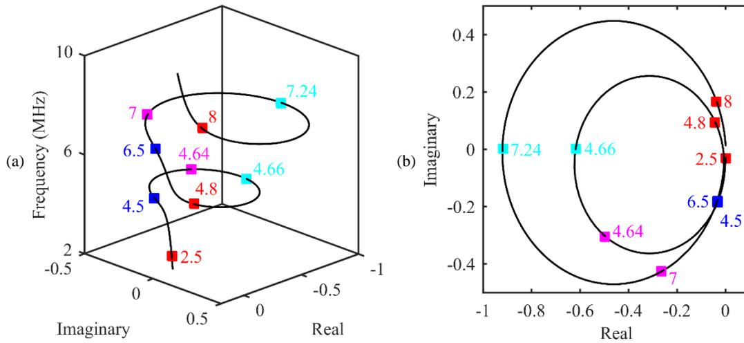
Figure 3.3: (a) Evolution of the complex amplitude of the reemitted Lamb wave against the frequency. (b) Top view (see from the positive  $z$ -axis) of the curve displayed in (a). The bending resonance B2 and the compressional resonance C1 are separated.
