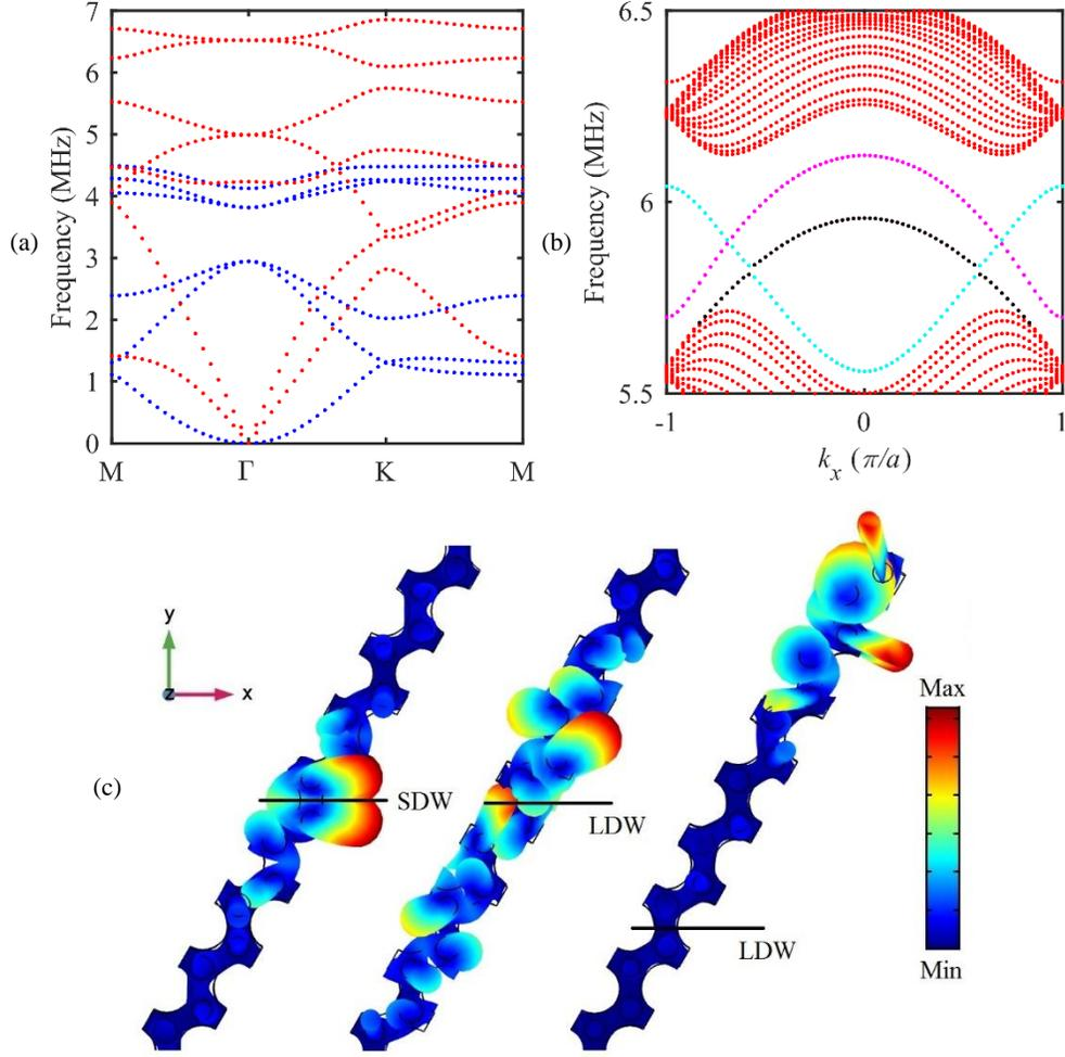
Figure 2.25: (a) Band structure of the perturbed PPnC with the diameter perturbation  $\Delta d_v = 10\mu\text{m}$ . (b) Symmetric dispersion curves of the ribbon supercell. (c) Eigenmodes of the edge states (magenta and cyan branches) and the locally resonant mode (black branch) at the wave vector  $k_x = 0.5\pi/a$ .
