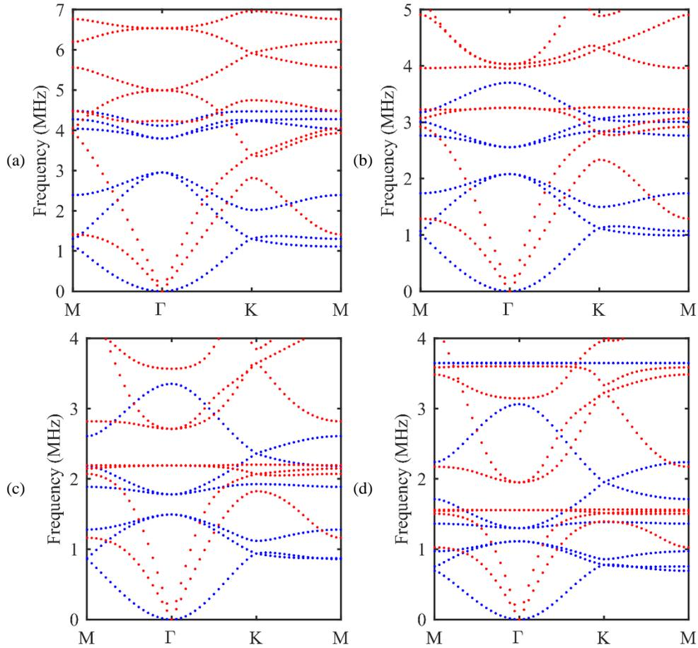
Figure 2.14: Band structures of the symmetric double-sided PPnCs with the height of the pillars set to be (a) 80 $\mu\text{m}$ , (b) 120 $\mu\text{m}$ , (c) 160 $\mu\text{m}$  and (d) 200 $\mu\text{m}$  respectively.
