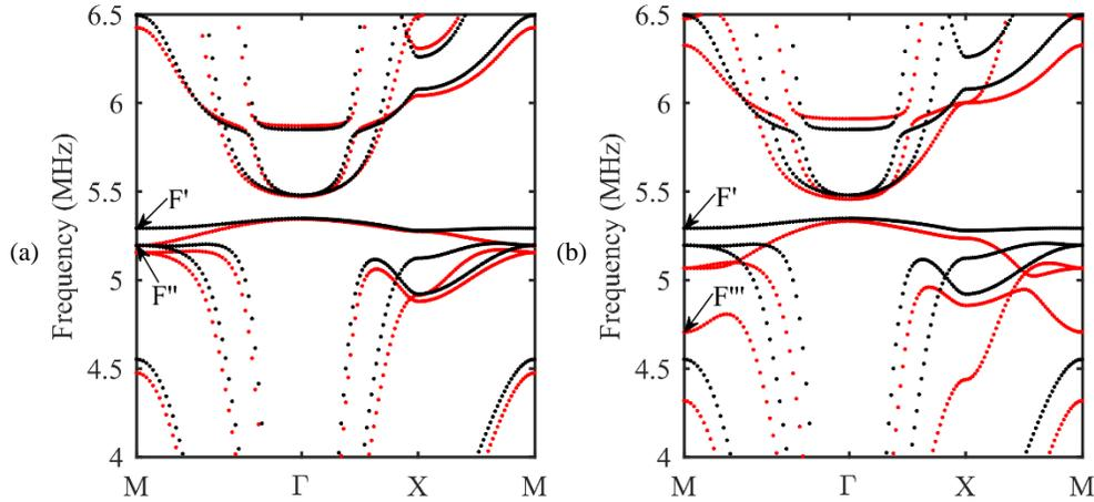
Figure 1.8: Band structures (red dotted lines) after introducing perforated holes with the diameter  $60\mu\text{m}$  (a) and  $100\mu\text{m}$  (b) at the four corners of the square lattice unit cell of the proposed ADPM. The band structure of ADPM without perforated holes is shown as the black dotted lines for reference.
