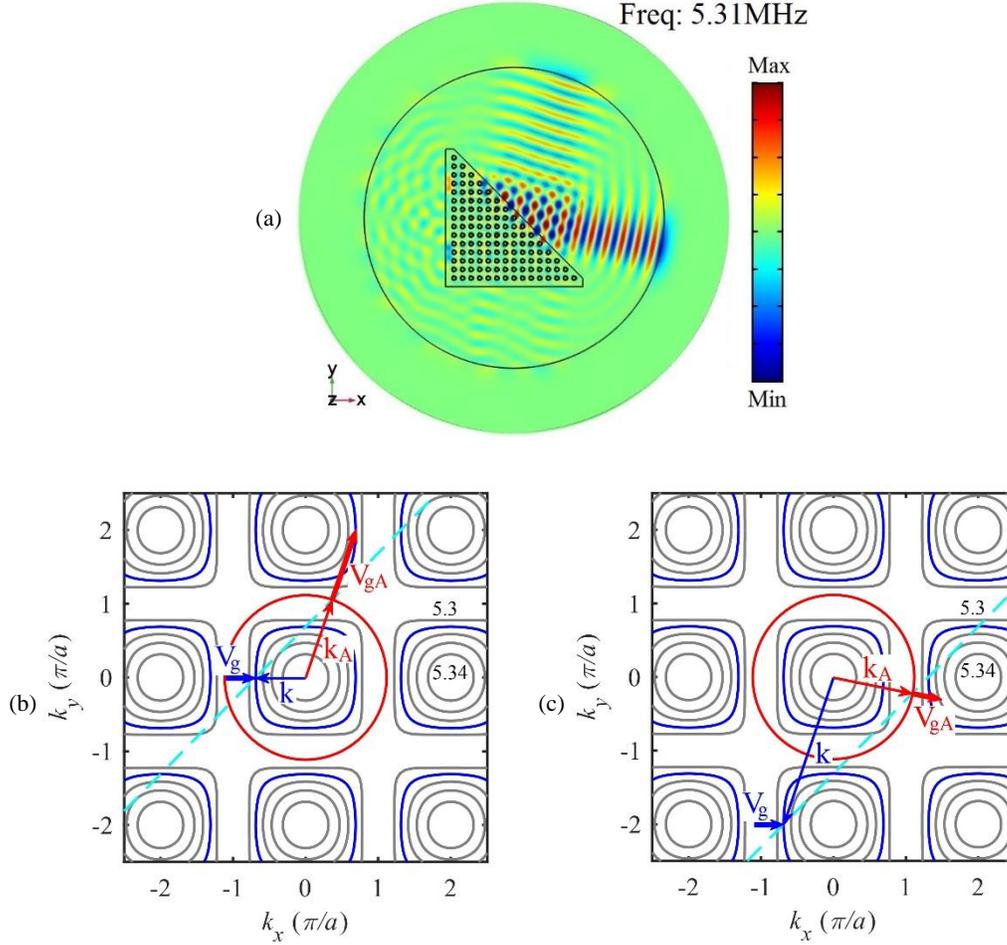
Figure 1.19: (a) Plot of the out-of-plane displacement on the top surface of the plate under the excitation of an incident  $SH_0$  mode at frequency 5.31MHz. EFCs analysis of (b) the negative and (c) the positive refraction at the outlet interface. The transmitted wave is assumed to be  $A_0$  mode only.
