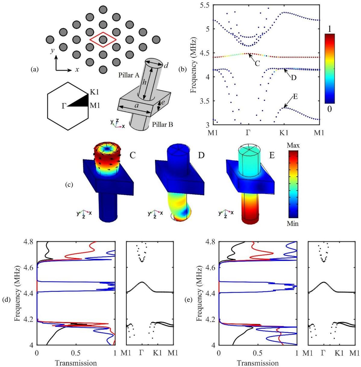
Figure 2.4: (a) Schematic of the proposed asymmetric double-sided PPnC arranged in the triangular lattice and (b) the corresponding band structure. (c) Eigenmodes at points C, D and E labelled in (b) and the black arrows represent the elastic deformation vectors. Transmission spectra of incident  $A_0$  (black),  $S_0$  (red) and  $SH_0$  (blue) Lambs wave propagating along (d)  $\Gamma K1$  and (e)  $\Gamma M1$  directions.
