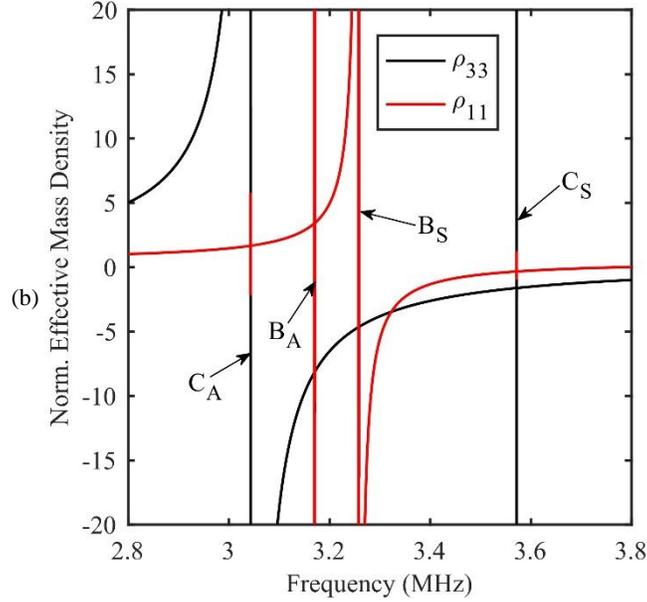
Figure 1.13: (a) Eigenmodes of the unit cell at the four representative resonance frequencies upon excitation  $(Ae^{i\omega t}, 0, 0)$ . (b) Effective mass density matrix components  $\rho_{11}$  (red) and  $\rho_{33}$  (black) normalized to the mass density of steel as a function of the excitation frequency.
