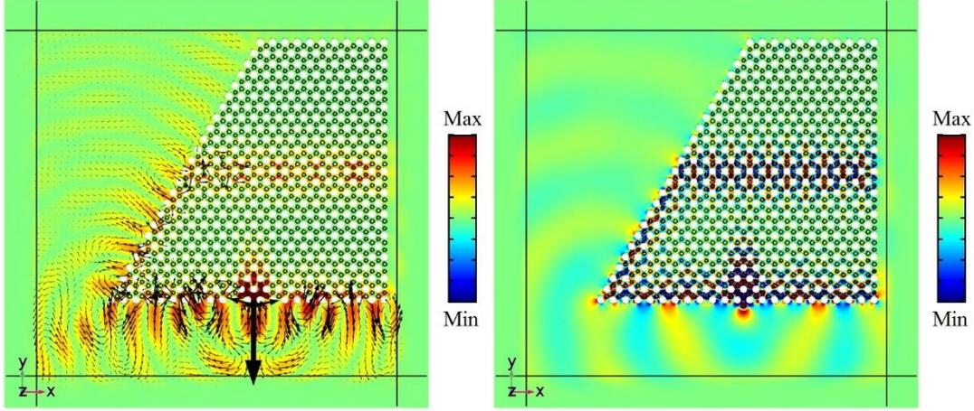
Figure 2.23: Plots of the magnitude of the in-plane displacement (left panel) and the out-of-plane displacement (right panel) on the top surface of the plate under the excitation of a  $z$ -polarized point source at the bottom interface.
