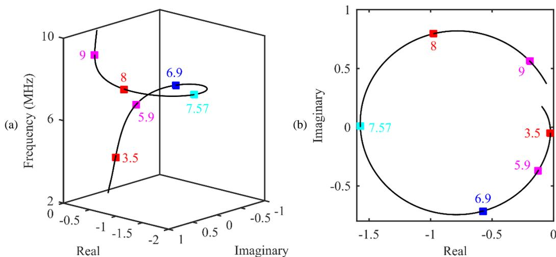
Figure 3.4: (a) Evolution of the complex amplitude of the reemitted Lamb wave against the frequency. (b) Top view (see from the positive  $z$ -axis) of the curve displayed in (a). The bending resonance B2 and the compressional resonance C1 are superimposed.
