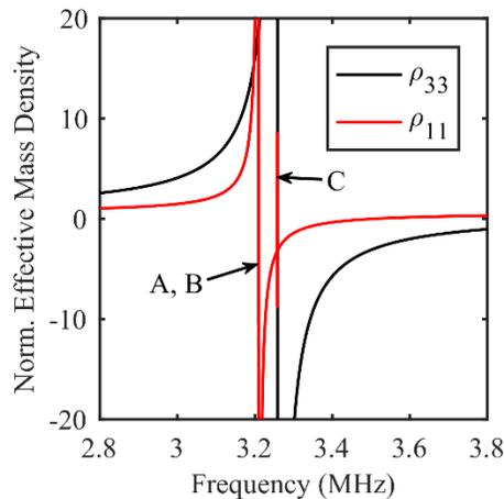
Figure 1.2: Effective mass density matrix components  $\rho_{11}$  (red) and  $\rho_{33}$  (black) normalized to the mass density of steel as a function of the excitation frequency.
