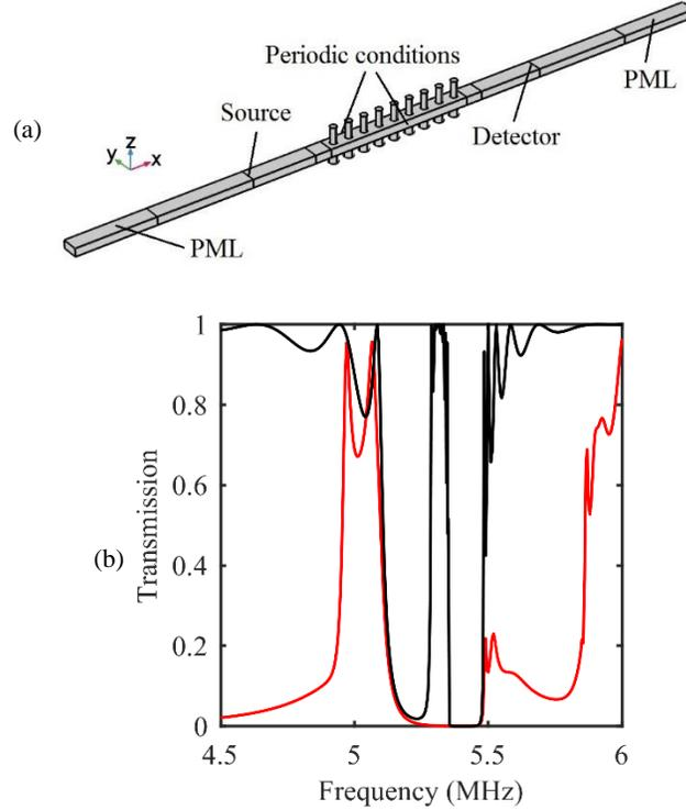
Figure 1.9: (a) Finite element model to investigate the transmission of an incident  $SH_0$  and  $A_0$  Lamb waves along  $\Gamma X$  direction. (b) Transmission spectra of incident  $SH_0$  (black) and  $A_0$  Lamb waves (red) propagating across the supercell in (a).
