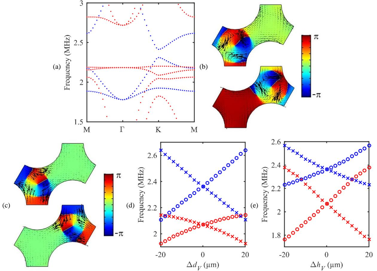
Figure 2.15: Band structure of the perturbed PPnC with the diameter perturbation  $\Delta d_V = 4\mu\text{m}$ . Energy flux (black arrows) and phase distribution of the out-of-plane displacement at the lower (bottom panel) and higher (top panel) bounding of the lifted Dirac cone at the valley K for the (b) symmetric and (c) antisymmetric band structure subcomponents. Evolutions of the valley pseudospin states against the (d) diameter and (e) height perturbation at the valley K.
