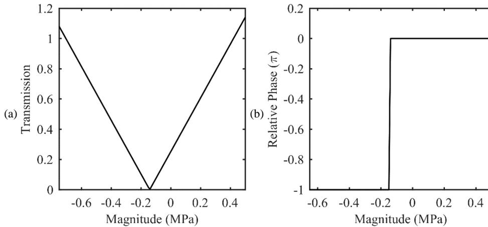
Figure 3.12: (a) Transmission spectrum against the magnitude of the external pressure when the phase difference is fixed at  $1.72\pi$ . (b) Relative phase between the transmitted amplitude  $A_{transTotal}$  and  $A_{transIn}$ .
