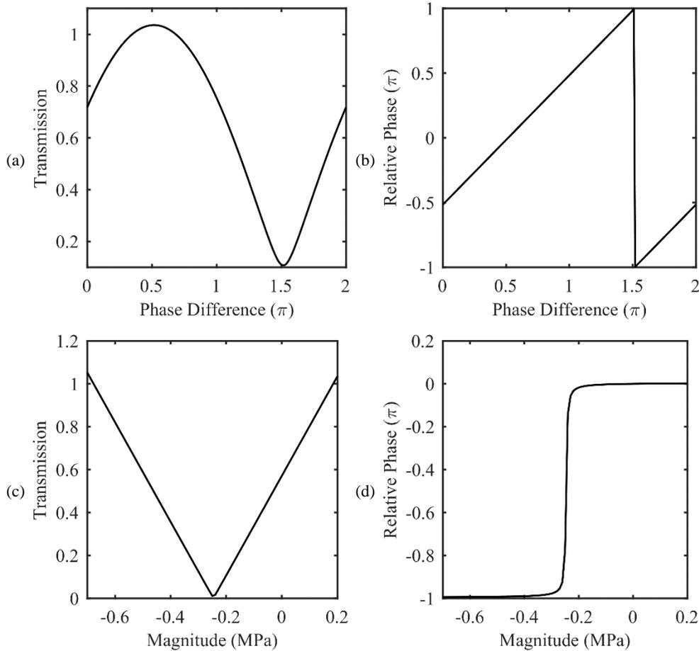
Figure 3.14: (a) Transmission coefficient against the phase difference of the external traction when the magnitude is assumed to be 0.2MPa. (b) Relative phase between the transmitted amplitude  $A_{transEx}$  and  $A_{transIn}$ . (c) Transmission coefficient against the magnitude when the phase difference is fixed at  $0.52\pi$ . (d) Relative phase between the transmitted amplitude  $A_{transTotal}$  and  $A_{transIn}$ .
