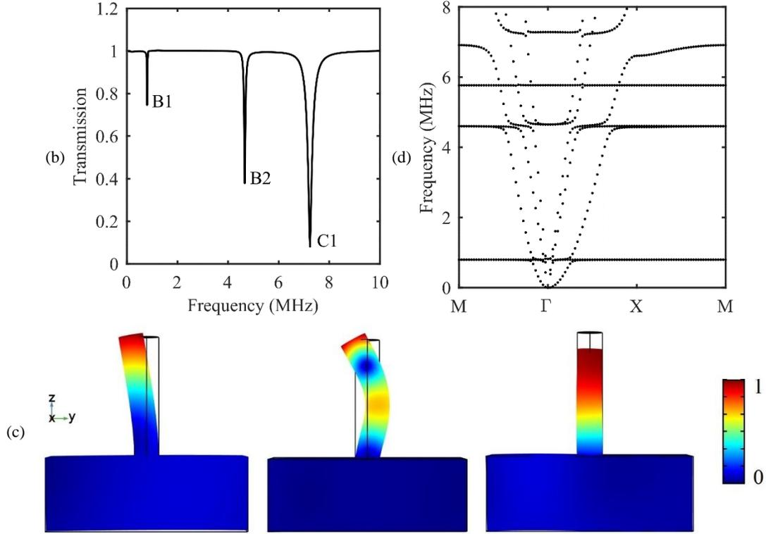
Figure 3.1: (a) Proposed finite element model and (b) transmission spectrum of an incident  $A_0$  Lamb wave propagating through the line of pillars. (c) Normalized displacement fields of the line of pillars at the three transmission dips. (d) Band structure of a square lattice pillared metamaterial built by the same pillar shown in (a) with lattice constant set to be  $200\mu\text{m}$ .
