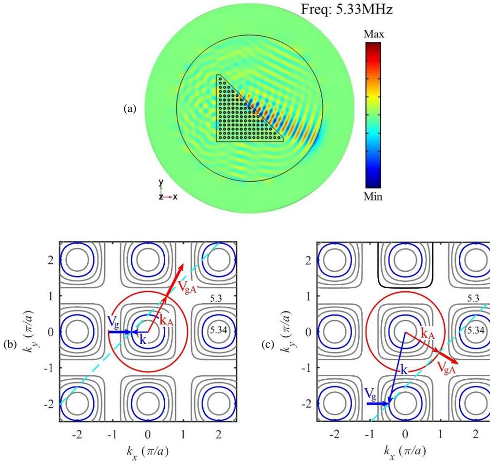
Figure 1.18: (a) Plot of the out-of-plane displacement on the top surface of the plate under the excitation of an incident  $SH_0$  mode at frequency 5.33MHz. EFCs analysis of (b) the negative and (c) the positive refraction at the outlet interface. The transmitted wave is assumed to be  $A_0$  mode only.
