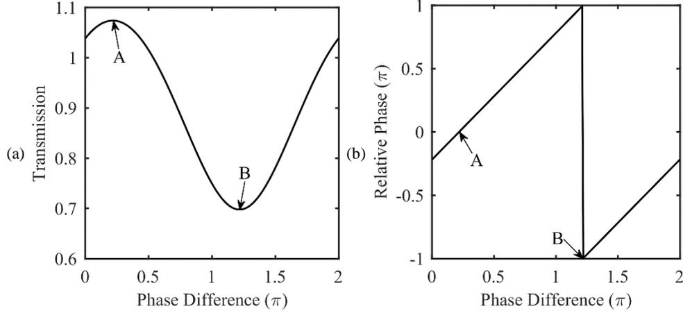
Figure 3.7: (a) Transmission coefficient against the phase difference of the external traction force when the magnitude is assumed to be 0.1MPa. (b) Relative phase between the transmitted amplitude  $A_{transEx}$  and  $A_{transIn}$ .
