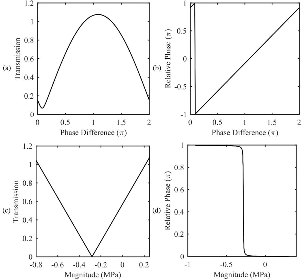
Figure 3.15: (a) Transmission coefficient against the phase difference of the external pressure when the magnitude is assumed to be 0.25MPa. (b) Relative phase between the transmitted amplitude  $A_{transEx}$  and  $A_{transIn}$ . (c) Transmission coefficient against the magnitude when the phase difference is fixed at  $1.08\pi$ . (d) Relative phase between the transmitted amplitude  $A_{transTotal}$  and  $A_{transIn}$ .
