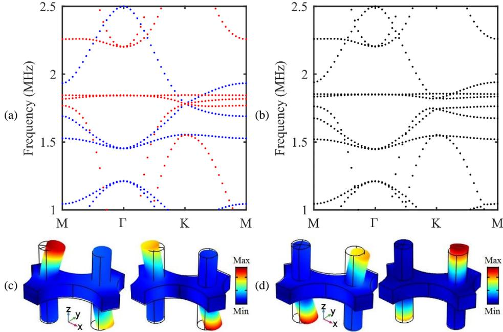
Figure 2.28: (a) Occurrence of the double Dirac cone. (b) Lifting of the double Dirac cone after imposing the height perturbation  $\Delta h_s = 3\mu\text{m}$ . Eigenmodes at the (c) lower and (d) higher Dirac cones respectively.
