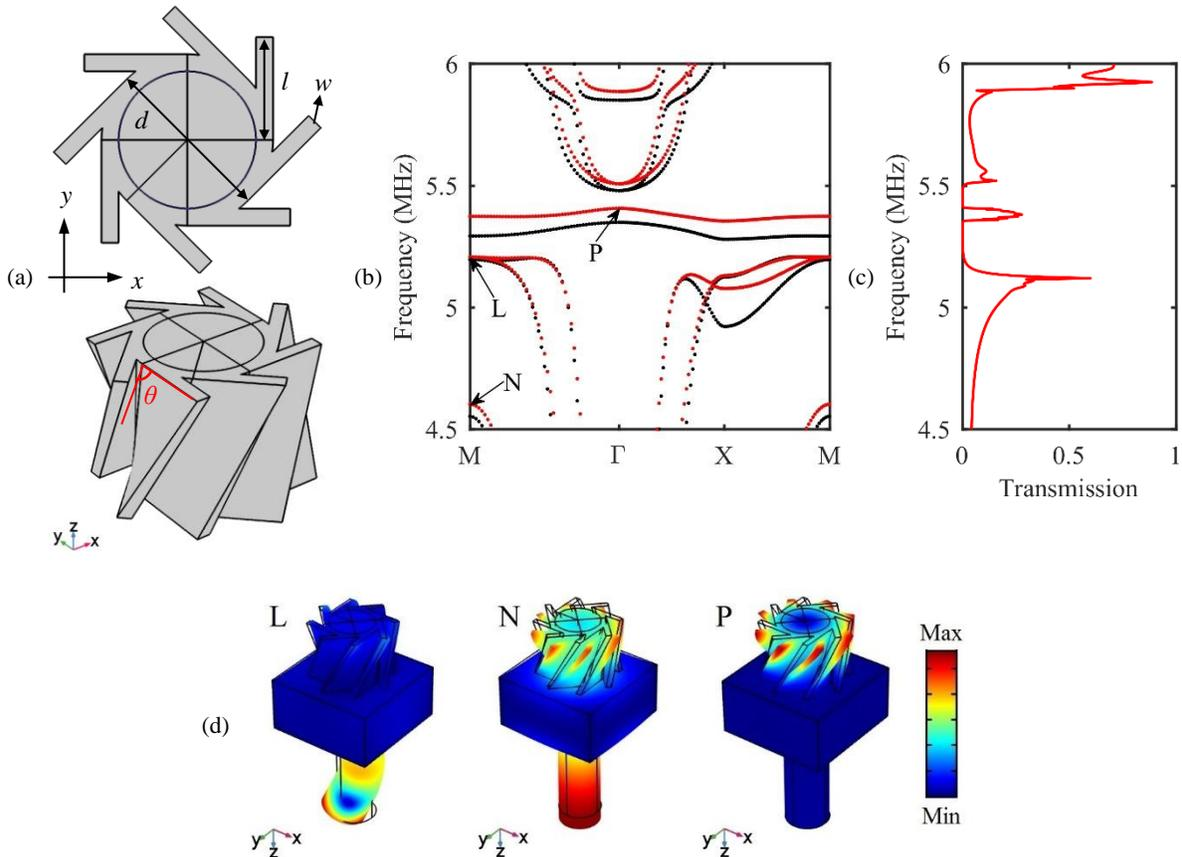
Figure 1.11: (a) Representative profile of the chiral pillar B. (b) Band structure of CDPM (red dotted lines) and ADPM (black dotted lines). (c) Transmission spectrum of an incident  $A_0$  mode propagating across the supercell shown in figure 1.9(a) with the chiral pillar B instead. (d) Eigenmodes of the unit cell at points indicated in (b).
