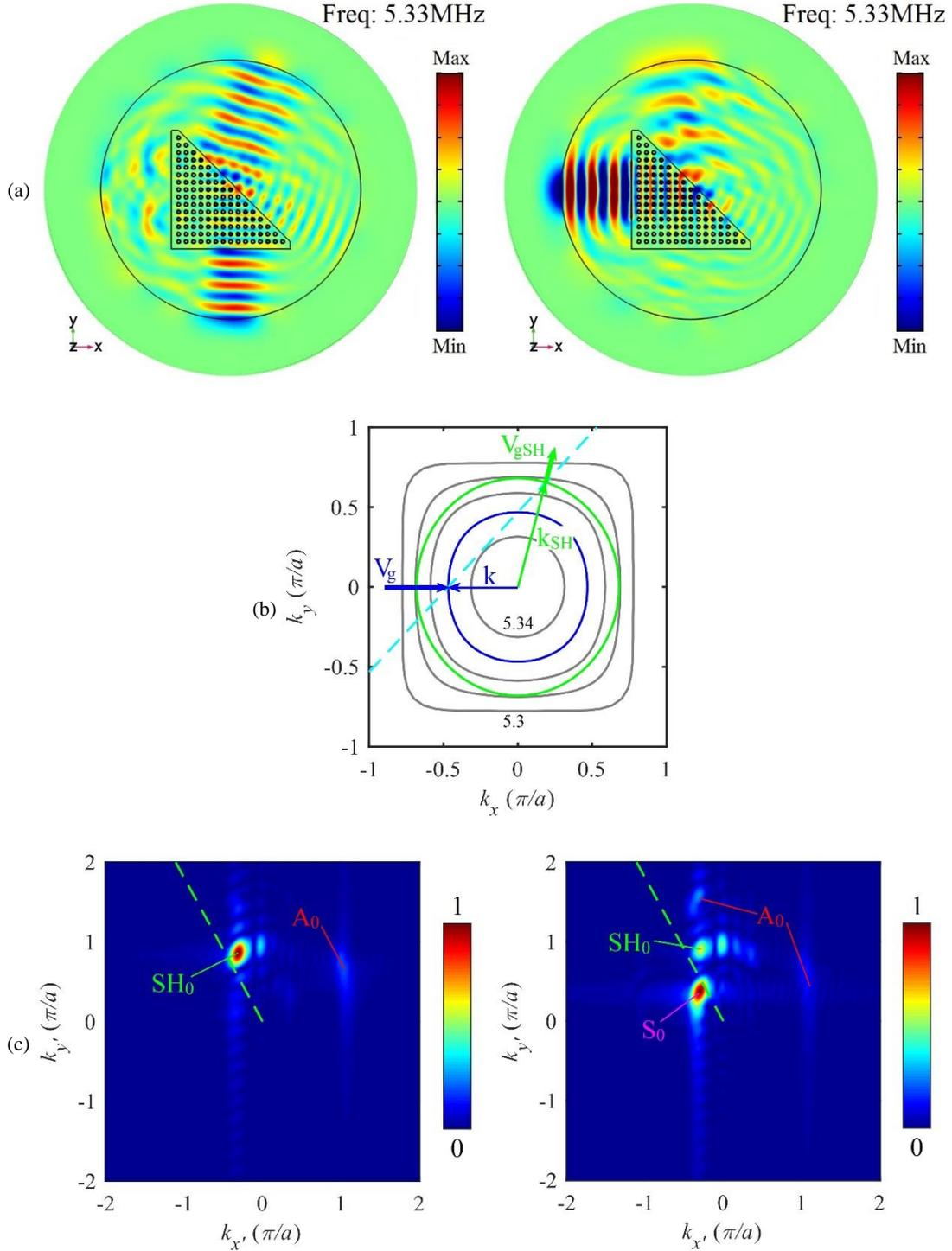
Figure 1.22: (a) Plots of the in-plane displacement components  $u_x$  (left panel) and  $u_y$  (right panel) on the top surface of the plate under the excitation of an incident  $SH_0$  mode at frequency 5.33MHz. (b) EFCs analysis of the refraction
