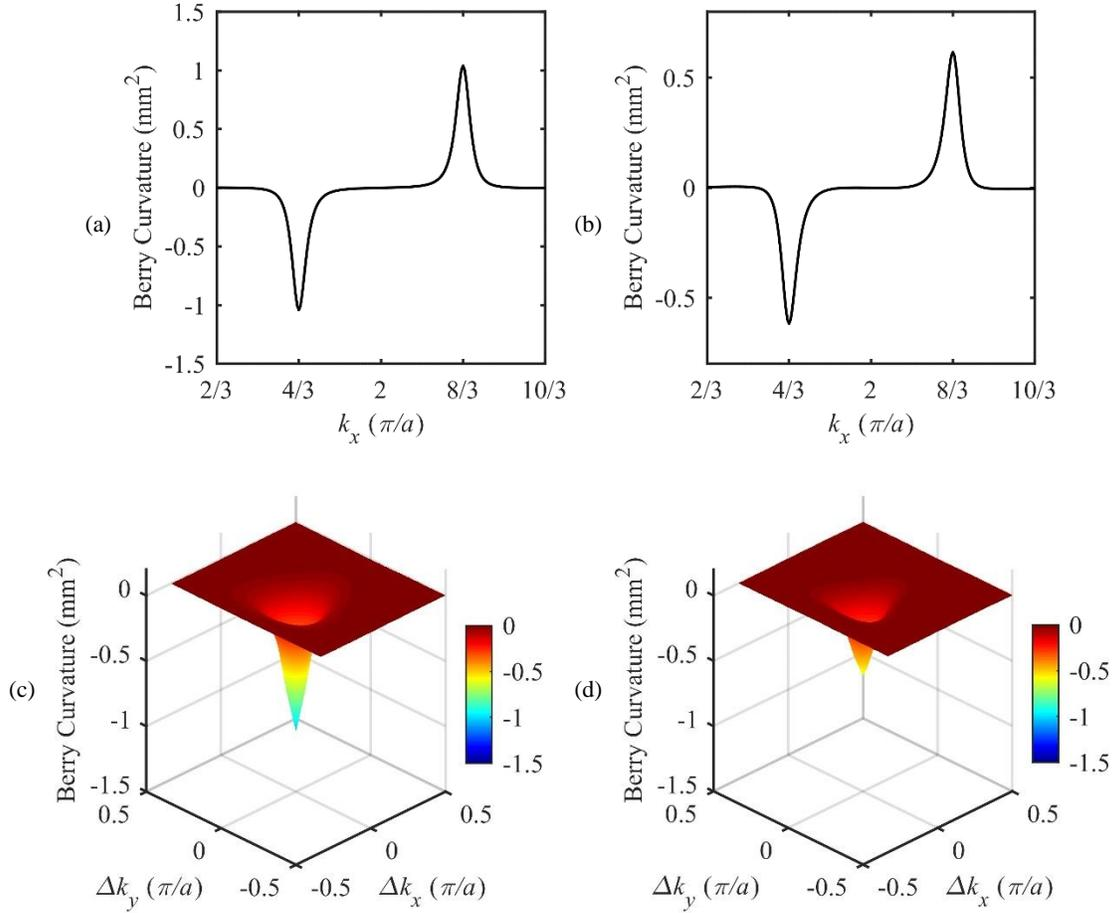
Figure 2.16: Numerical results of the Berry curvature of the lower bounding of the lifted Dirac cones: at the wave vectors varying from  $k_x = 2\pi/3a$  to  $k_x = 10\pi/3a$  and  $k_y = 0$  for the (a) antisymmetric and (b) symmetric band structure subcomponents and in the vicinity of the valley K for the (c) antisymmetric and (d) symmetric band structure subcomponents.
