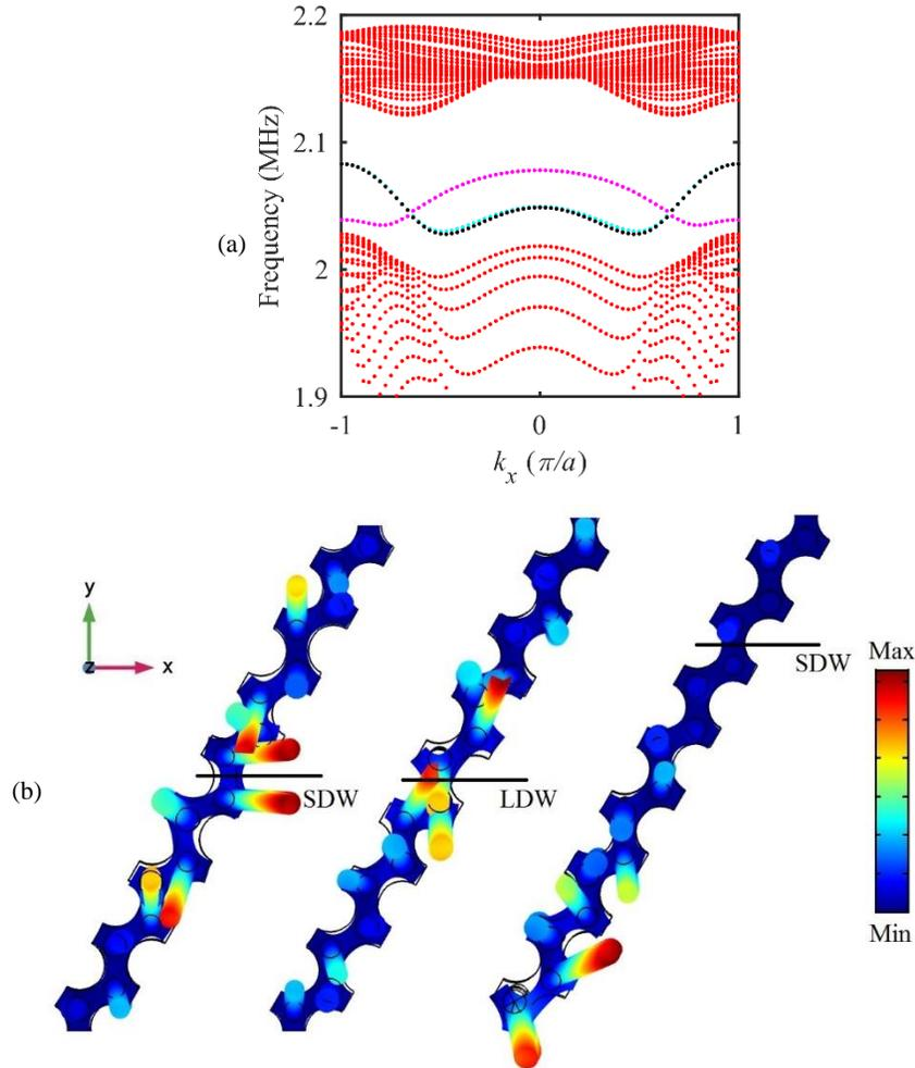
Figure 2.21: (a) Symmetric dispersion curves of the ribbon supercell. (b) Eigenmode of the edge states (magenta and cyan branches) and locally resonant mode (black branch) at the wave vector  $k_x = 0.5\pi/a$ .
