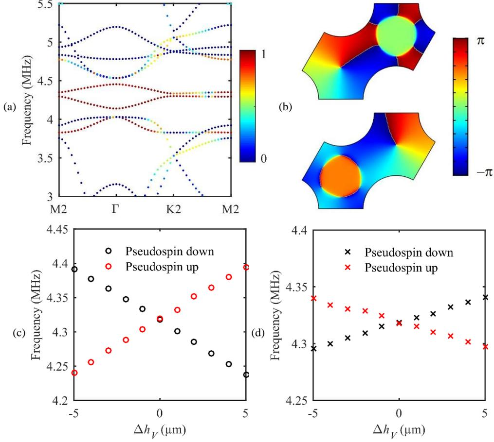
Figure 2.6: (a) Band structure of the perturbed PPnC with the height perturbation  $\Delta h_V = 1 \mu\text{m}$ . (b) Phase distribution of the out-of-plane displacement on the top surface of the plate at the higher (top panel) and lower (bottom panel) bounding of the lifted Dirac cone. Evolution of the pseudospin up and down states at the valley K2 against the height perturbation  $\Delta h_V$  in the (c) lower (red and black circles) and (d) upper (red and black crosses) pillars.
