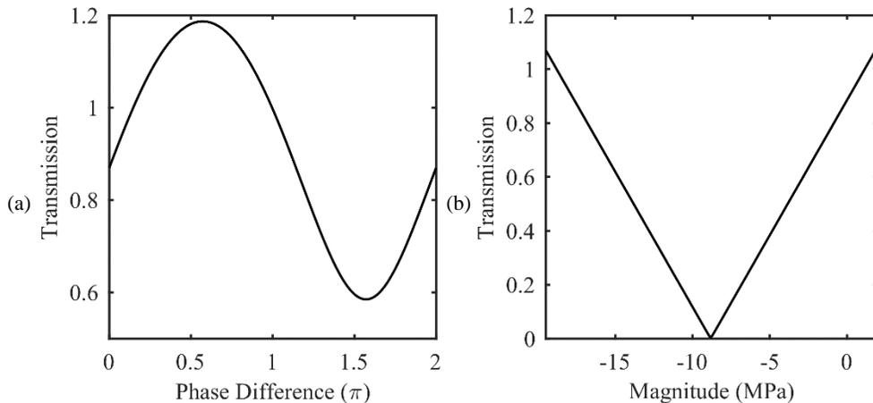
Figure 3.9: (a) Transmission coefficient against the phase difference of the external pressure when the magnitude is assumed to be 3MPa. (b) Transmission coefficient against the magnitude of the external pressure when the phase difference is chosen to be  $0.57\pi$ .
