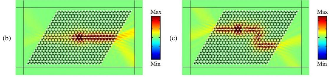
Figure 2.12: (a) Dispersion curves of the proposed three-layers ribbon supercell with the increased height perturbation  $\Delta h_V = 2\mu\text{m}$ . Plots the magnitude of the out-of-plane displacement on the top surface of the plate under the excitation of the  $K_2'$ -polarized  $SH_0$  wave at frequency  $4.304\text{MHz}$  in the (b) straight and (c) Z-shape wave guides.
