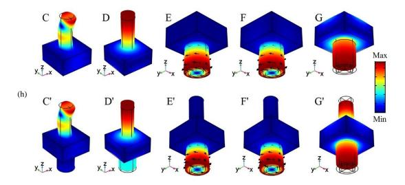
Figure 1.6: Elementary unit cells of (a) SPM-A, (b) SPM-B and (c) DPM and corresponding band structures of (d) SPM-A, (f) SPM-B and (g) ADPM. (e) Effective mass density matrix components  $\rho_{11}$  (red solid line) and  $\rho_{33}$  (black solid line) normalized to the mass density of steel as a function of the excitation frequency. (h) Eigenmodes of the unit cell at points labelled in panels (d), (f) and (g).
