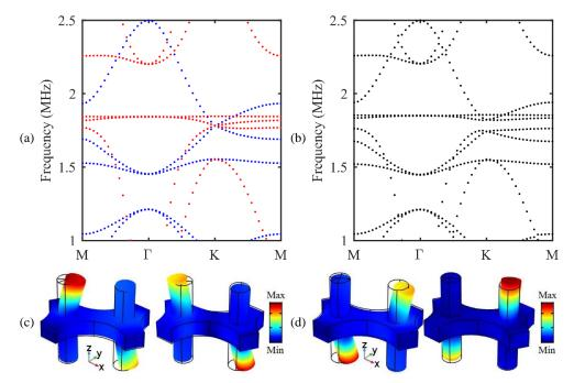
Figure 2.28: (a) Occurrence of the double Dirac cone. (b) Lifting of the double Dirac cone after imposing the height perturbation  $\Delta h_S = 3\mu m$ . Eigenmodes at the (c) lower and (d) higher Dirac cones respectively.
