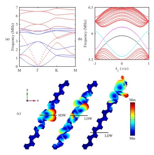
Figure 2.25: (a) Band structure of the perturbed PPnC with the diameter perturbation  $\Delta d_V = 10 \mu m$ . (b) Symmetric dispersion curves of the ribbon supercell. (c) Eigenmodes of the edge states (magenta and cyan branches) and the locally resonant mode (black branch) at the wave vector  $k_x = 0.5\pi/a$ .
