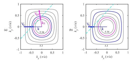
Figure 1.20: EFCs analysis of the refraction at the outlet interface at frequencies (a) 5.33MHz and (b) 5.31MHz. The transmitted wave is assumed to be S<sub>0</sub> mode only.
