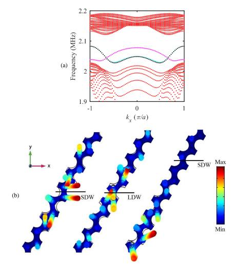
Figure 2.21: (a) Symmetric dispersion curves of the ribbon supercell. (b) Eigenmode of the edge states (magenta and cyan branches) and locally resonant mode (black branch) at the wave vector  $k_x = 0.5\pi/a$ .
