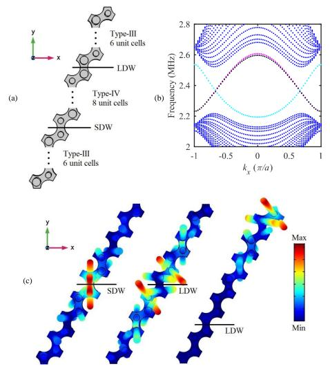
Figure 2.18: (a) Schematic of the proposed three-layers ribbon supercell constructed by sandwiching eight unit cells of type-IV PPnC in between two sets of six unit cells of type-III PPnC. (b) Antisymmetric dispersion curves of the ribbon supercell. (c) Eigenmode of the edge states (magenta and cyan branches) and locally resonant mode (black branch) at the wave vector  $k_x = 0.5\pi/a$ .
