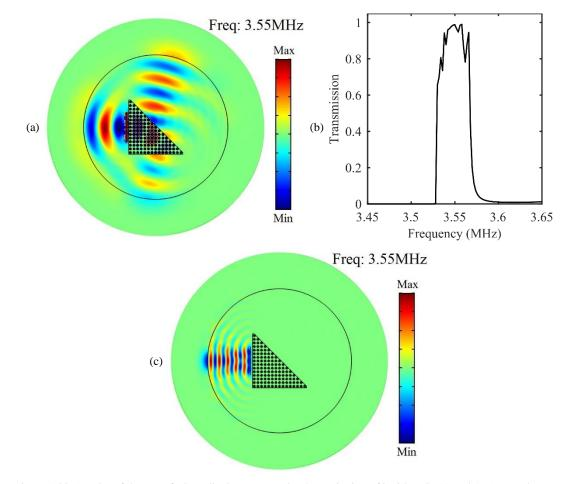
Figure 1.23: (a) Plot of the out-of-plane displacement under the excitation of incident  $S_0$  (a) and  $A_0$  (c) Lamb waves at frequency 3.55MHz. (b) Transmission coefficient of  $S_0$  Lamb wave impinging a phononic crystal built by eleven unit cells along the *x*-axis and infinite along the *y*-axis at normal incidence.
