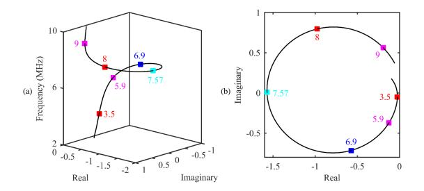
Figure 3.4: (a) Evolution of the complex amplitude of the reemitted Lamb wave against the frequency. (b) Top view (see from the positive *z*-axis) of the curve displayed in (a). The bending resonance B2 and the compressional resonance C1 are superimposed.
