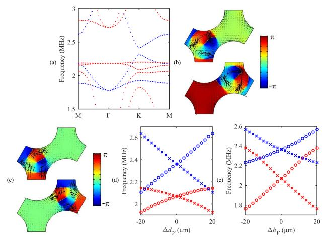
Figure 2.15: Band structure of the perturbed PPnC with the diameter perturbation  $\Delta dv = 4\mu$ m. Energy flux (black arrows) and phase distribution of the out-of-plane displacement at the lower (bottom panel) and higher (top panel) bounding of the lifted Dirac cone at the valley K for the (b) symmetric and (c) antisymmetric band structure subcomponents. Evolutions of the valley pseudospin states against the (d) diameter and (e) height perturbation at the valley K.
