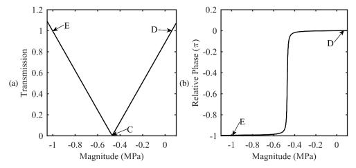
Figure 3.8: (a) Transmission coefficient against the magnitude of the external traction force when the phase difference is fixed at  $0.22\pi$ . (b) Relative phase between the transmitted amplitude  $A_{transTotal}$  and  $A_{transIn}$ .
