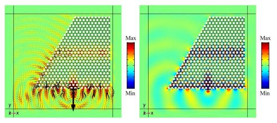
Figure 2.23: Plots of the magnitude of the in-plane displacement (left panel) and the out-of-plane displacement (right panel) on the top surface of the plate under the excitation of a *z*-polarized point source at the bottom interface.
