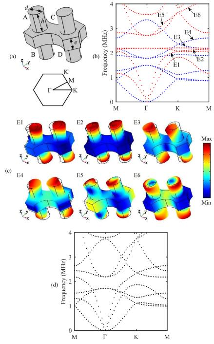
Figure 2.13: (a) Elementary unit cell of the proposed symmetric double-sided PPnC and (b) the corresponding band structure. (c) Eigenmodes at points labelled from E1 to E6 in (b). (d) Band structure of the single-sided PPnC by removing all the pillars on one side of the plate.
