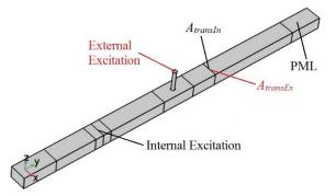
Figure 3.5: Schematic of the transmission control by introducing external sources applied on the line of pillars.
