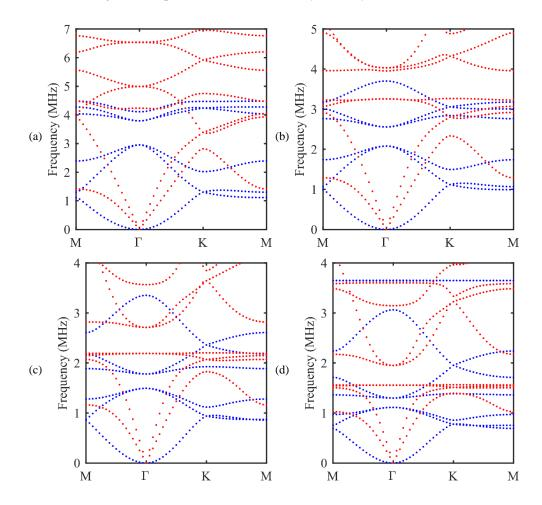
Figure 2.14: Band structures of the symmetric double-sided PPnCs with the height of the pillars set to be (a)  $80\mu$ m, (b)  $120\mu$ m, (c)  $160\mu$ m and (d)  $200\mu$ m respectively.
