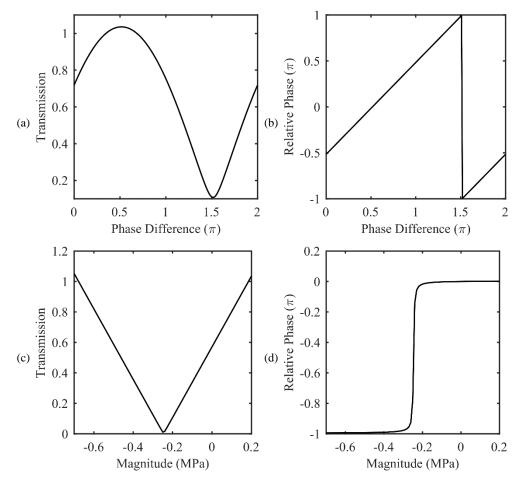
Figure 3.14: (a) Transmission coefficient against the phase difference of the external traction when the magnitude is assumed to be 0.2MPa. (b) Relative phase between the transmitted amplitude  $A_{transEx}$  and  $A_{transIn}$ . (c) Transmission coefficient against the magnitude when the phase difference is fixed at 0.52 $\pi$ . (d) Relative phase between the transmitted amplitude  $A_{transTotal}$  and  $A_{transIn}$ .
