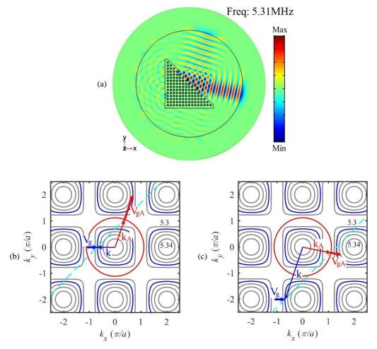
Figure 1.19: (a) Plot of the out-of-plane displacement on the top surface of the plate under the excitation of an incident  $SH_0$  mode at frequency 5.31MHz. EFCs analysis of (b) the negative and (c) the positive refraction at the outlet interface. The transmitted wave is assumed to be  $A_0$  mode only.
