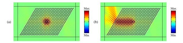
Figure 2.10: Plots of the magnitude of the out-of-plane displacement on the top surface of the plate under the excitation of the K2'-polarized (a) SH<sub>0</sub> and (b) A<sub>0</sub> Lamb waves at frequency 4.325MHz. The straight wave guide is constructed by inverting the position of type-I and type-II PPnCs as illustrated in figure 2.9(a).
