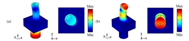
Figure 1.7: Eigenmodes of ADPM unit cell at the wave vectors in the middle of  $\Gamma$ M (a) and  $\Gamma$ X (b) boundaries. Their top views are shown in the corresponding right panels.
