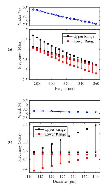
Figure 1.15: Edges of the band gap (lower panel) and relative width of the double-negative branch (upper panel) against (a) the height and (b) the diameter of the pillars. The black (red) solid lines stand for the upper (lower) part of the band gap. In both panels the blue curve is the relative width of the band where the doubly negative property occurs.
