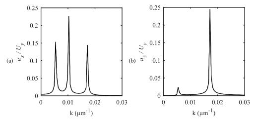
Figure 1.10: Fourier spectrum of the displacement components along the x-axis (a) and the z-axis (b) of the transmitted wave at the frequencies inside the double-negative branch.
