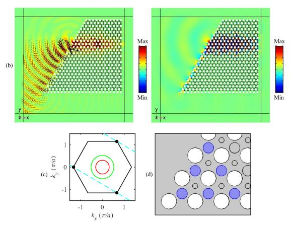
Figure 2.22: Plots of the magnitude of the in-plane displacement (left panel) and the out-of-plane displacement (right panel) on the top surface of the plate under the excitation of the left-going K'-polarized edge state at frequency 2.042MHz that was launched in the middle (a) with and (b) without the resonant pillars. (c) EFCs analysis of the refracted pattern at the left zigzag termination. (d) Zoomed view of the left bottom corner in (a) and (b).
