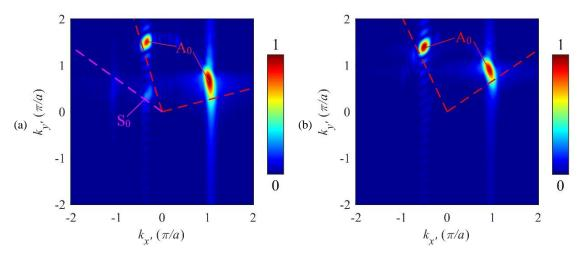
Figure 1.21: Two-dimensional Fourier transform of the out-of-plane displacement in the red rectangle dashed area shown in figure 1.17(a) at frequencies (a) 5.33MHz and (b) 5.31MHz. The red and magenta dashed lines represent their refracted angles calculated from the EFCs analysis.
