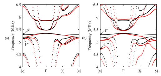
Figure 1.8: Band structures (red dotted lines) after introducing perforated holes with the diameter  $60\mu m$  (a) and  $100\mu m$  (b) at the four corners of the square lattice unit cell of the proposed ADPM. The band structure of ADPM without perforated holes is shown as the black dotted lines for reference.
