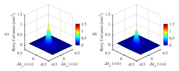
Figure 2.17: Numerical results of the Berry curvature of the higher bounding of the lifted Dirac cones: at the wave vectors varying from  $k_x = 2\pi/3a$  to  $k_x = 10\pi/3a$  and  $k_y = 0$  for the (a) antisymmetric and (b) symmetric band structure subcomponents and in the vicinity of the valley K for the (c) antisymmetric and (d) symmetric band structure subcomponents.
