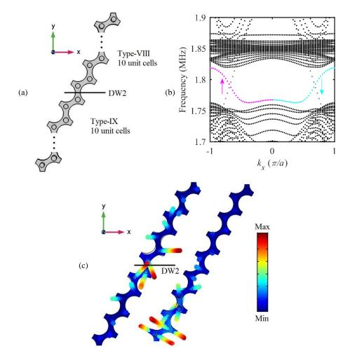
Figure 2.31: (a) Schematic of the proposed two-layers ribbon supercell constructed by juxtaposing ten unit cells of type-VIII PPnC and ten unit cells of type-IX PPnC vertically. (b) Dispersion curves of the ribbon supercell. (c) Eigenmodes of the grey and cyan branches at the wave vector  $k_x = 2\pi/3a$ .
