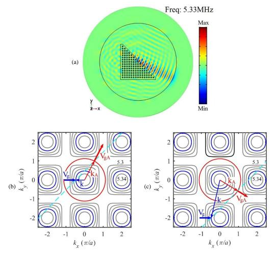
Figure 1.18: (a) Plot of the out-of-plane displacement on the top surface of the plate under the excitation of an incident  $SH_0$  mode at frequency 5.33MHz. EFCs analysis of (b) the negative and (c) the positive refraction at the outlet interface. The transmitted wave is assumed to be  $A_0$  mode only.
