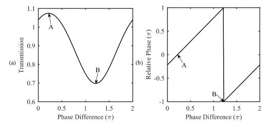
Figure 3.7: (a) Transmission coefficient against the phase difference of the external traction force when the magnitude is assumed to be 0.1MPa. (b) Relative phase between the transmitted amplitude  $A_{transEx}$  and  $A_{transIn}$ .
