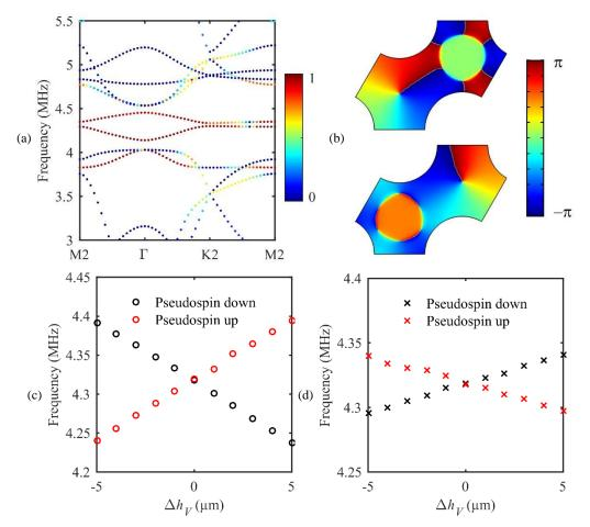
Figure 2.6: (a) Band structure of the perturbed PPnC with the height perturbation  $\Delta h_V = 1 \mu m$ . (b) Phase distribution of the out-of-plane displacement on the top surface of the plate at the higher (top panel) and lower (bottom panel) bounding of the lifted Dirac cone. Evolution of the pseudospin up and down states at the valley K2 against the height perturbation  $\Delta h_V$  in the (c) lower (red and black circles) and (d) upper (red and black crosses) pillars.
