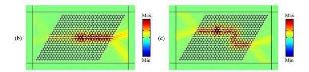
Figure 2.12: (a) Dispersion curves of the proposed three-layers ribbon supercell with the increased height perturbation  $\Delta h_V = 2\mu m$ . Plots the magnitude of the out-of-plane displacement on the top surface of the plate under the excitation of the K2'-polarized SH<sub>0</sub> wave at frequency 4.304MHz in the (b) straight and (c) Z-shape wave guides.
