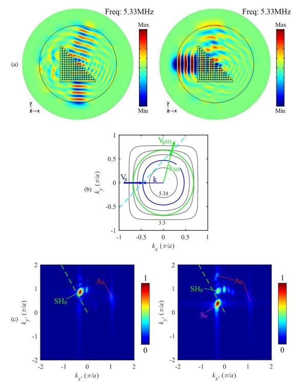
Figure 1.22: (a) Plots of the in-plane displacement components  $u_x$  (left panel) and  $u_y$  (right panel) on the top surface of the plate under the excitation of an incident SH<sub>0</sub> mode at frequency 5.33MHz. (b) EFCs analysis of the refraction
