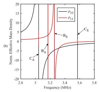
Figure 1.13: (a) Eigenmodes of the unit cell at the four representative resonance frequencies upon excitation  $(Ae^{i\alpha t}, 0, 0)$ . (b) Effective mass density matrix components  $\rho_{11}$  (red) and  $\rho_{33}$  (black) normalized to the mass density of steel as a function of the excitation frequency.
