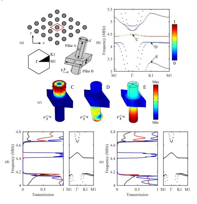
Figure 2.4: (a) Schematic of the proposed asymmetric double-sided PPnC arranged in the triangular lattice and (b) the corresponding band structure. (c) Eigenmodes at points C, D and E labelled in (b) and the black arrows represent the elastic deformation vectors. Transmission spectra of incident  $A_0$  (black),  $S_0$  (red) and  $SH_0$  (blue) Lambs wave propagating along (d)  $\Gamma K1$  and (e)  $\Gamma M1$  directions.
