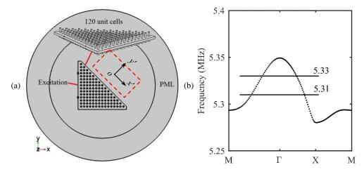
Figure 1.17: (a) Finite element model adopted to investigate the refraction at the outlet interface between a prismshaped supercell and the surrounding plate. (b) Relative positions of the excitation frequencies inside the doublenegative branch.
