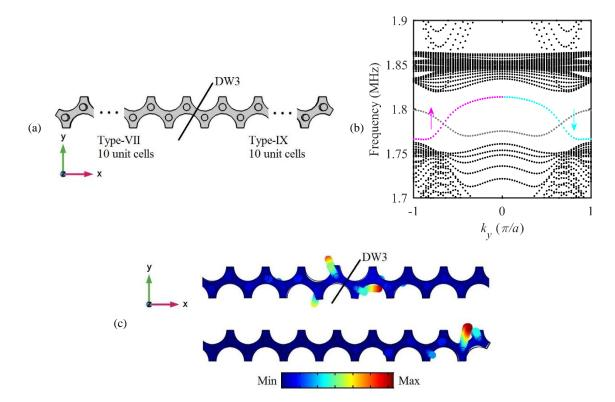
Figure 2.32: (a) Schematic of the proposed two-layers ribbon supercell constructed by juxtaposing ten unit cells of type-VII PPnC and ten unit cells of type-IX PPnC horizontally. (b) Dispersion curves of the ribbon supercell. (c) Eigenmodes of the cyan (top panel) and grey (bottom panel) branches at  $k_x = 2\pi/3a$ .
