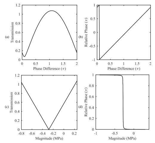
Figure 3.15: (a) Transmission coefficient against the phase difference of the external pressure when the magnitude is assumed to be 0.25MPa. (b) Relative phase between the transmitted amplitude  $A_{transEx}$  and  $A_{transIn}$ . (c) Transmission coefficient against the magnitude when the phase difference is fixed at  $1.08\pi$ . (d) Relative phase between the transmitted amplitude  $A_{transTotal}$  and  $A_{transIn}$ .
