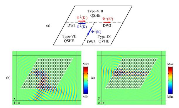
Figure 2.33: (a) Schematic of the T-shaped wave guide and the valley based splitting of the pseudospin down edge states. Plots of the out-of-plane displacement on the top surface of the plate while the pseudospin-protected edge states are locked to the valley (b) K and (c) K' respectively.
