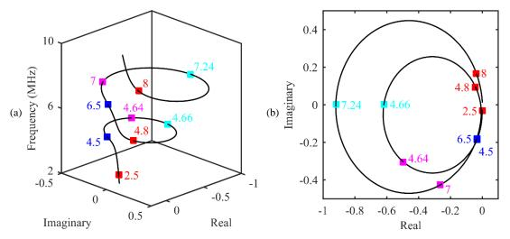
Figure 3.3: (a) Evolution of the complex amplitude of the reemitted Lamb wave against the frequency. (b) Top view (see form the positive *z*-axis) of the curve displayed in (a). The bending resonance B2 and the compressional resonance C1 are separated.
