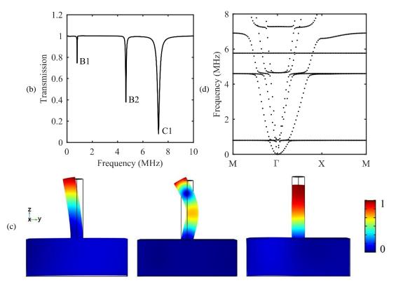
Figure 3.1: (a) Proposed finite element model and (b) transmission spectrum of an incident  $A_0$  Lamb wave propagating through the line of pillars. (c) Normalized displacement fields of the line of pillars at the three transmission dips. (d) Band structure of a square lattice pillared metamaterial built by the same pillar shown in (a) with lattice constant set to be 200 $\mu$ m.
