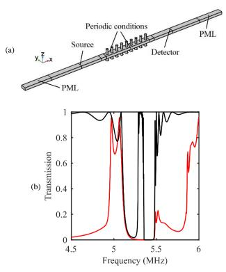
Figure 1.9: (a) Finite element model to investigate the transmission of an incident SH<sub>0</sub> and A<sub>0</sub> Lamb waves along  $\Gamma$ X direction. (b) Transmission spectra of incident SH<sub>0</sub> (black) and A<sub>0</sub> Lamb waves (red) propagating across the supercell in (a).
