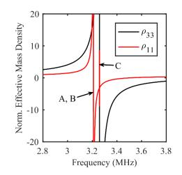
Figure 1.2: Effective mass density matrix components  $\rho_{11}$  (red) and  $\rho_{33}$  (black) normalized to the mass density of steel as a function of the excitation frequency.
