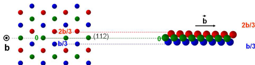
Figure 1.12 – Illustration of the origin of twinning / anti-twinning directions for \langle 111 \rangle screw dislocations: (left) Atomic structure of BCC as seen from a [111] direction. Along this direction, the BCC structure can be seen as the superposition of three atom strings as highlighted by three colors (green, blue, red), shifted by b/3 along the [111] direction. (right) Atomic structure as seen from the side. The atomic arrangement is not symmetric \{112\} planes (after Chaussidon 2007) [32].
