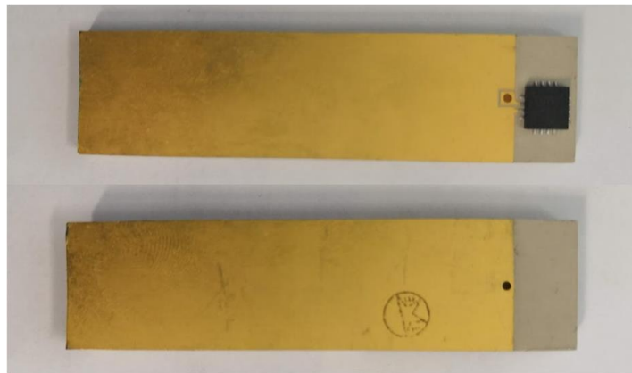
Figure 3.18: Fabricated \lambda/2 UHF RFID sensor tag
