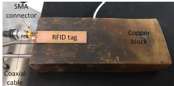
Figure 6.10: Measurement setup of the RFID antenna tag
