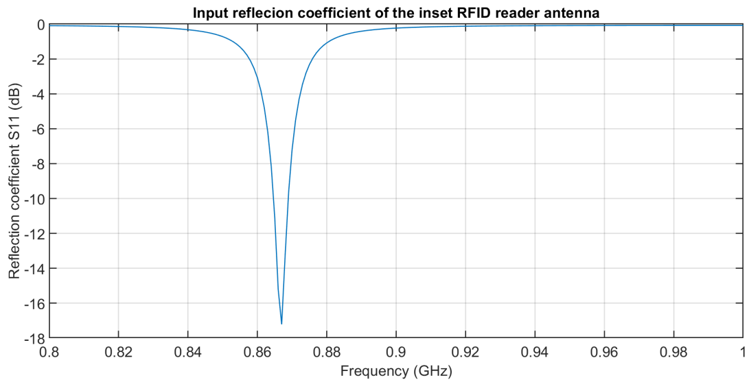
Figure 4.30: Input reflection coefficient of inset RFID reader antenna
