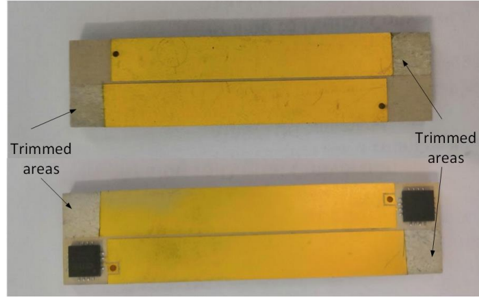
Figure 4.10: Fabricated \lambda/2 twin RFID tag with the trimmed areas marked
