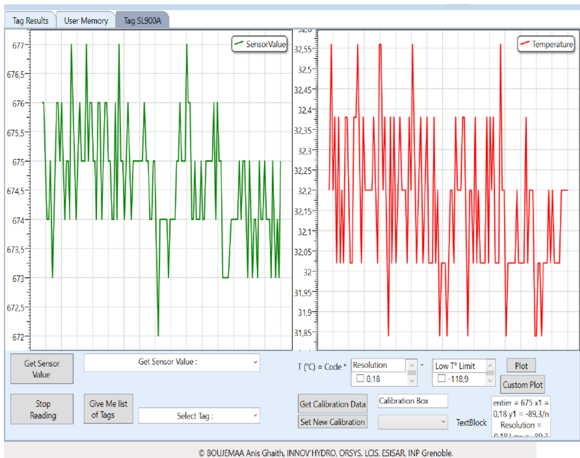
Figure 7.18: Developed interface for acquiring the output value of the integrated temperature sensor of the SL900A RFID chip
