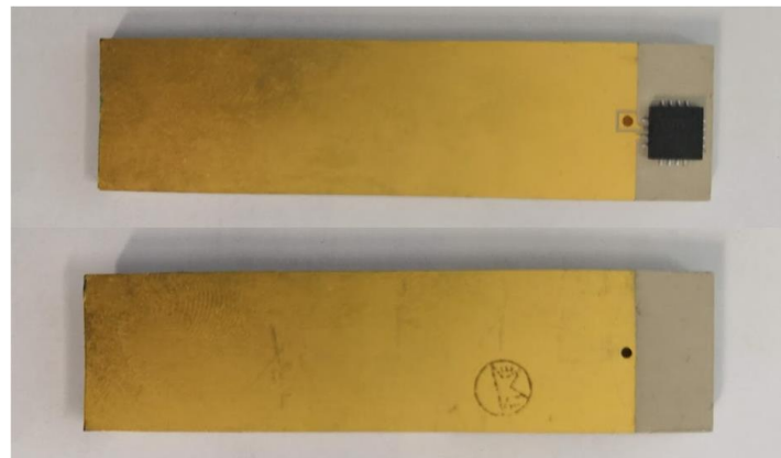
Figure 3.18: Fabricated \lambda/2 UHF RFID sensor tag
