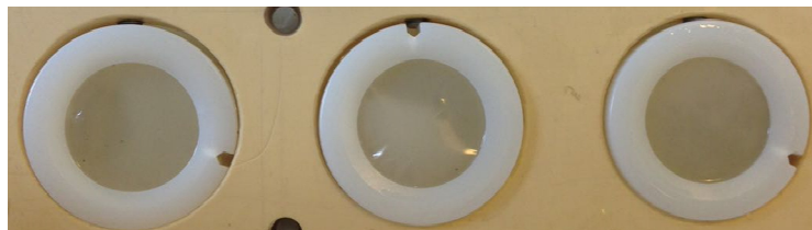
Zr-DGT samplers (72h deployment time)
