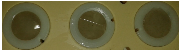
Zr-DGT samplers (216h deployment time)
