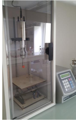
Figure IV.155 – Sonicateur Vibracell 75041 (Fisher Bioblock Scientific)
