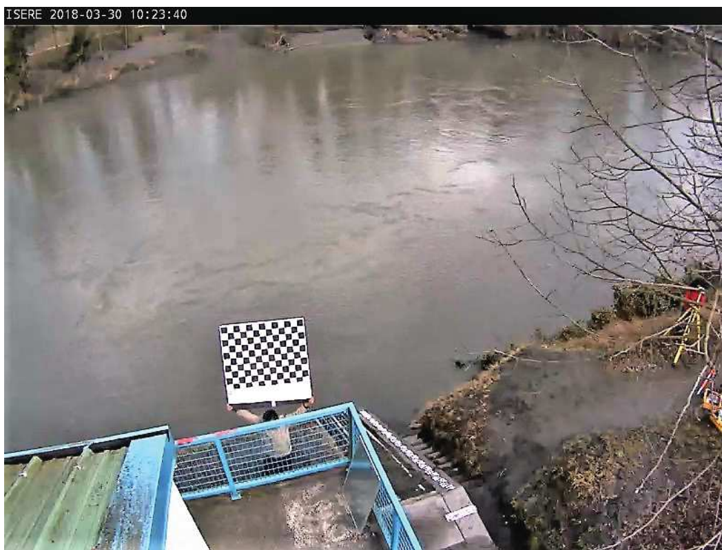
Figure II.9: Using a chessboard on the field to correct the image fisheye distortion on video frames.
