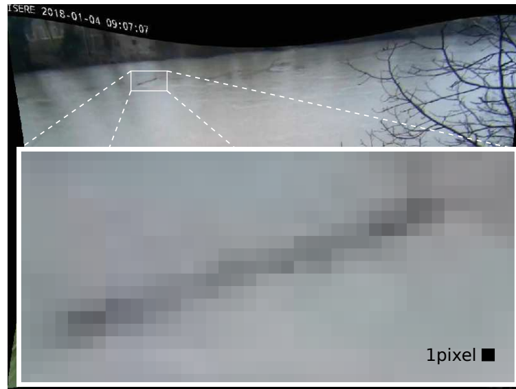
Figure II.16: Uncertainty on detection of the wood length due to the blurry area at the borders of the object.
