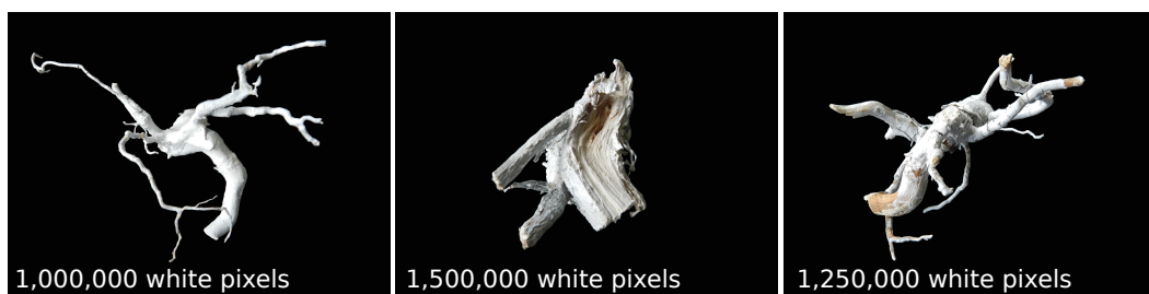
Figure III.12: Measuring frontal area of natural logs. Image size is 12Mpixel.
