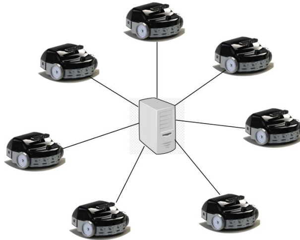
Figure 1.2: Centralized control scheme
