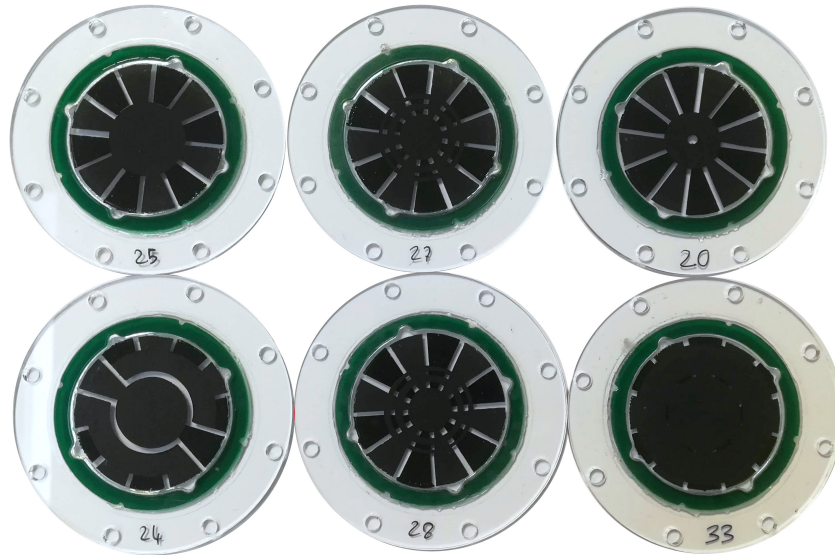
Fig. 3.9. Samples of dielectric elastomer membrane coated with patterned electrodes, with different electrode shapes.
