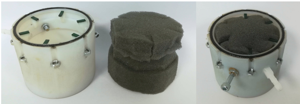
Fig. 5.16. DE loudspeaker cavity with foam, for damping both the membrane modes and the acoustic cavity modes.
