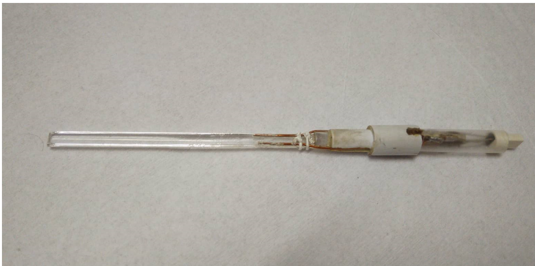
Figure 3.4 – Homemade sample holder adapted for electric measurements.
