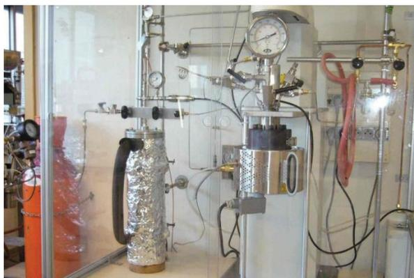
**Figure S1. Autoclave used for ethylene polymerization.**
