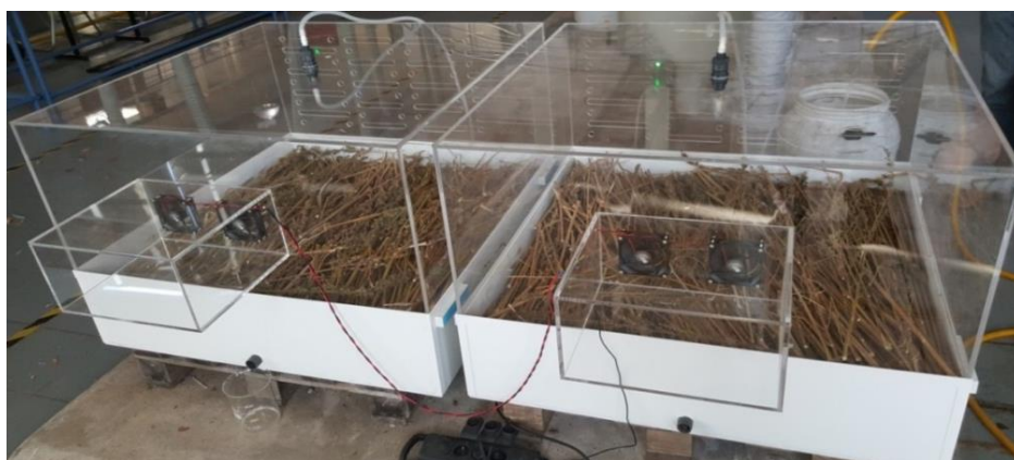
Figure V.3. Lab-scale pilot units used for a controlled and accelerated retting
