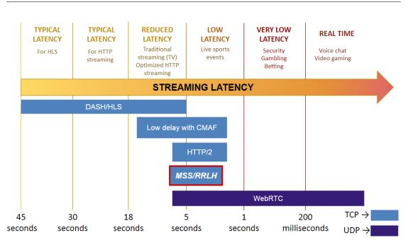
Figure 6.18: Latency range of MSS/RRLH compared with SotA solutions
