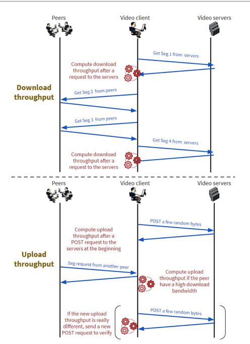
Figure 5.11: Overview of the upload and download throughput estimation in PMS+
