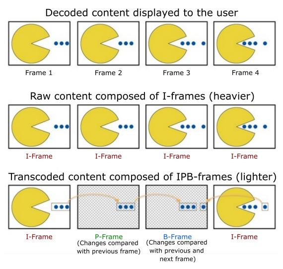
Figure 2.1: IPB frames in a transcoded video
