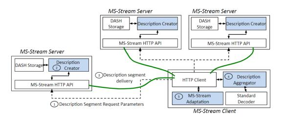
Figure 6.5: MS-Stream logical architecture
