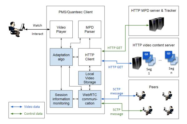
Figure 5.2: Peer's software architecture
