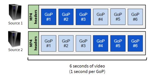
Figure 3.3: Two substreams with GoP in high and low quality from two different sources
