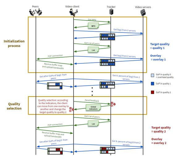
Figure 5.3: Sequence diagram of data exchange in PMS
