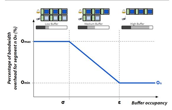
Figure 6.11: Relation between overhead selection and buffer occupancy level
