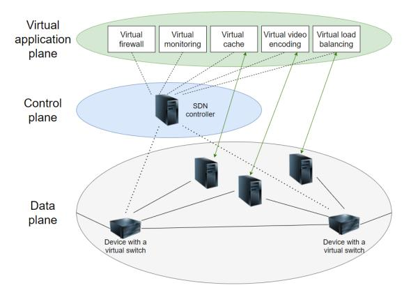
Figure 4.4: Simplified architecture of SDN/NFV
