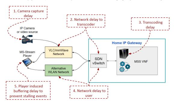
Figure 6.14: Different components of the end-to-end live latency
