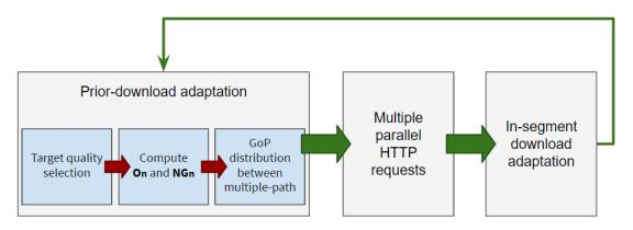
Figure 6.8: Overview of MSS/RRLH mechanisms for VoD
