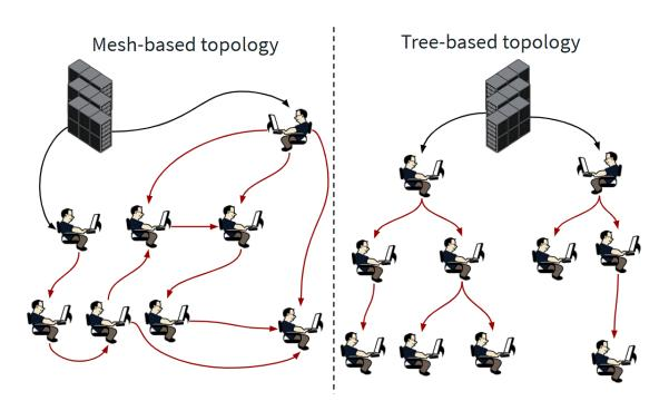
Figure 4.2: Mesh-based topology and tree-based topology
