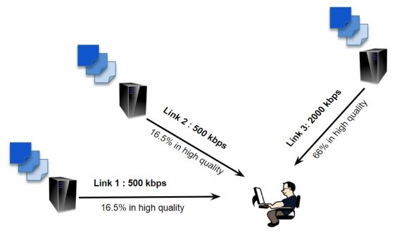
Visual quality of 3000 kbps by aggregating the bandwidths
