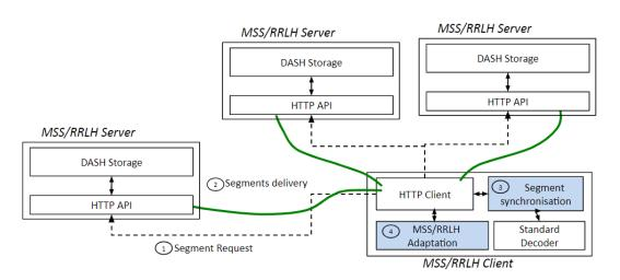
Figure 6.7: MSS/RRLH simplified logical architecture
