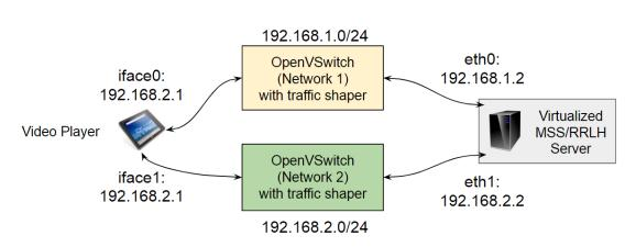
Figure 6.15: Experimental setup: the client is connected to the virtual server through two virtual network paths limited by traffic shapers
