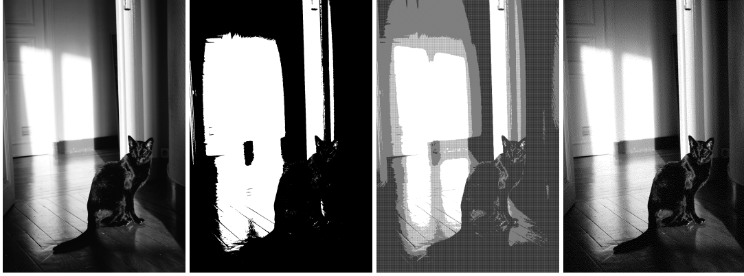
Figure 3.1: Result of dithering for different protocols. From left to right: original image, threshold dithering, ordered dithering (with the same matrix as described in the text), and error diffusion dithering (using a Floyd-Steinberg algorithm). The threshold method loses a lot of information, while the ordered dithering one creates unwanted patterns. The error diffusion result, on the other hand, is quite pleasing to the eye (dithering might only appear if you zoom in). All images are of size 1920 \times 1280 pixels.
