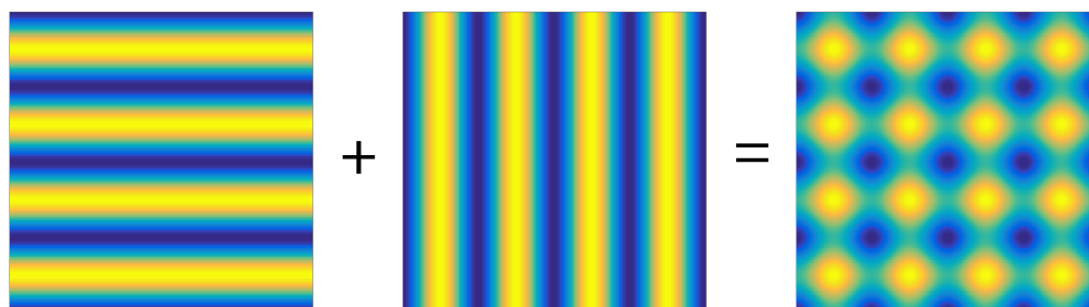
Figure A.3: It then suffices to add the vertical and the horizontal modulations to get the desired shape.
