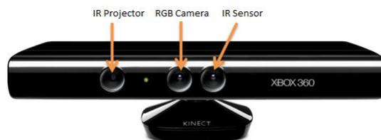
Figure 4.3 – Kinect V1 PrimeSense camera
