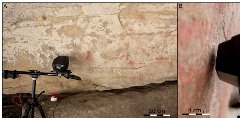
FIGURE VII.3 – The portable X-ray fluorescence ELIO spectrometer device during the analyses of Ghost Cave paintings (A) and Cycle of Life shelter (B).
