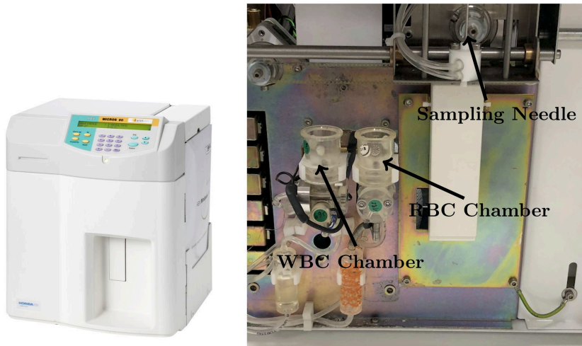
Figure 3.1 – Haematological automaton ABX Micros 60 developed by HORIBA Medical.
