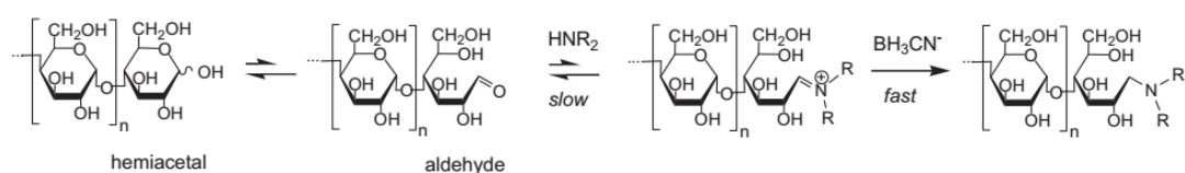
Fig. 1. 6 Reductive amination with cyanoborohydride at the reducing end of polysaccharide chain [37]
