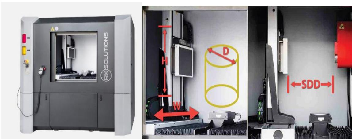
*Figure 5.15: Left: X-rays Tomograph, right: Internal structure of the Tomograph [180].*
