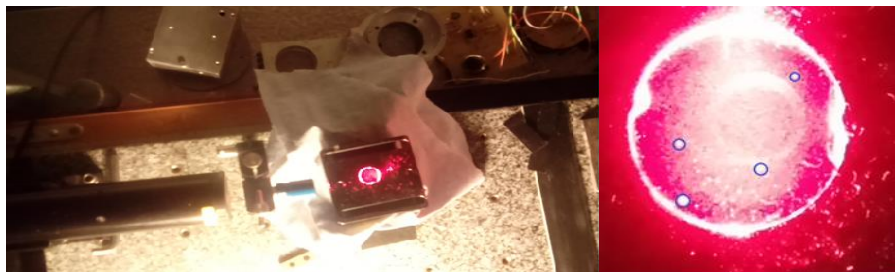
Figure 5.21: Left: Instrument passing the beam, Right: Enlarged illuminated crystal blade.
