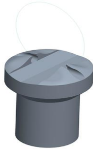
Figure 5.16: Holder with a quartz blade of 14 mm diameter.
