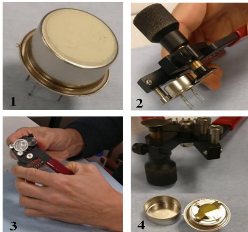
Figure 5.1: Dismantling of the quartz crystal resonator.
