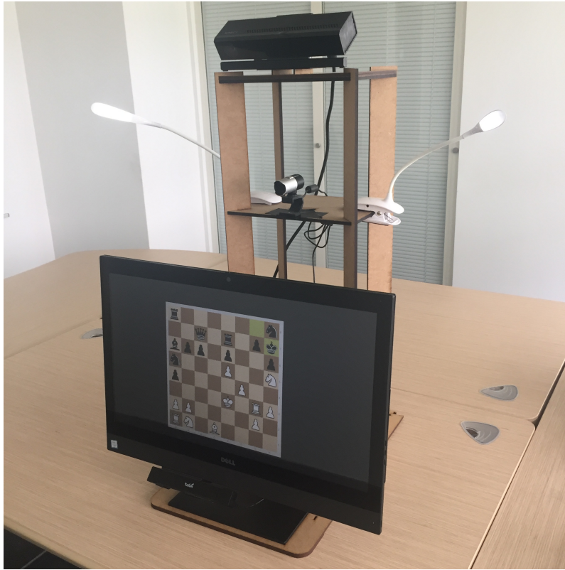
Figure 5.3: Designed Experimental Equipment for the CEEGE project, adapted from the Figurines project (Portaz et al., 2017). From top to down, sensors are: a Kinect2, a webcam, a touch-screen and a remote eye-tracking (below the screen). All these remote sensors are focusing on the subject engaged in problem-solving presented on the screen.
