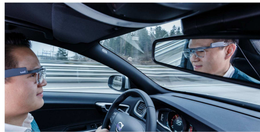
(b) A driver wearing eye-tracking glasses to capture is point of regard while engaged in a driving situation.
