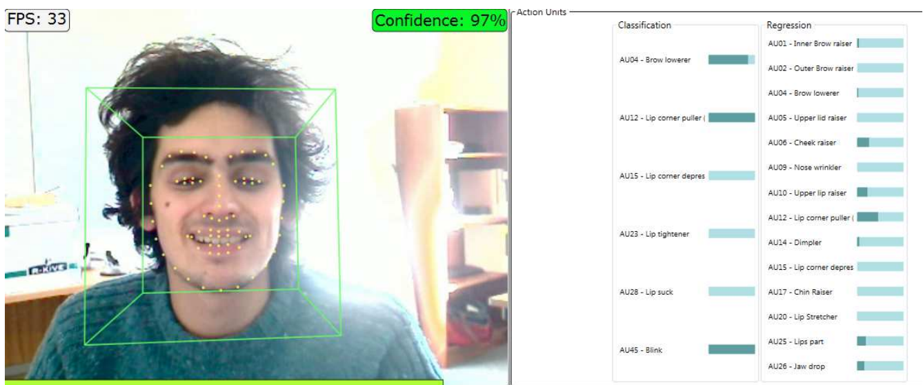
Figure 5.5: Facial Landmarks Detection with Head Pose Tracking (Left) and Action Units Detection (Right) Performed by OpenFace 2.0 (Source: Baltrusaitis et al., 2018)
