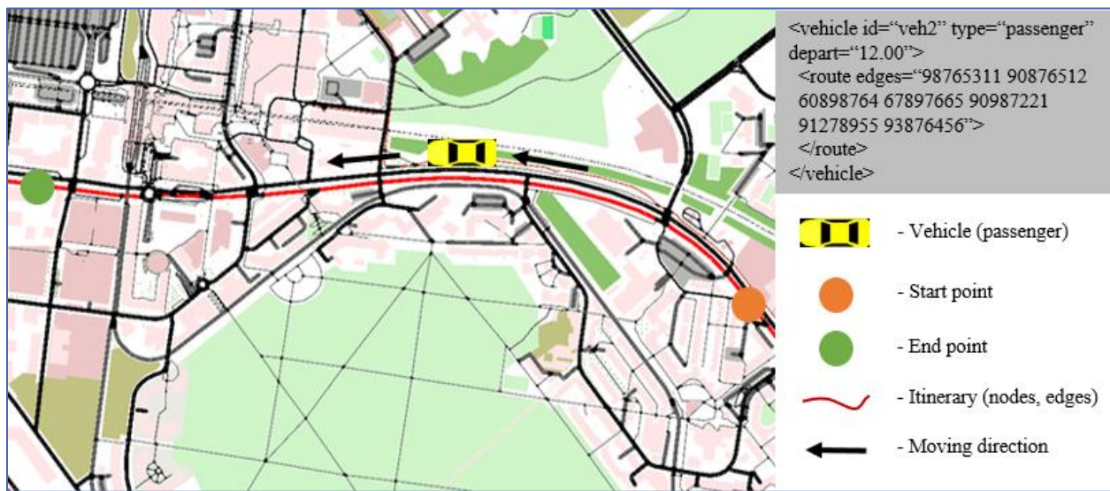
Figure 2-4. Vehicle itinerary presented in SUMO GUI interface
