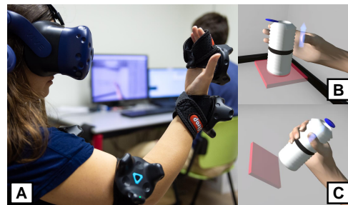
Figure 4 – Virtual reality setup. A: The subject wears a display headset and wireless motion trackers on the chest, upper arm, forearm and hand. B, C: Snapshots of the virtual scene during the grasping and placing phases. Credit © Gautier Dufau
