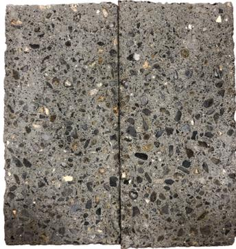
*Figure 2.2-5* Vertical cross section of reference high-strength grout
