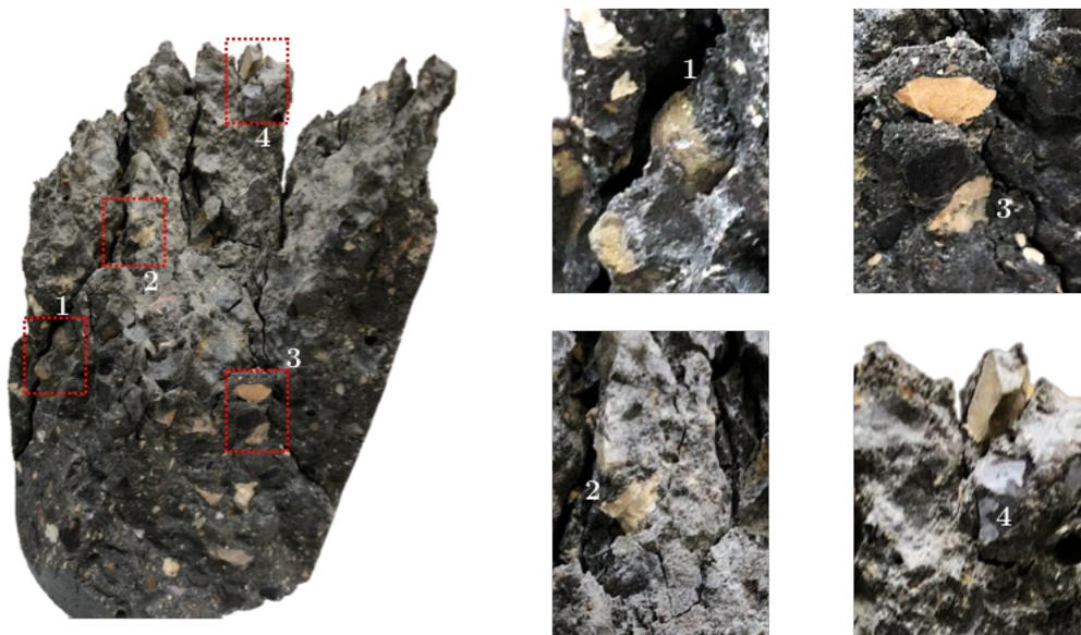
*Figure 4.4-7* Failure surface of a specimen with entrained air and areas with interface microcracking
