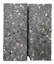
Figure 2.3-4 Increased water quantity and segregation (left); use of viscous agent (right)
