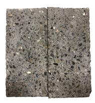
Figure 2.2-5 Vertical cross section of reference high-strength grout
