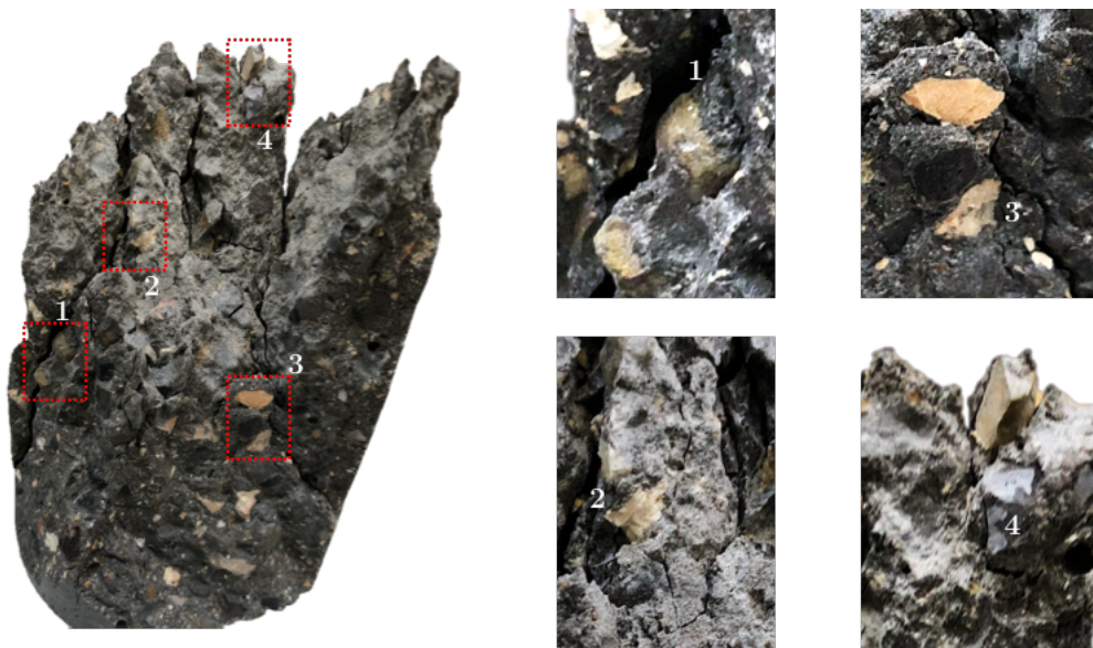
Figure 4.4-7 Failure surface of a specimen with entrained air and areas with interface microcracking
