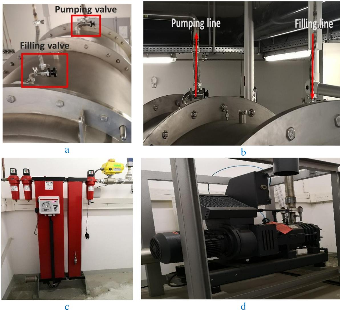
Figure II.6: (a) & (b) represent the pumping and filling valves and lines, (c) is the pure air generator and (d) is the pump coupled to *CHARME*.
