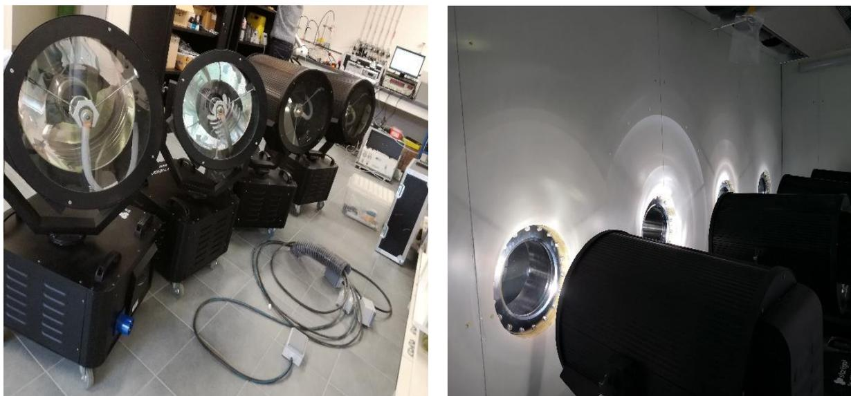
[Figure II.7](#): The light projectors (SKY TRACER 5000) that irradiate *CHARME*.
