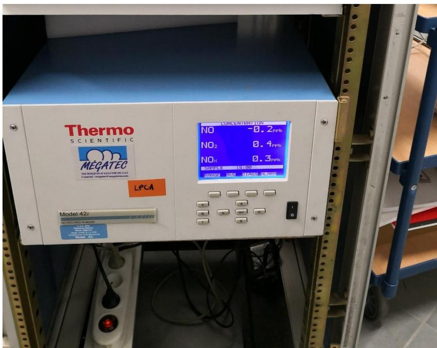
Figure II.13: NO<sub>x</sub> analyzer (chemiluminescence; Thermo Scientific 42i) coupled to CHARME.
