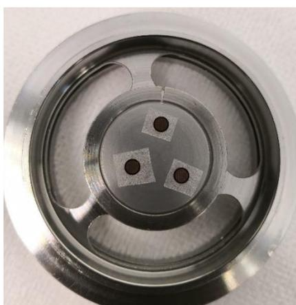
Figure IV. 12: One collection plate of the impactor with a nucleopore membrane and 3 lacey carbon grids.
