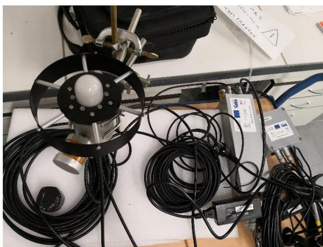
Figure II.11: The spectroradiometer (Metcon) used with *CHARME*.
