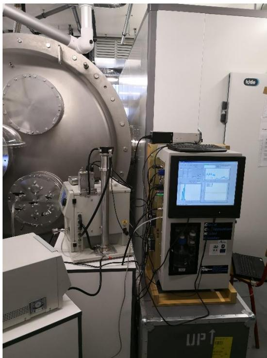
Figure II.19: The CCNc (DMT-100 Droplet measurement Technologies, USA) used to evaluate the CCN activity of particles in *CHARME*.
