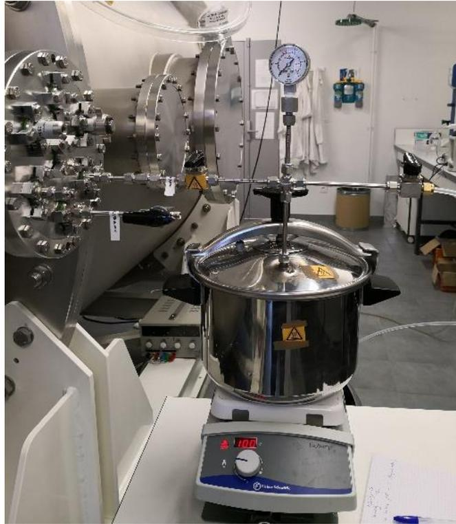
Figure III.4: The steam reactor used for introduction of water vapor.
