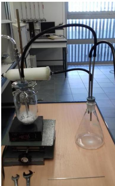
Figure III. 17: Setup used to introduce SiO<sub>2</sub> particles into the CHARME.
