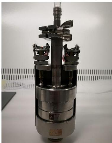
Figure IV. 11: The Dekati 3-stage cascade impactor used for sampling the SOA in *CHARME*.
