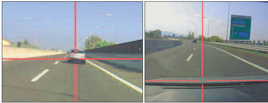
Fig. 4. Video created using the ASL software with a cross superimposed to the scene showing the eye fixations. In the left figure the vehicle was seen, in the right one it was not seen.
