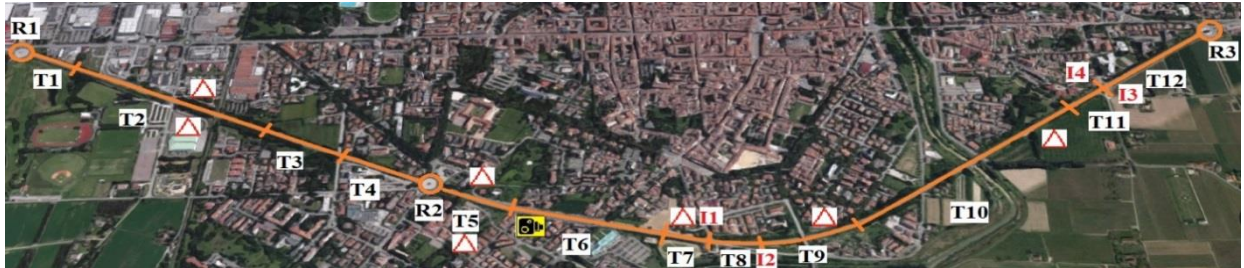
Fig. 1. The studied road: track subdivision (black), intersections (red), speed camera (yellow) and studied vertical signs (red triangles)
