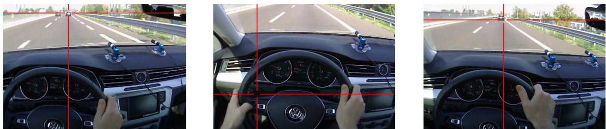
Figure 34. a. Driver gaze at the lead vehicle; b. driver gaze at dashboard; c. gaze back to lead vehicle
