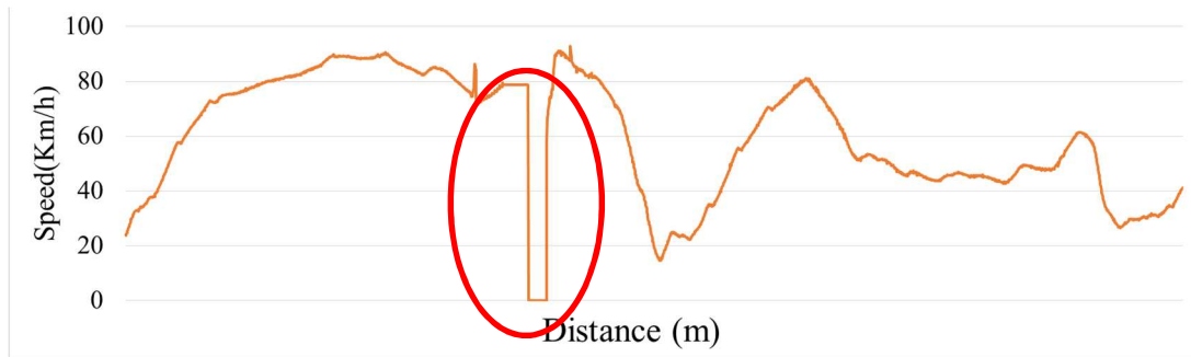
Figure 16. Velocity profile of one driver with a lost of GPS signal
