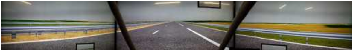
Figure 5. Visual cueing unit (View from the driver seat)
