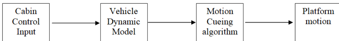
Figure 11. Motion cueing algorithm implementation
