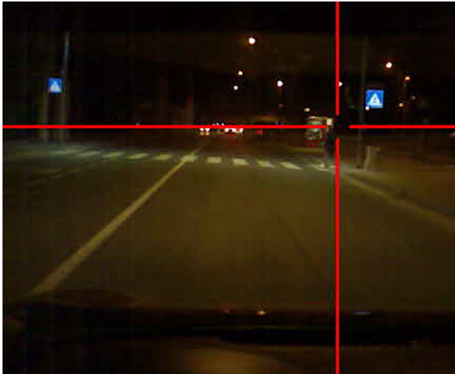
Fig. 6. Pedestrian crossing in condition 2 (enhanced lighting) from the point of view of the incoming driver. The red cross shows an ocular fixation of the driver towards the pedestrian. (For interpretation of the references to color in this figure legend, the reader is referred to the web version of this article.)
