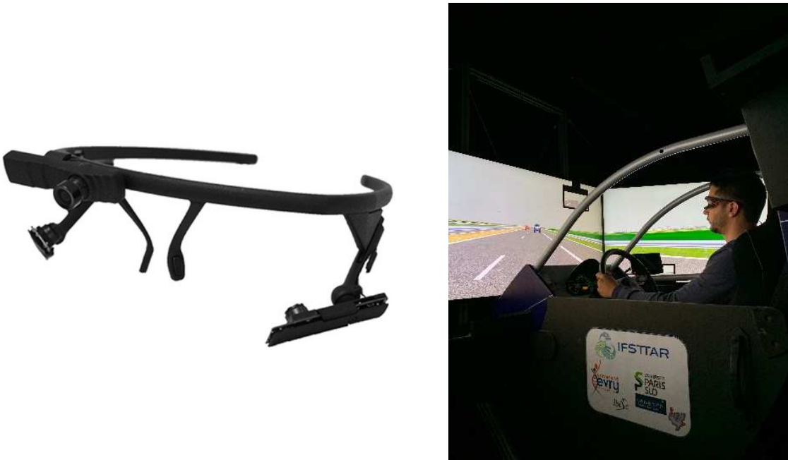
Figure 42. a. Pupil core eye tracker, b. participant during the simulation with eye tracker
