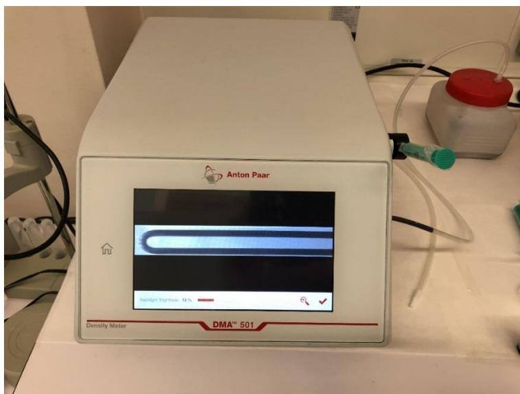
**Figure III.19.** Density meter DMA 501.
