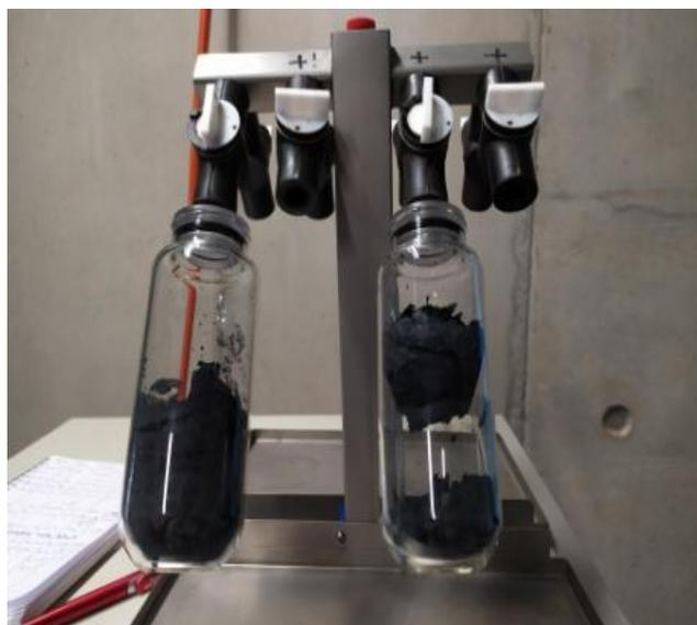
**Figure III.5.** Samples of FLG being freeze-dried.
