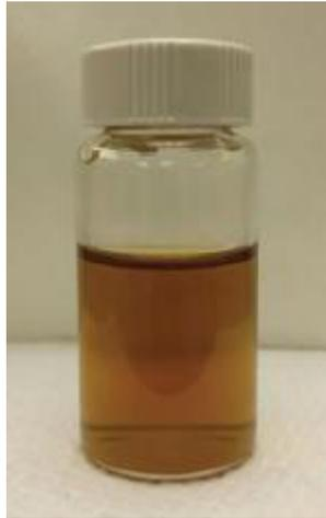
**Figure II.1.** Photograph of a graphene oxide aqueous nanofluid [2].
