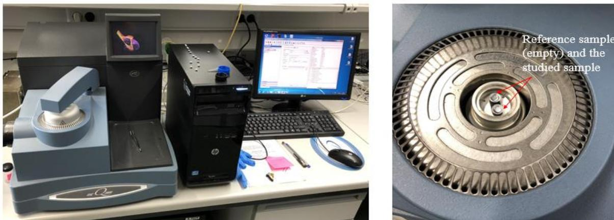
**Figure III.13.** Differential Scanning Calorimeter DSC-Q2000 apparatus.
