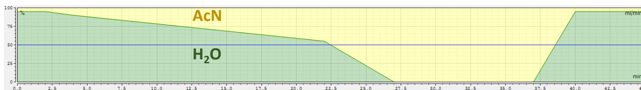
Figure 2 : Acetonitrile/water (AcN/ H 2 O) gradient used in the analytical and semi-preparative HPLC separations.
