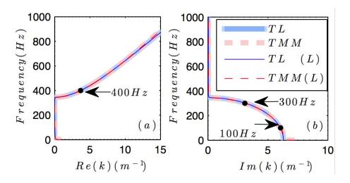
**Fig. III.4.** (a) and (b) respectively show the real and imaginary parts of the complex dispersion relation. Blue solid lines (Red dashed lines) show the results obtained by using TL approach, Eq. (III.45) (TMM, Eq. (III.49)). The thin (thick) solid and dashed lines correspond to the lossy (lossless) cases. The black points in Fig. III.4 show the frequencies used in the simulations, 400 Hz, 300 Hz and 100 Hz in chapter IV.
