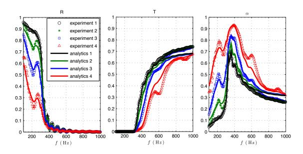
**Fig. IV.8.** (a) Reflection coefficients. (b) Transmission coefficients. (c) Absorption coefficients. Black circles (lines), green stars (lines), blue squares (lines) and red triangles (lines) present the experimental (analytical) results with the noise source around 100 dB (experiment 1), 120 dB (experiment 2), 130 dB (experiment 3) and 140 dB (experiment 4) respectively.
