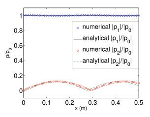
Fig. IV.3. Small deviation of approximate analytical solutions from the numerical simulations by using a cosinusoidal driver with  $p_0 = 4$  kPa,  $f_1 = 650$  Hz. Circles and squares depict numerical results, while solid and dashed lines correspond to the analytical (perturbative) findings.
