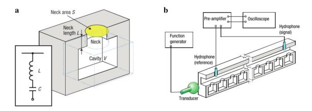
**Fig. I.5.** (a) Simple Helmholtz system; (b) Acoustic metamaterial with effective negative bulk modulus. (a) and (b) are adapted from Ref. [41].
