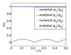
Fig. IV.4. Small deviation of approximate analytical solutions from the numerical simulations by using a cosinusoidal driver with  $p_0 = 10$  kPa,  $f_1 = 350$  Hz. Circles and squares depict numerical results, while solid and dashed lines correspond to the analytical (perturbative) findings.
