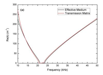
**Fig. I.6.** Dispersion relation for double negative acoustic metamaterials, adapted from Ref. [40].
