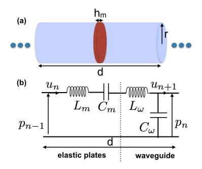
**Fig. II.1.** (a) One cell of acoustic waveguide loaded with clamped plates in linear regime, without considering viscothermal losses. (b) Corresponding unit-cell circuit.
