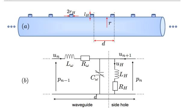
**Fig. III.3.** (a) Acoustic metamaterials composed of a waveguide loaded with an array of side holes. (b) Corresponding unit-cell circuit.
