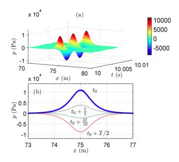
Fig. V.5. (a) 3D plot depicting the evolution of a gap soliton of the form of Eq. (V.35), obtained by numerically integrating the lossless version of Eq. (III.9)  $(R_{\omega} = 0)$  with  $\epsilon = 0.04$   $(2\epsilon\eta P_0 = 12158 \text{ Pa})$ , in a lattice with a length of 150 m. (b) Numerical spatial profiles of gap soliton measured from  $t_0$  (at which gap soliton has a maximal amplitude) to  $t_0 + T/2$  (at which gap soliton has a minimal amplitude).
