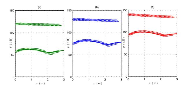
Fig. IV.10. Experimental and analytical results about dispersion managed, second harmonic generation. The sources are  $A\sin(\omega t)$  with different amplitude, (a) A = 120 dB, (b) A = 130dB and (c) A = 140 dB. The symbols (lines) are experimental (analytical) results. Circles (squares) stand for the experimental results of  $p_{\omega}$  ( $p_{2\omega}$ ). Dashed (solid) lines stand for the analytical results of  $p_{\omega}$  ( $p_{2\omega}$ ).
