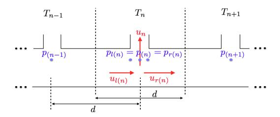
Fig. IV.9. Schematic of *n*-th side hole.
