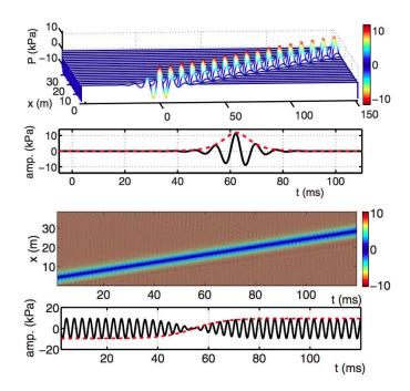
**Fig. I.7.** In the first (third) panel: contour plot of a bright (dark) soliton. In the second (fourth) panel, the black continuous (red dashed) line depicts the numerical (analytical) result for the sech- (tanh-) shaped envelope. [44].
