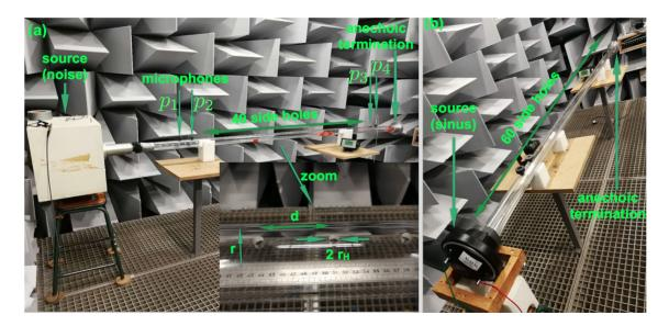
**Fig. IV.7.** (a) Pictures of the experimental setup for amplitude-dependent reflection, transmission and absorption coefficients. (b) Picture of the experimental setup for dispersion managed, second-harmonic generation.
