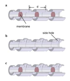
**Fig. I.4.** (a) Membrane-type acoustic metamaterial with effective negative mass density; (b) Hole-type acoustic metamaterial with effective negative bulk modulus; (c) Double negative acoustic metamaterials. (a)-(c) are adapted from Ref. [35].
