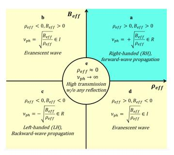
Fig. I.1. Effective mass density  $\rho_{eff}$  and bulk modulus  $B_{eff}$  diagram [1].  $v_{ph}$  denotes the phase velocity. R and I indicate purely real and imaginary part of phase velocity, respectively. Normal materials in nature belong to (a) with double positive parameters. Metamaterials can be classified as negative mass density (b), double negative parameters (c), negative bulk modulus (d) and near-zero mass density (e).
