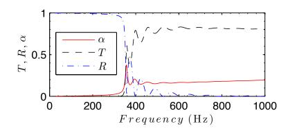
Fig. III.5. The frequency dependent transmission T (black dashed line), reflection R (blue dot-dashed line) and absorption  $\alpha$  (red continuum line) coefficients for a lattice of 1.7 m (~ 34 cells).
