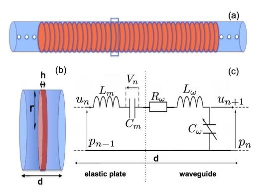
**Fig. III.1.** (a) Waveguide loaded with an array of clamped plates; (b) the unit-cell of the system; (c) corresponding unit-cell circuit.
