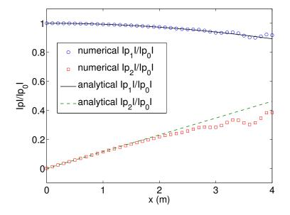
Fig. IV.1. Fubini solution, for the wave propagation in a uniform waveguide without clamped plates or side-holes, with f = 400 Hz. Solid and dashed lines depict analytical results, while circles and squares depict numerical ones. Black solid line and blue circles represent the fundamental component, while dashed green line and green squares correspond to the second harmonic component. The numerical results have a good agreement with the Fubini solution at the beginning of the lattice.
