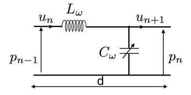
Fig. II.4. Unit-cell circuit of weakly nonlinear wave propagation in acoustic waveguide, without considering viscothermal losses.
