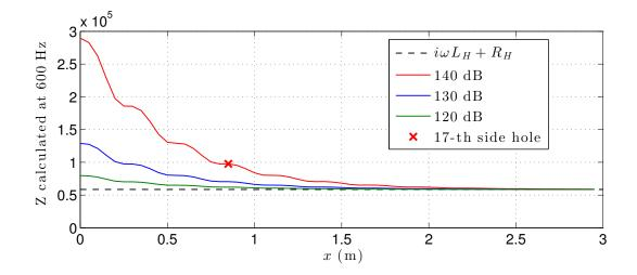
Fig. IV.11. Real part of acoustic impedance of each side hole calculated at 600 Hz (frequency of the source). Amplitude-dependent impedance of the side holes are shown in red (140 dB), blue (130 dB) and green (120 dB) lines. The linear part (back dashed line),  $\text{Re}(i\omega L_H + R_H)$ , is independent of the position of the side holes. Acoustic impedance of 17-th side hole for the case of 140 dB is noted by red cross.
