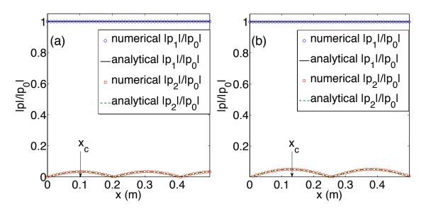
Fig. IV.2. Harmonic generation in the presence of dispersion in the case of a cosinusoidal driver with frequency in the propagating band. The amplitude of the second harmonic oscillates in space due to the phase mismatch. Circles and squares depict numerical results, while solid and dashed lines correspond to the analytical (perturbative) findings. Both  $|p_1| / |p_0|$  (upper) and  $|p_2| / |p_0|$  (lower) are in the pass band. (a) f = 350 Hz; (b) f = 400 Hz.
