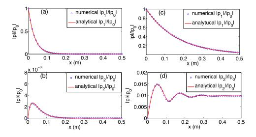
Fig. IV.5. Harmonic generation in the presence of dispersion in the case of a cosinusoidal driver with frequency in the band gap. Blue circles and red lines depict, respectively numerical and analytical results. (a) f = 90 Hz,  $|p_1|/|p_0|$  in the band gap; (b) f = 90 Hz,  $|p_2|/|p_0|$  in the band gap; (c) f = 300 Hz,  $|p_1|/|p_0|$  in the band gap; (d) f = 300 Hz,  $|p_2|/|p_0|$  in the pass band.
