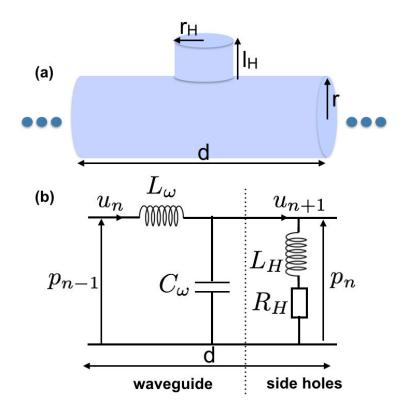
**Fig. II.2.** (a) One cell of acoustic waveguide loaded with side holes in linear regime, without considering viscothermal/radiation losses. (b) Corresponding unit-cell circuit.
