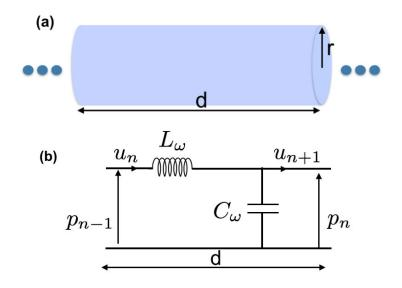
Fig. II.3. (a) One cell of 1D acoustic waveguide of radius r. The length of the cell is d. (b) The unit-cell circuit of the equivalent TL model of the acoustic waveguide.
