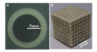
**Fig. I.2.** (a) Cross section of a coated lead sphere that forms the basic structure unit; (b) An  $8 \times 8 \times 8$  cubic crystal. (a) and (b) are adapted from [12].
