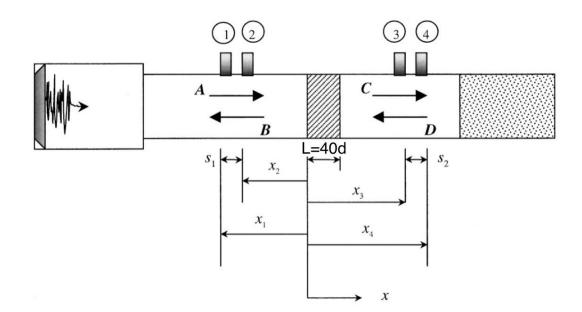
Fig. VII.1. Schematic diagram of the standing wave tube, adapted from Ref. [121].
