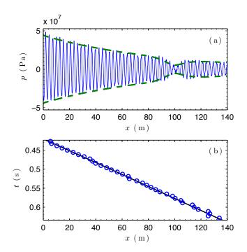
Fig. V.13. (a) Numerical spatial profile of dissipative gray soliton calculated at t = 0.58 s with  $\phi = \pi/8$  (blue line). Green dashed lines are the corresponding analytical envelope, Eq. (V.75).; (b) The corresponding space-time diagram of dissipative gray soliton (blue circles). The slop of the black line shows the analytical velocity of dissipative gray solitons, Eq. (V.76).
