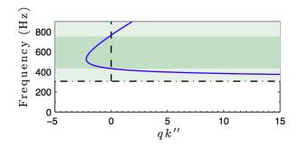
Fig. V.1. The frequency dependence of qk", the product of the dispersion and nonlinearity coefficients of the NLS equation. The light (dark) green region corresponds to the focusing (defocussing) case, with qk" > 0 (qk" < 0).
