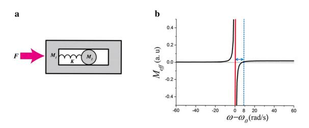
**Fig. I.3.** (a) Simple mass-spring system; (b) Effective inertial response as a function of angular frequency. (a) and (b) are adapted from [30] and [1] respectively.
