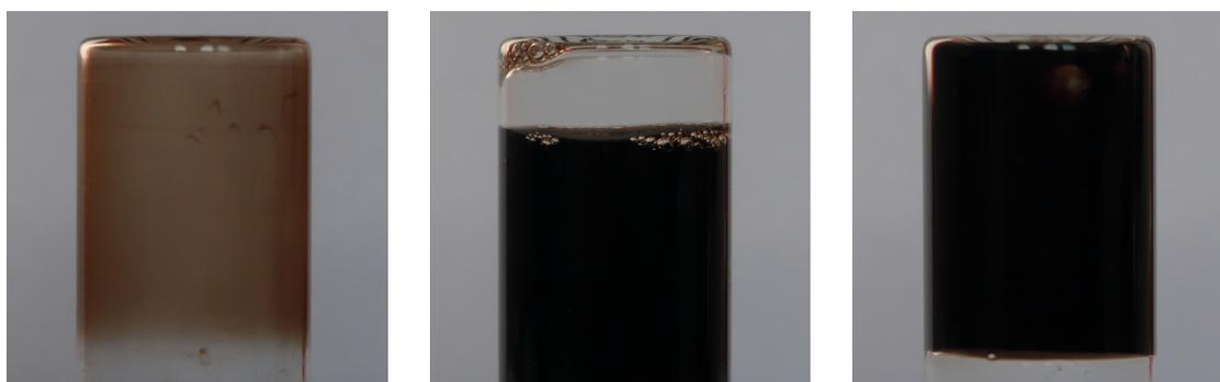
**Figure IV.10:** Polydopamine samples. **Left:** Glass vial after polymerization without imogolite present. **Right:** Sample after polymerization with imogolite present. Note that there is no deposit on the glass vial. **Right:** Sample after polymerization with imogolite present. When left to rest, a gel forms that turns liquid again after agitating the sample.
