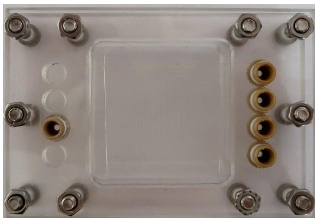
**Figure II.42:** Top view on the PMMA device holder.
