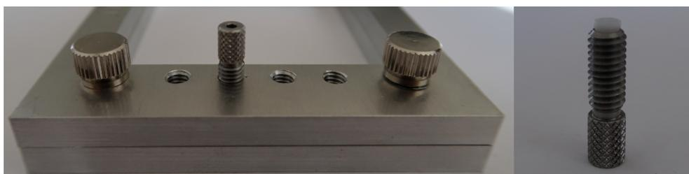
**Figure II.14:** Left: IMT device holder with tube connector. Right: IMT tube connector with PTFE gasket.
