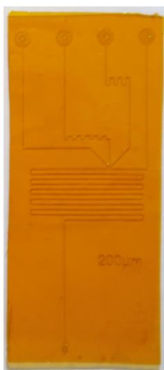
**Figure II.17:** A finished polyimide/OSTE+ composite device.
