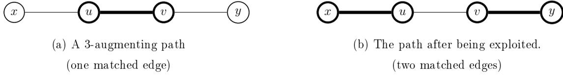
Figure 4.2 – An example of exploitation of an augmenting path. On the left we have the initial matching and on the right the new matching after exploitation of the augmenting path.
