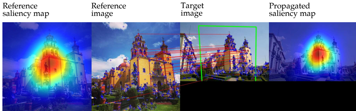
Figure 5.7: Saliency map generation through homography estimation. Green polygon over target image shows the transformation given estimated homography when the polygon condition is satisfied. The red lines depicts keypoints matching. For saliency maps over images: red means more attention and blue less attention (jet colormap is used).
