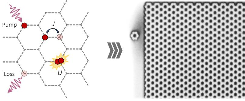
Figure 2.16: **A photonic platform for analog simulation:** (Left) schematic representation of a honeycomb lattice for interacting bosons subject to pump and losses. (Right) SEM image of the corresponding analog implementation with coupled microcavities, image adapted from [190].
