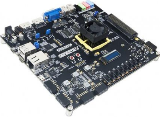
Figure VI-21: Genesys 2 board used for FPGA implementation
