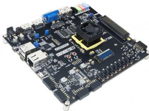
Figure VI-21: Genesys 2 board used for FPGA implementation
