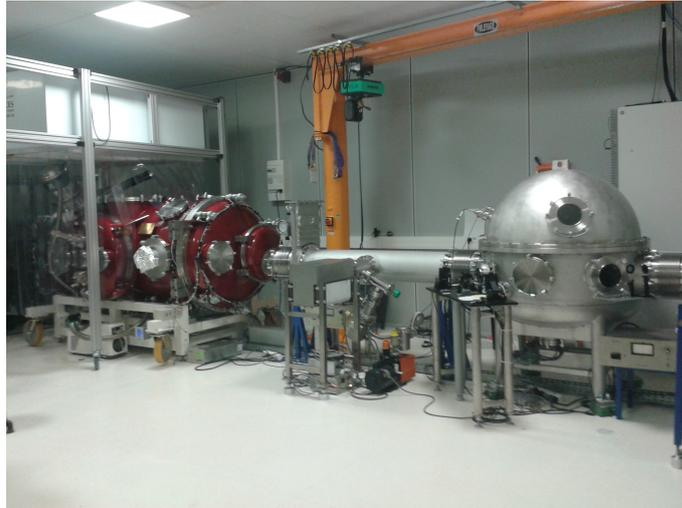
Figure 4.1 – First clean room of CALVA with the red tank, named Ferrarix, used for the in-vacuum preparation bench of the Exsqueeze experiment and the grey tank where the first mirror of the filter cavity stands.
