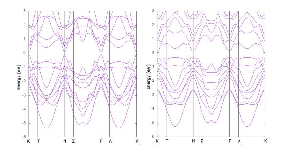
Figure 2.6: Band structure a) without and b) with spin orbit interactions.
