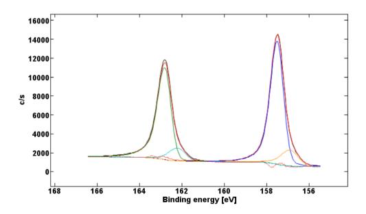
Figure 4.14: Fit of the  $Bi4f_{7/2}$  doublet for the 6 nm thick film showing the contributions from the  $Bi_2Te_3$  (high intensity doublet) and Bi (low intensity doublet).
