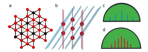
Figure 4.2: a - View on the c plane (001) of  $Bi_2Te3$  cell. b - Two main symmetry planes in the hexagonal cell, the difference between them is precisely 30°. c and d - Artistic representation of diffraction pattern made with RHEED along with two main symmetries, colors are corresponding to the planes marked in picture b; the received pattern is in reciprocal lattice.
