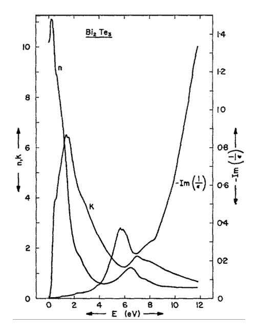
Figure 7.4: Optical constants n and k of  $Bi_2Te_3$  and energy loss function  $-Im(1/\epsilon)$  from Kramers-Kroning analysis,  $E \perp c$ . From Greenaway J. Phys. Chem. Sol. (1965)[38].
