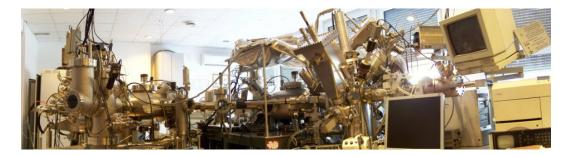
Figure 3.6: High vacuum cluster in laboratory of Surface Physics in Institute of Physics, University of Silesia.
