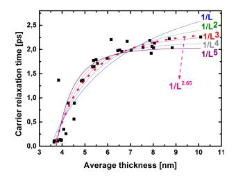
Figure 5.17: Results of fitting the power of law function to the time of relaxation of hot carriers versus the film thickness. The performed calculation resulted in the relaxation of the fitting procedure close to  $\alpha = 2.65$ .
