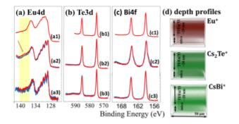
FIG. 2. The XPS photoemission spectra of (a) Eu4d (b) Te3d (c) Bi4f. Spectra obtained (a1) for 20nm thick Eu grown on Mo substrate, (b1, c1) Te3d and Bi4f of 15 nm thick Bi2Te3 layer respectively, (a2, b2, c2) after deposition of 2 nm thick Eu layer, (a3, b3, c3) after deposition of 2 nm thick Bi2Te3 top layer. Blue lines correspond to angle dependent XPS measurements. 3D depth profiles (d) represent distribution of Eu ions and (Te or Bi) cesium ions within the heterostructure.
