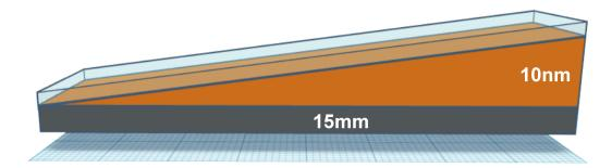
Figure 3.8: Sample B2 - art view of monocrystaline wedge of  $Bi_2Te_3$  with slope of 0.66nm/mm.
