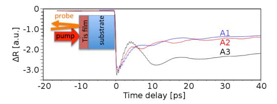
Figure 5.9: Time-resolved optical reflectivity obtained for samples  $A_1, A_2, A_3$ , data was normalized to largest magnitude for clarity.
