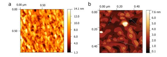
Figure 4.1: a  $-1 \times 1 \mu m$  AFM image of sample A2,  $Bi_2Te_3$  grown on Si(001). b  $-0.45 \times 0.45 \mu m$ AFM image of sample A1 grown on Muscovite mica (110). From R.Rapacz [30]
