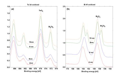
Figure 4.15: XPS doublets of  $Te3d_{5/2}$  (a) and  $Bi4f_{7/2}$  (b) after oxidation of the film.
