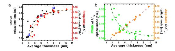
Figure 5.15: Thickness dependence of the ultrafast carrier and phonon dynamics. a - Thickness dependence of the electron-phonon relaxation time for the wedge B2 (black squares) and step B1 (centered blue squares) samples. Thickness dependence of the  $A_{1g}^1$  optical phonon frequency (red dots). b - Thickness dependence of the A1g optical phonon amplitude (gold squares) and full width at height maximum (green dots).
