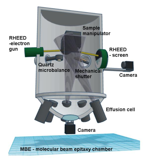
Figure 3.5: Model of MBE chamber used in our experiments.
