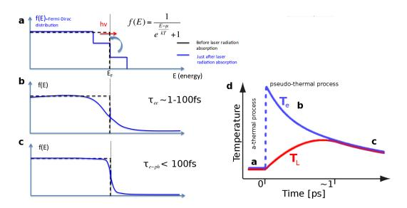
Figure 5.3: Time dependence of the Fermi distribution after an ultrafast laser exciton: a - photon energy is first absorbed by the electrons, b - thermalization of the electronic subsystem, c - thermalization of the electronic subsystem with the phonon (cations) subsystem. d - TTM two temperature model shows the time scale of the processes mentioned earlier.
