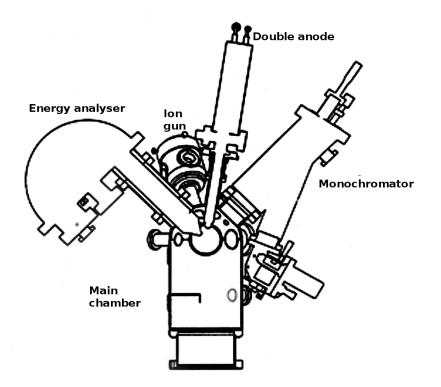
Figure 4.10: Schematic of *PhysicalElectronicsPHI*5700 spectrometer.
