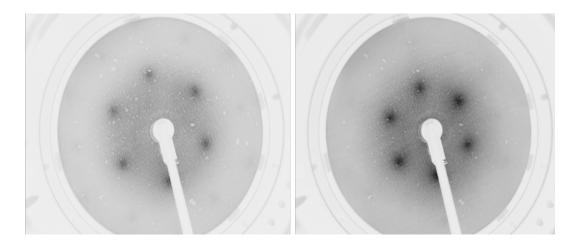
Figure 4.8: LEED diffraction image of sample C3 reviling characteristic  $Bi_2Te_3$  hexagonal crystal structure. Broadening of the diffraction spots is a result of slight mismatch between nearest QL's.
