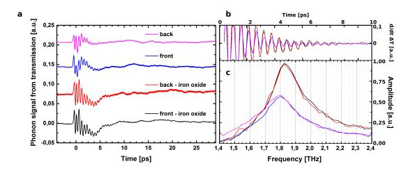
Figure 5.22: Time-resolved transmission ( $\Delta T$ ) obtained for the sample C1. The graph presents the extracted phonon signals. b - presents overlapped derivatives of the signal showing, in real-time, the difference in frequency. Graph c presents the FFT showing the appearance of a blue shift of  $A_{g1}^1$  frequency in  $Bi_2Te_3$  doped with iron oxide.
