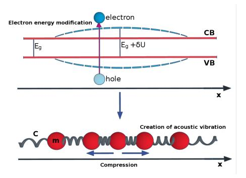
Figure 5.6: Deformation potential in band structure picture: excitation of an electron-hole pair disturbs the electronic distribution and modifies the interatomic interaction leading to a change of atomic positions and consequently to the generation of a strain field.
