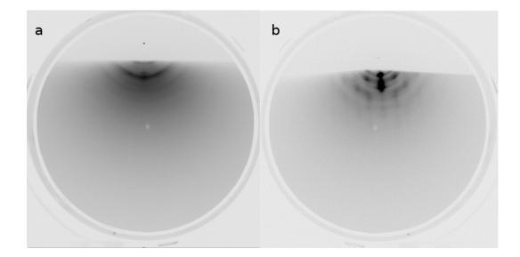
Figure 4.5: RHEED diffraction image of sample a - A2 and b - A3. Observed half circles are proof polycrystalline growth of the sample.
