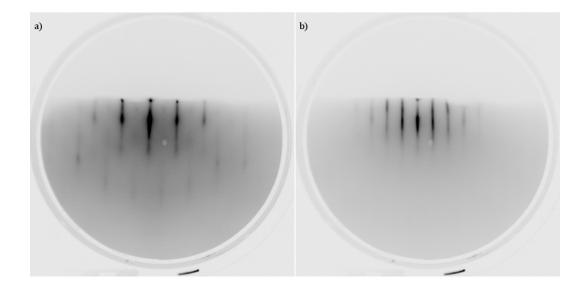
Figure 4.4: RHEED diffraction image of sample A1 along two main planes of symmetry characteristic to  $Bi_2Te_3$  hexagonal crystal structure. Detected streaks are proof of monocrystalline terrace growth of the sample.
