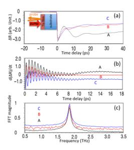
FIG. 2. (Color online) (a) Time-resolved optical reflectivity obtained for  $Bi_2Te_3$  thin films deposited on various substrates: films A–C (see text for details on samples). Curves have been normalized to the largest magnitude point for clarity. (b) A1g(I) optical phonon signals. (c) Corresponding fast Fourier transform of curves shown in (b).
