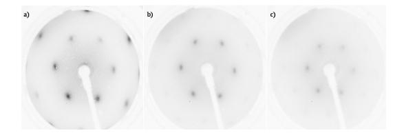
Figure 4.7: LEED diffraction image of sample A1 at different electron incident energies a) 56eV; b) 75eV; c) 98eV.
