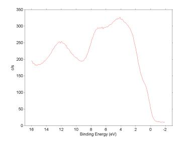
Figure 4.18: XPS spectra of valence band after the oxidation.
