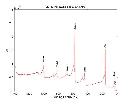
Figure 4.11: Typical XPS spectra of pure  $Bi_2Te_3$  sample.
