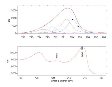
Figure 4.17: XPS spectra of Fe2p3/2 core level.
