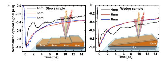
Figure 5.14: Ultrafast optical response of ultrathin layers of  $Bi_2Te_3$ . Time-resolved optical reflectivity obtained for various layers of  $Bi_2Te_3$  for the a - step B1 and b - wedge B2 sample. The signals are normalized to the maximum of the electronic peak. (insets) The pump and probe are represented in the artist's view as red and orange beams.
