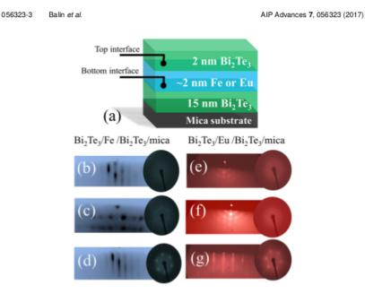
FIG. 1. Structure of deposited heterostructures (a) combined with diffraction patterns obtained with the use of RHEED and LEED at each step of deposition process for (b) 2nm of Bi<sub>2</sub>Te<sub>3</sub> top layer, (c) 2.4nm Fe, (d) 15nm Bi<sub>2</sub>Te<sub>3</sub> bottom layer along [100] direction, (e) 2nm Bi<sub>2</sub>Te<sub>3</sub> top layer, (c) 2 nm Eu, (d) 15nm of Bi<sub>2</sub>Te<sub>3</sub> bottom layer along [1-20] direction.
