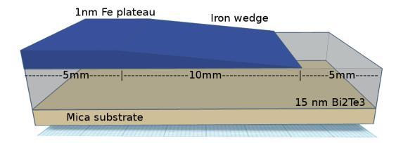
Figure 3.9: Sample C2 - art view of monocrystaline sample of  $Bi_2Te_3$  with 3 sections: 1st - plateau of iron with a thickness 1nm and lenght 5mm; 2nd - wedge of iron with gradient 1Å/mm; 3rd - free surface sample of BT.
