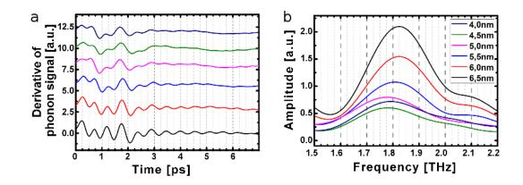
Figure 5.16: a - Typical oscillatory component at a short time scale revealing the A1g optical phonon. b - Fast Fourier Transform (FFT) of the signal shown in a reveal that the  $A_{1g}^1$  mode is softening for the ultrathin layer.
