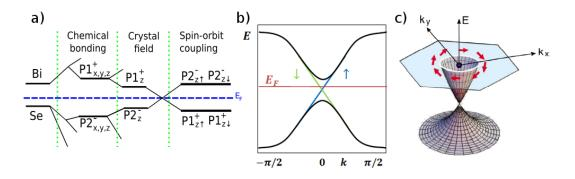
Figure 2.1: a - Evolution of the molecular band structure leading to appearence of TI state. b - Schematic of the spin-polarized surface-states dispersion in bismuth based TI. Green and blue arrow indicate the polarization of the spin. c - 3D visulization of the Dirac cone in TI. From Hasan and Kane (2010).
