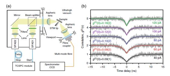
**Figure 2.17:** Single photon emission from a ZnPc molecule. (a) Experimental setup. (b) Second-order correlation function as a function of the time delay for different tunneling currents. Adapted from [132]
