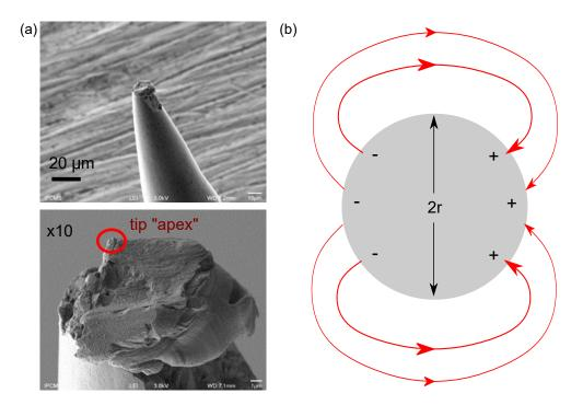
**Figure 2.5: Description of Localized Surface Plasmons confined in the subwavelength size tip apex.** (a) Scanning Electron Microscopy image of a tungsten tip covered with silver. The tip apex area (red circle) presents metallic structures smaller than 0.1 micrometer. (b) Sub-wavelength size metallic sphere model of the tip apex. Charge oscillations are confined in the sphere. The red arrows represent the generated electric field lines.
