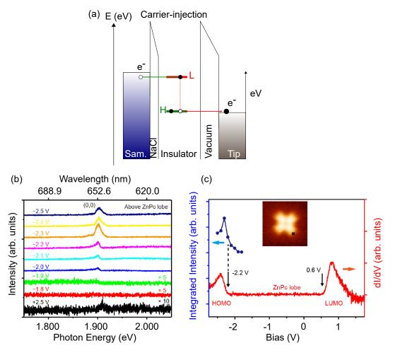
**Figure 2.18:** Carrier injection mechanism at negative bias voltage. (a) Energy sketch of the mechanism. An electron is injected from the sample in the LUMO and a hole is injected from the tip in the HOMO. A voltage drop is present on both sides of the junction. (b) Voltage dependency of the STM-LE intensity of a single ZnPc. (c) Comparison of the voltage dependency of the integrated STM-LE intensity and the differential conductance of a single ZnPc. (b) and (c) are adapted from [129].
