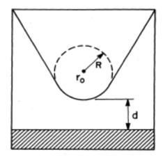
Figure 1.6: Sketch of the tip geometry assumed by Tersoff and Hamann. The end of the tip is assumed to be a sphere or radius *R*. The center of the sphere is located to  $\mathbf{r}_0$ , the tip-sample distance is d. Reproduced from [118].
