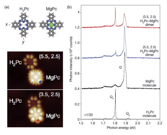
**Figure 2.13:** Intermolecular energy transfer via dipole-dipole interaction. (a) Sketch of the experiment. (b) Dimer of  $H_2Pc$  and MgPc molecules. (c) STM-LE spectra obtained. The two top spectra are acquired at the position marked by a dot in (b). Adapted from [49].
