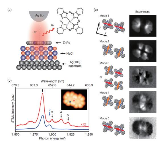
**Figure 2.11: Coherent dipole-dipole coupling.**(a) A ZnPc molecule is decoupled from a Ag(100) surface by a three atomic NaCl layers. (b) STM-LE spectra of a ZnPc dimer excited at the corresponding colored cross in the STM image inset. The five different peaks correspond to five different coupling modes. (c) Experimental maps for the five peaks compared with theoretical maps. Adapted from [129]
