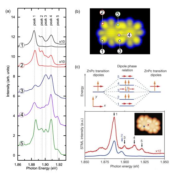
**Figure 4.5:** Spatial variation of the supra-molecular exciton emission (a) STM-F spectra recorded at the different positions marked in (b). Spectra 3, 4, and 5 are arbitrarily magnified to emphasise the different electronic modes. (b) STM images of the ZnPc dimer. (c) Sketch depicting the attribution by Zhang *et al.* of the five peaks appearing in (a) to five dipole coupling modes (Adapted from [129]).
