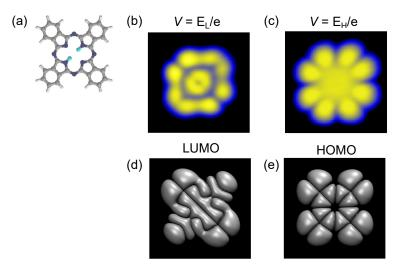
**Figure 1.10:** Voltage dependency of STM images. (a) Topological structure of an H<sub>2</sub>Pc molecule. (b) STM image of the H<sub>2</sub>Pc LUMO orbital ( $3 \times 3 \text{ nm}^2$ ; V = +0.5V; I = 10pA). (c) STM image of the H<sub>2</sub>Pc HOMO orbital ( $3 \times 3 \text{ nm}^2$ ; V = -2.5V; I = 10pA). (d) LUMO orbital obtained by DFT. (e) HOMO orbital obtained by DFT.
