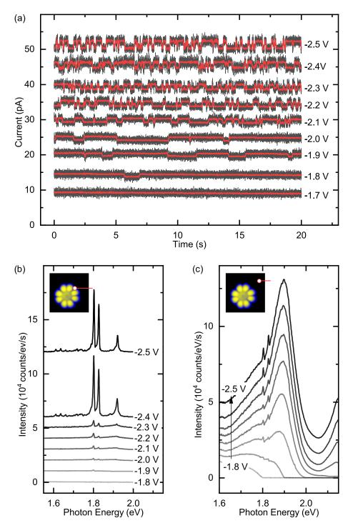
**Figure 3.12:** Voltage onset of the tautomerization process. (a) Current traces at different voltages (initial current setpoint I = 10 pA). (b) Series of fluorescence spectra (I = 10 pA; acquisition time t = 180 s) acquired at different voltages at the position marked by a dot in the STM image in inset. (c) Series of fluorescence spectra (I = 600 pA; acquisition time t = 180 s) acquired at different voltages at the position marked by a dot in the STM image in inset.
