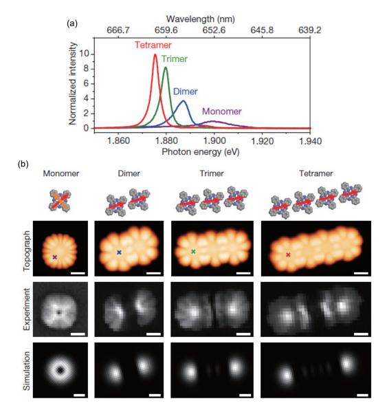
Figure 2.12: Evolution of the lowest energy coupling mode as a function of the number of molecules. (a) Top pannel: Spectra of a monomer, dimer, trimer and tetramer of ZnPc. Spectra are acquired at the cross-marked position in (b). Intensities are normalized by the monomer one. (b) Corresponding experimental photon maps compared to the simulated maps. Adapted from [129].
