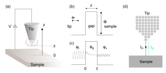
**Figure 1.3: Origin and description of the tunnel current.** (a) Sketch of the STM junction. (b) Energetic sketch of the junction from a classical point of view. (c) Energetic sketch of the junction from a quantum point of view. (d) Description of the apex of the tip (red circle in (a)).
