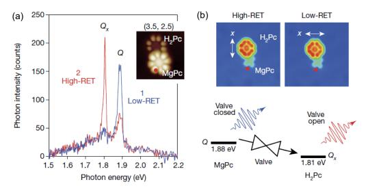
**Figure 2.14:** Energy transfer controlled with dipoles respective orientations. (a) Spectra illustrating the two regimes of energy transfer. The two spectra are acquired a the position marked by a dot in the STM image inset. (b) STM images of the dimer in the two energy transfer regimes. The LUMO image of the  $H_2Pc$  molecule shows a symmetry axis related to the orientation of the  $Q_x$  transition. Adapted from [49]
