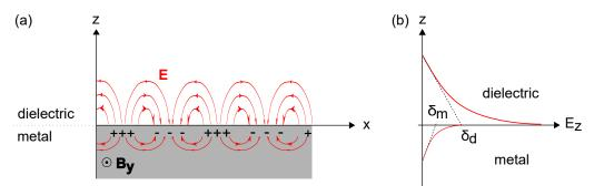
**Figure 2.3:** Description of the Surface Plasmon Polariton (SPP). (a) Sketch depicting the structure of the SPP wave. Collective oscillations of conduction charges are localized in the vicinity of the metal surface. The generated field is both transferal and longitudinal. Red arrows represent the electric field. (b) The evanescent character of the electric field z component.  $\delta_d$  and  $\delta_m$  are the decay lengths of the latter in the dielectric and the metal respectively.
