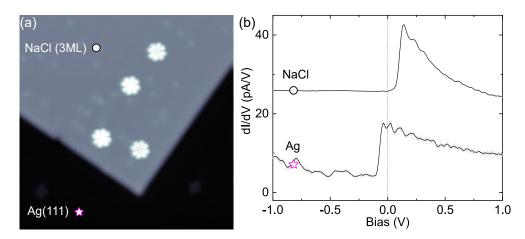
**Figure 3.13:** Interface state on NaCl. (a) STM image (V = -2.5 V; I = 10 pA; 30  $\times$  30 nm<sup>2</sup>) of four H<sub>2</sub>Pc molecules on a three layer NaCl island deposited on Ag(111). (b) Differential conductance spectra allowing to identify the energy position of the surface state on NaCl and Ag(111).
