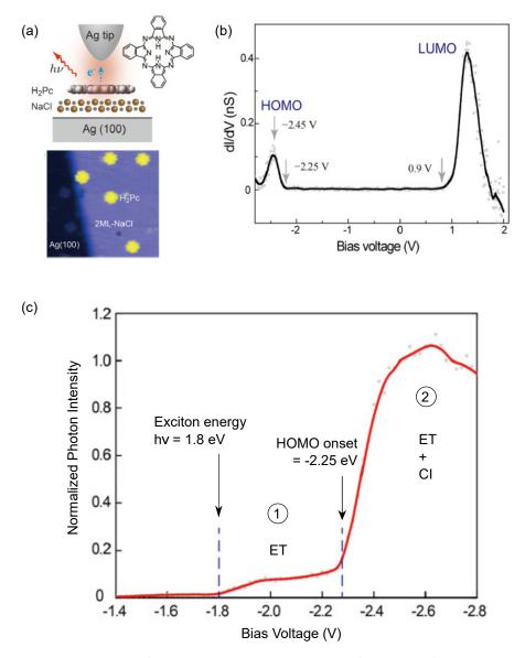
**Figure 2.20:** STM-LE of a single  $H_2Pc$  molecule as a function of the voltage. (a) Sketch of the experiment. (b) Differential conductance as a function of the voltage. The resonance peak at negative voltage (resp. positive) corresponds to the HOMO state (resp. LUMO). (c) STM-LE as a function of the voltage. Adapted from [16]
