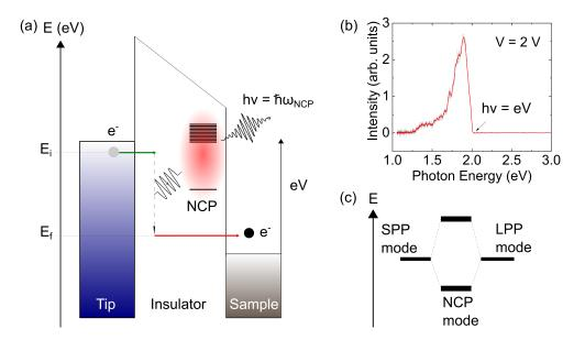
**Figure 2.7:** Light emission process in a metal-metal junction. (a) An inelastic tunneling transition excites an NCP mode that decays into a photon in the far field. (b) Broadband emission spectrum of the NCP at a bias voltage V = 2 V. The spectral shape depends on the spectral density of the NCP modes. The spectrum shows a quantum cutoff at hv = 2 eV. (c) Energetic sketch illustrating the hybridization between LSP and SPP that generate NCP modes.
