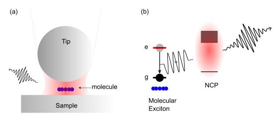
**Figure 2.8:** Decay of a molecular excitation in a plasmonic nanocavity. (a) A molecule is placed in the gap on the STM junction. (b) The molecular excitation decays toward NCP modes due to fluctuations of the plasmonic vacuum. NCP excitations decay into photons in the far-field at the molecular exciton energy.
