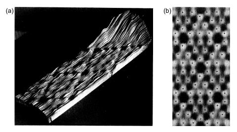
Figure 1.1: Image of the surface reconstruction of Si(111) with STM (a) Relief form of the original recordings of two complete  $7 \times 7$  units cells. (b) Top view of (a) The two diagonals of the unit cell are  $29 \pm 4$  Å and  $46 \pm 1$  Å in good agreements with the crystallographic values at that time (26.88 Å and 46.56 Å respectively.). Reproduced from [8]
