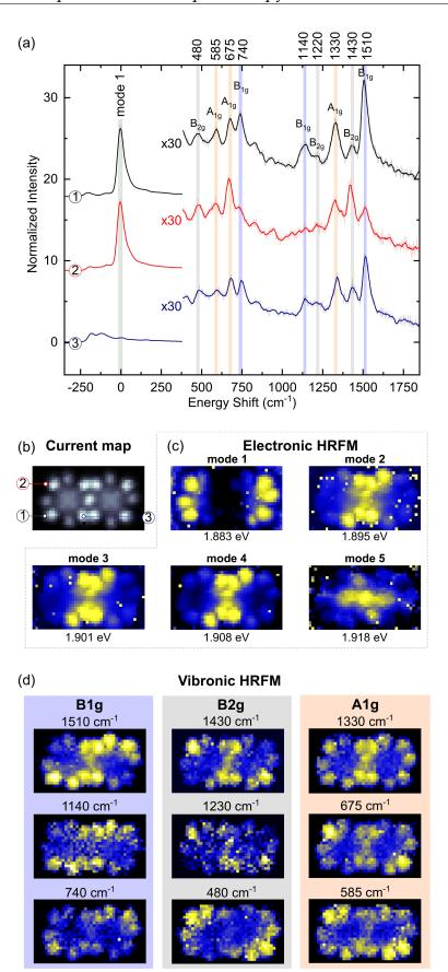
**Figure 4.8: Spatial variation of the vibronic signal.** (a) STM-F spectra acquired at the three positions of a dimer in (b). (b) Current map of the dimer. (c) HRFM maps of the electronic contributions. (c) HRFM maps of the different vibronic peaks indicated in (a).
