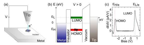
**Figure 1.9: Tunneling through molecular orbitals.** (a) Sketch of the STM junction. The insulating layer is usually several atomic layers thick. (b) Energetic sketch of the double barrier junction. (c) Experimental differential conductance obtained on a single free-base phthalocyanine molecule decoupled from an Ag(111) surface by a thin layer of NaCl.
