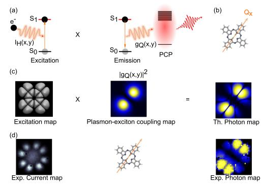
**Figure 3.6:** Modelisation of the  $Q_x$  HRFM map (a) Sketch depicting the fluorescence process. (b) Orientation of the transition moment dipole of the  $Q_x$  transition. (c) Theoretical map obtained as a convolution of the excitation map and the emission map. The emission map is the square absolute value of the plasmon-exciton coupling map. (d) Experimental map.
