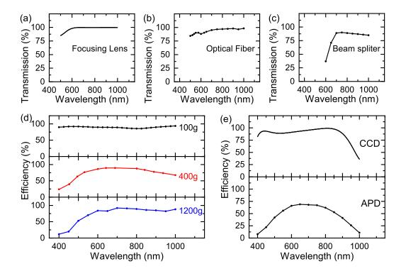
**Figure 1.13:** Transmission and efficiency of the optical components. (a) Focusing lens transmission as a function of the wavelength (Thorlabs AC 254-050-B) (b) Transmission of the optical fiber (SEDI ATI  $7 \times 200$  Vis-IR). (c) Transmission of the beam splitter (Thorlabs cube beam splitter 700-1100 nm) (d) Efficiency of the three different gratings. (e) Efficiency of the CCD camera (top pannel) and the APD (lower pannel).
