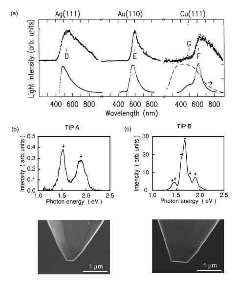
**Figure 2.2: Influence of the tip shape and composition of the STM junction on the STM-LE spectrum.** (a) Spectra obtained with the same tungsten tip above different metallic surfaces. Adapted from [6] (b) and (c) Top panel: STM-LE spectra obtained with two different tips, labelled Tip A and Tip B. Bottom panel: SEM image of the two different tips. Adapted from [75]
