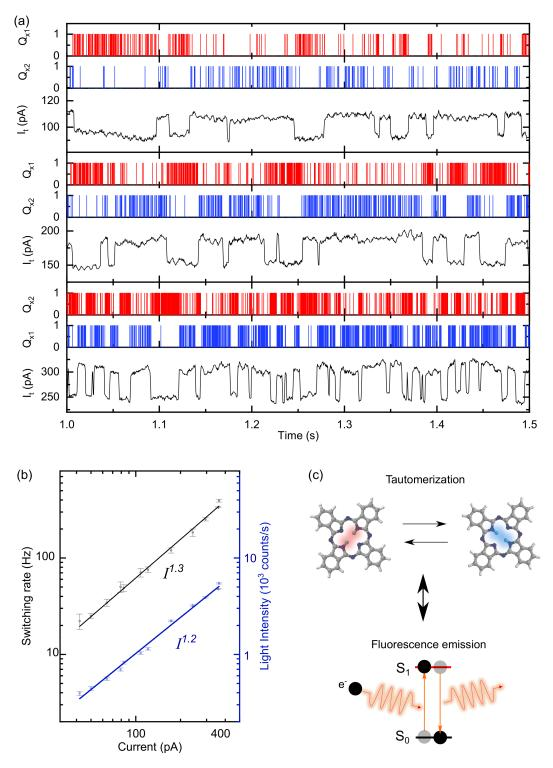
**Figure 3.11:** Evolution of the tautomerization switching rate as a function of the current. (a) Temporal traces of the  $Q_{x1}$  and  $Q_{x2}$  lines, and of the tunneling current (V = -2.5 V). (b) Evolution of the switching rate (dark line) and the light intensity (blue line) as a function of the tunneling current. (c) Sketch illustrating the connection between tautomerization and fluorescence excitation.
