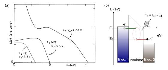
**Figure 2.1: Light emission from a metal-insulator-metal junction.** (a) Spectra obtained under different voltages for different metals. Adapted from [64] (b) Sketch depicting the emission of a photon by an inelastic electron.
