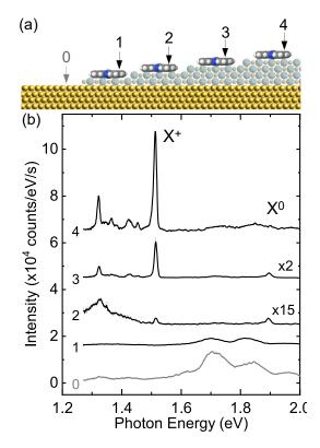
Figure 5.3: Influence of the insulator thickness on the otpical response of the two redox species (a) Sketch depicting the experiment where STM-F spectra are recorded on a single ZnPc molecule adsorbed on 0, 1, 2, 3, and 4 atomic layers of NaCl. (b) STM-F spectra (V = -2.5 V; I = 300 pA) recorded on a single molecule adsorbed on 1ML (t = 300 s), 2ML (t = 180 s), 3ML (t = 120 s), 4ML (t = 10 s). The spectrum labeled 0 is recorded on the bare Au(111) surface.
