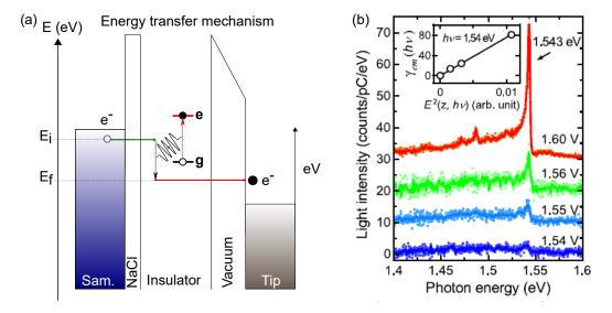
**Figure 2.19:** Energy transfer mechanism (a) Energy sketch of the mechanism. The inelastic tunneling transition is resonant with the molecular exciton with the condition  $E_i - E_f = hv$ . Therefore the energy threshold is given by  $e|V| \ge hv$ . (b) Voltage dependency of the STM-LE intensity of a suspended porphyrin molecule. Adapted from [20]
