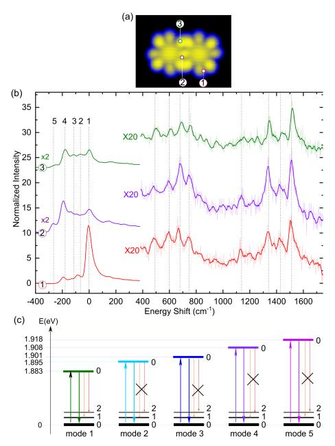
**Figure 4.7: Impact of the excitonic coupled modes on the vibronic signal** (a) STM image of a dimer. (b) STM-F spectra recorded at the three different positions marked in (a). (c) Sketch of the different transitions for the five different excitonic modes.
