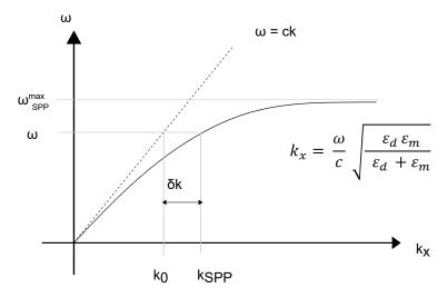
**Figure 2.4:** Dispersion relation of SPP (dark line). The dashed line corresponds to the dispersion relation for a free propagating electromagnetic field.  $\delta k$  is the impulsion mismatch between SPP and the photon.
