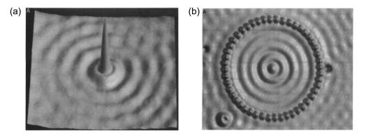
**Figure 1.4:** Electronic standing waves probed by STM. (a) STM image of a single Fe atom deposited on a Cu(111) surface. The concentric rings are standing waves due to the scattering of surface state electrons. (b) STM image of a ring of 48 Fe atoms deposited on a Cu(111) surface. The standing wave pattern is due to the closure of the ring that confines electrons inside t,he ring.
