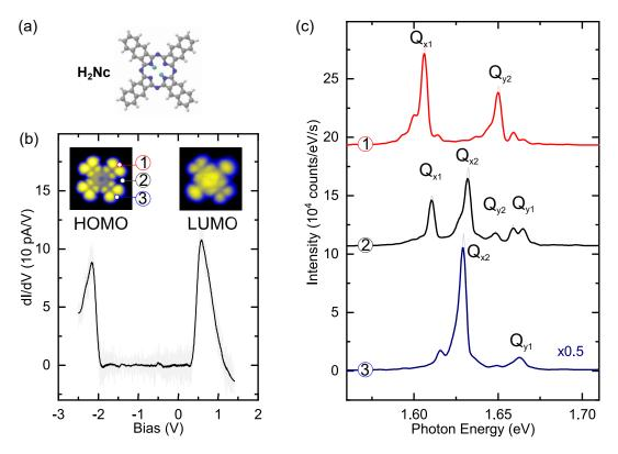
**Figure 3.14:** Properties of the naphthalocyanine molecule (H<sub>2</sub>Nc). (a) Sketch of the H<sub>2</sub>Nc molecule. (b) Differential conductance spectrum of a single H<sub>2</sub>Nc molecule adsorbed on 3 layers of NaCl on Ag(111). Inset: STM images ( $3.5 \times 3.5$  nm<sup>2</sup>) of the HOMO (V = -1.9 V; I = 10 pA) and LUMO (V = +0.7 V; I = 10 pA). (c) STM-F spectra (V = -2.2 V; I = 50 pA; acquisition time: t = 180 s) recorded at the different tip positions marked in (b).
