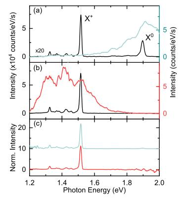
Figure 5.4: Influence of the NCP on the optical response of the two redox species (a) STM-F spectra (V = -2.5 V; I = 300 pA) recorded on the single molecule (dark line; t = 300 s), and on the NaCl (blue line; t = 60 s) to provide the NCP response. (b) STM spectra of the ZnPc molecule (dark line) and of the NCP (red line). (c) ZnPc spectra normalized by the corresponding NCP response.
