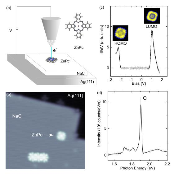
**Figure 4.1: Description of the system** (a) Sketch of the experiment. (b) Large scale image of ZnPc molecules on three-layers NaCl island on Ag(111). (c) Differential conductance spectrum of the ZnPc molecule. Inset: STM image ( $2.7 \times 2.7 \text{ nm}^2$ ) of the LUMO (V = +1 V; I = 10 pA) and HOMO (V = -2.2 V; I = 10 pA) orbitals. (d) STM-F spectrum of the ZnPc molecule (V = -2.5 V; I = 300 pA; acquisition time t = 180 s).
