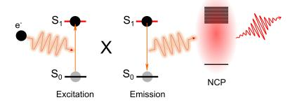
Figure 3.4: Fluorescence process in a STM junction
