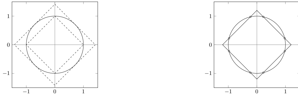
(a) The \ell_2 -sphere of radius 1 (continuous line) and the \ell_1 -spheres of radius s_l = 1 and s_l = \sqrt{2} (dashed lines).
