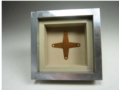
Figure 3.21: Star-shape metallization for coaxial probes connection
