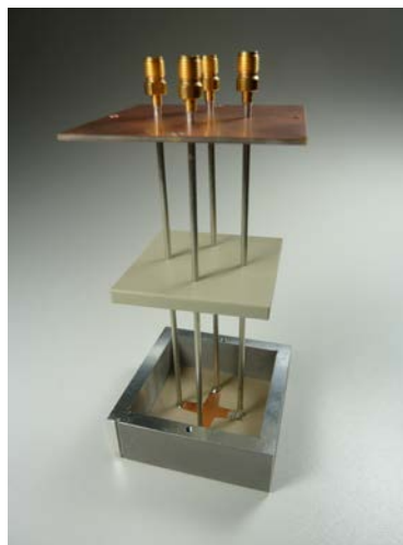
Figure 3.22: Assembly of the different parts of the antenna
