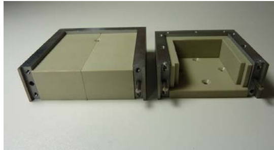
Figure 2.22: Two versions of the polypropylene blocks inside the cavity
