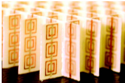
Figure 1.30: Wire-SRR metamaterial to verify negative refraction[17]
