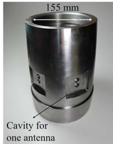
Figure 19: Carrier model to embedded antennas: 155 mm projectile section
