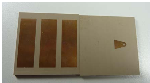
Figure 2.23: Metallization design of microstrip layers
