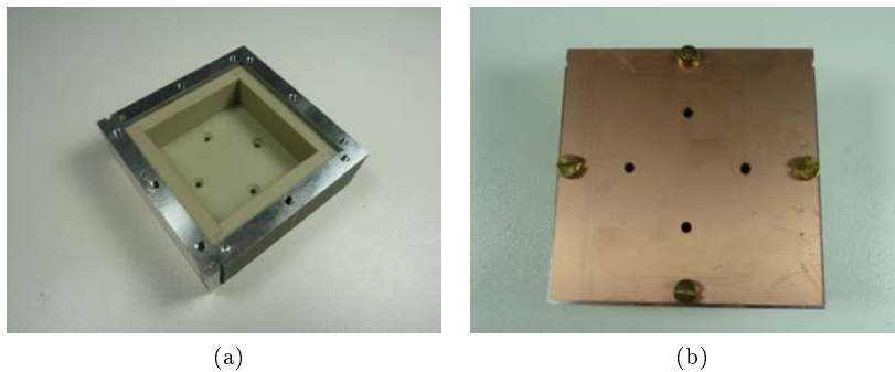
Figure 3.20: (a) Cavity with polypropylene blocks. (b) Bottom cooper part of the cavity
