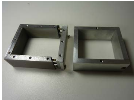
Figure 2.21: Two versions of the metal cavity used for the prototypes
