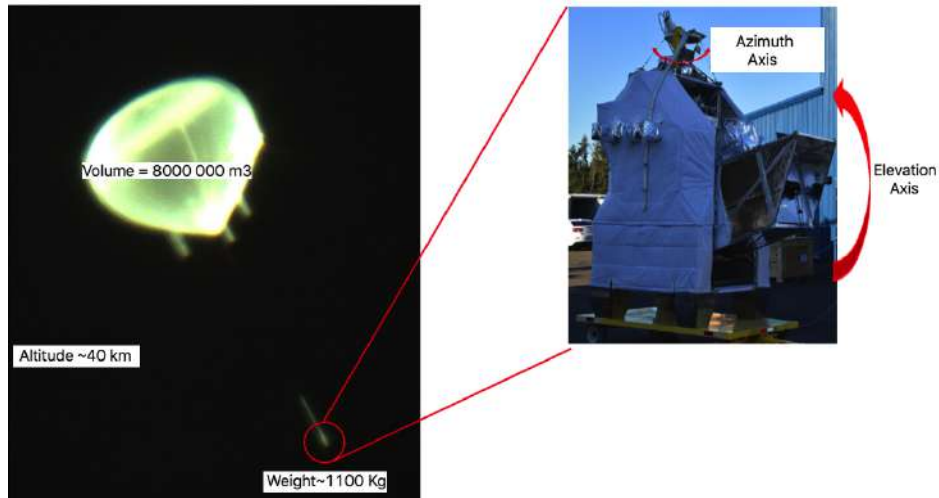
Figure 2.1: Views of the PILOT experience. Left: the stratospheric balloon in flight above Timmins in September 2015. Right: the gondola on the way to the tarmac.
