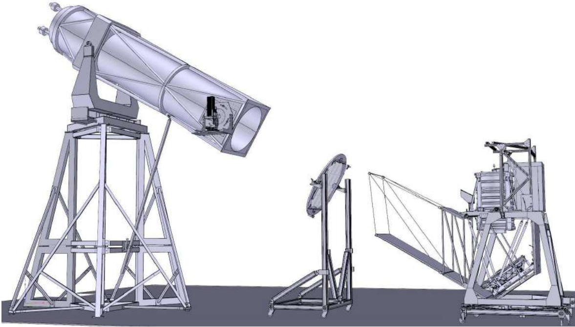
Fig. 15 Optical bench used to characterize polarization properties of the instrument. From right to left, the PILOT pointed load, the large format Archeops polarizer and the IRAP \phi = 1 m collimator.
