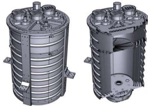
Fig. 6 Schematic view of the cryostat. The right panel shows the inner structure of the helium tank (upper part), the cold optics compartment (lower part) and the various thermal screens.
