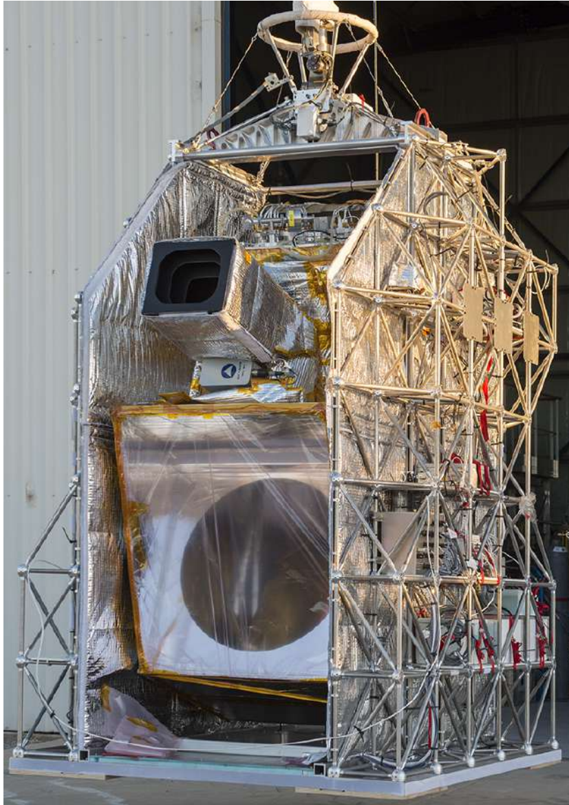
Figure 4.1: Picture of PILOT during the health tests of the stellar sensor in Alice Springs, in April 2017. The black part over the baffle opening of the PILOT mirror is the baffle of the ESTADIUS stellar sensor
